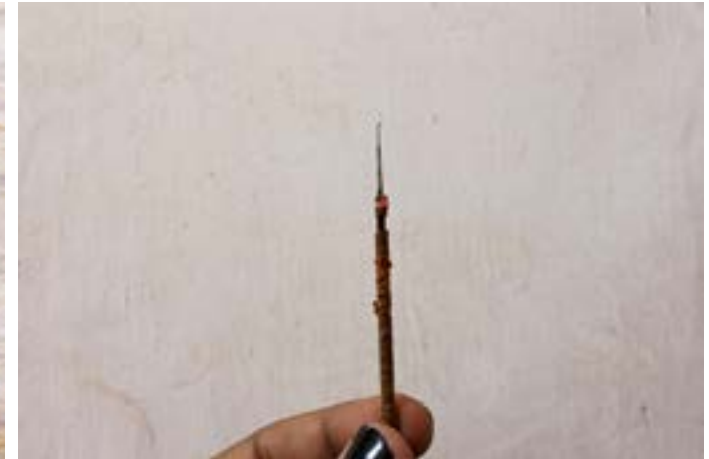
Aari (needle), shaped like a hook at the tip used to embroider.
