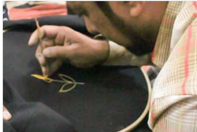
The silk thread is held with a finger and carried to the upper side to secure the previous stitch.
