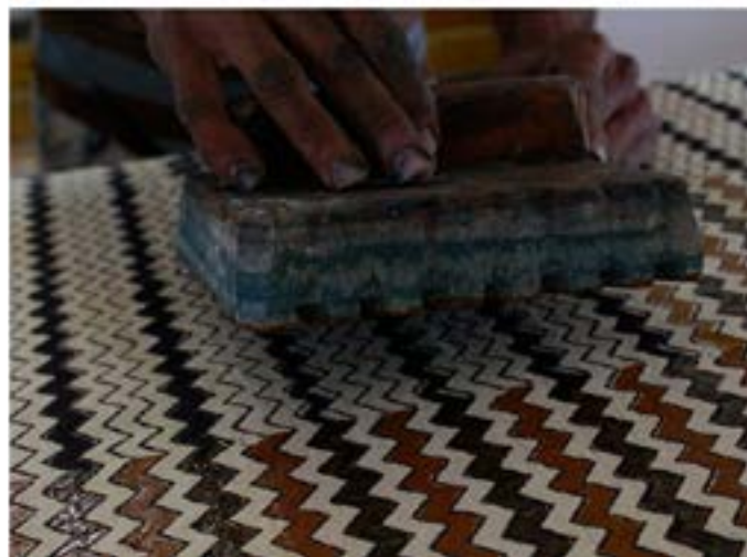
The outlines are printed first and they are filled with another set of printing.
