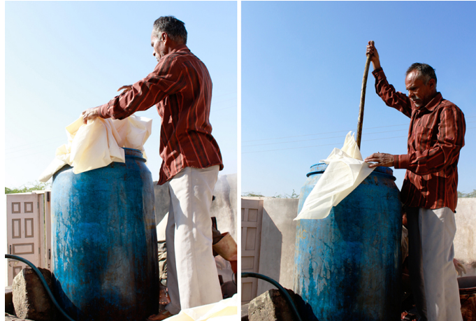
The cloth is dipped in the color solution.
