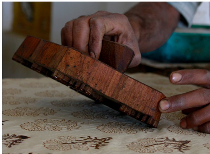
Artisan printing on fabric using designer wooden blocks.
