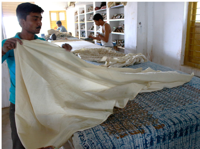
Fabric is evenly spread on a table before printing.
