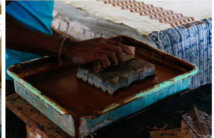
Wooden blocks are dipped in the printing color for printing on the fabric.
