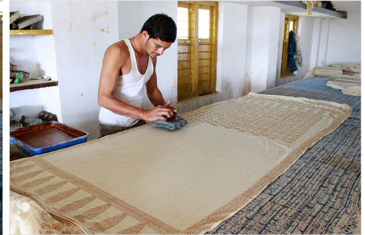
Artisan carefully placing the wooden block to print on the cloth.
