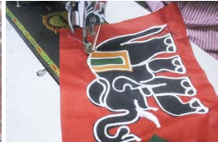
Different sized motif pieces are stitched together along with the lining fabric.
