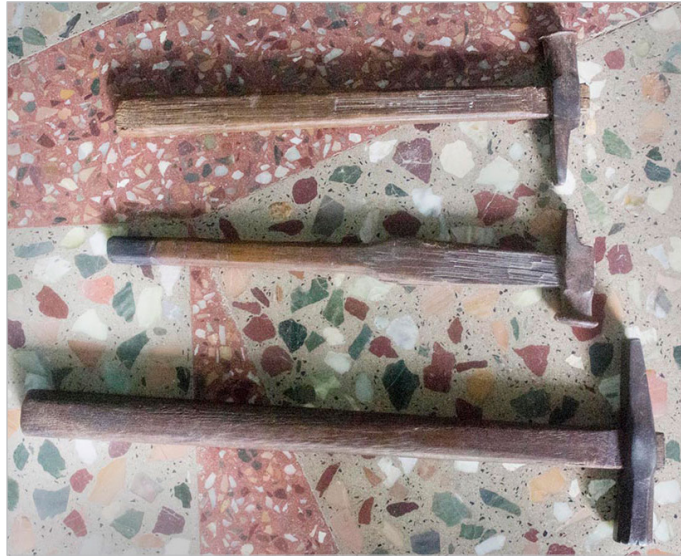
Hammer used for fixing the relief sheets.
