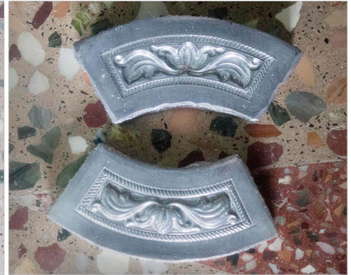
Mould is used for creating impressions on the metal sheets.
