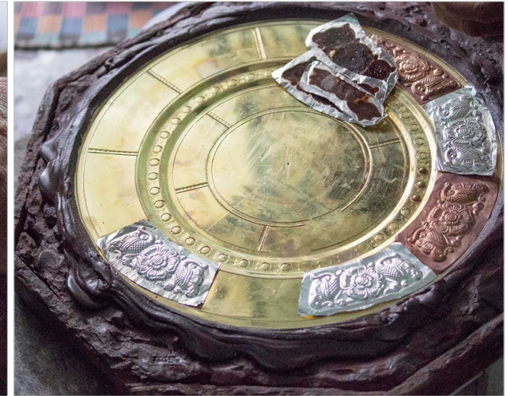
Initially the outer most circle is filled with the metal reliefs as per the design.
