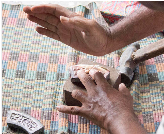
It is again tapped by hand to gain the precise impression.
