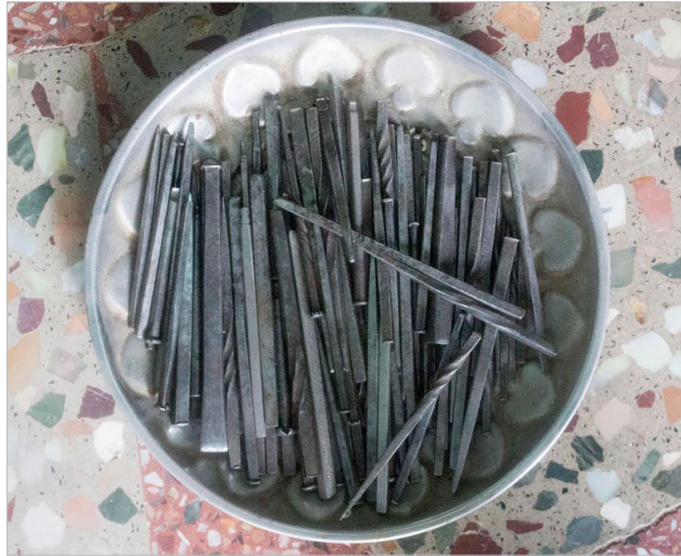
Chisels used for engraving the metal sheets.
