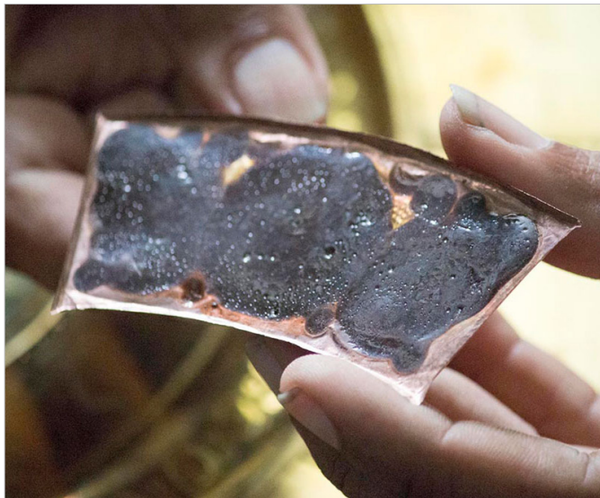
Mixture of brick powder, gingili oil and frankincense is filled in hollow depressions at the back of metal reliefs.
