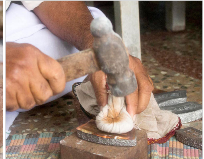
Keeping cloth as the support, impression is gained by tapping on the copper sheet-using hammer.
