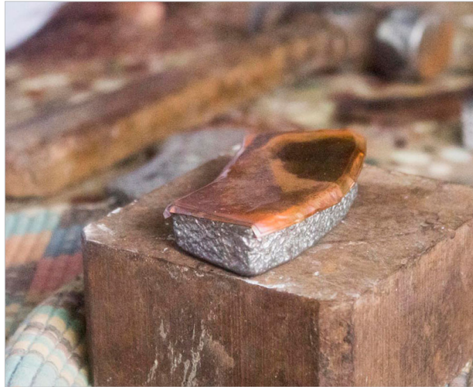
Copper sheet is placed on the mould.
