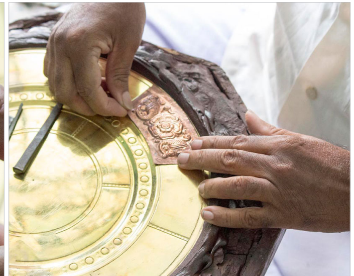
These metals reliefs are placed on the base metal sheet of brass.
