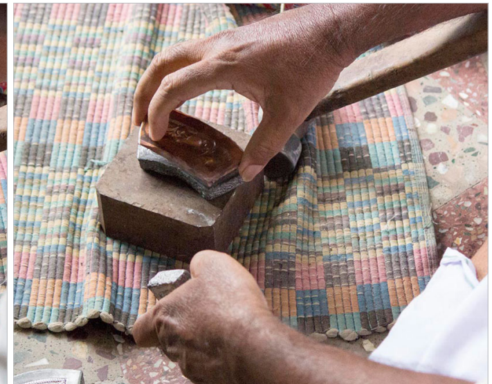
The copper sheet is removed from the mould.
