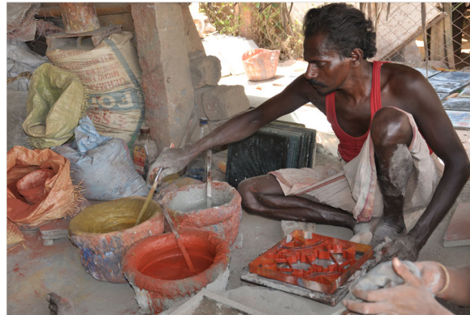
Wooden frame is kept on the glass and wire frame is placed to start the tile making.
