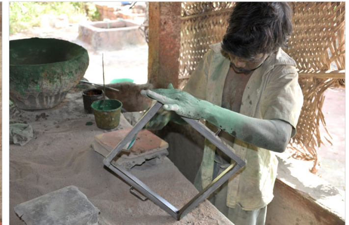
Glass frames are cleaned after every use.
