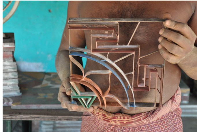
The iron frame through which the colored paste are poured to make the designs.
