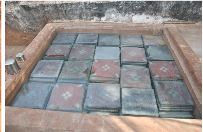
Tiles are dipped in water once these are made. Artisans build water tank in the vicinity for this purpose.
