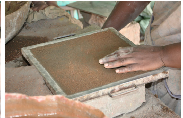
The mortar is checked for leveling with hands.
