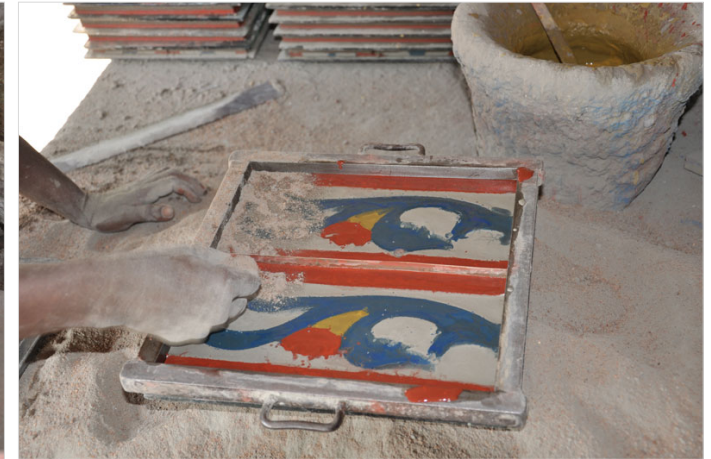
Mixture of dry cement and sand is sprinkled on the surface in order to set the design.
