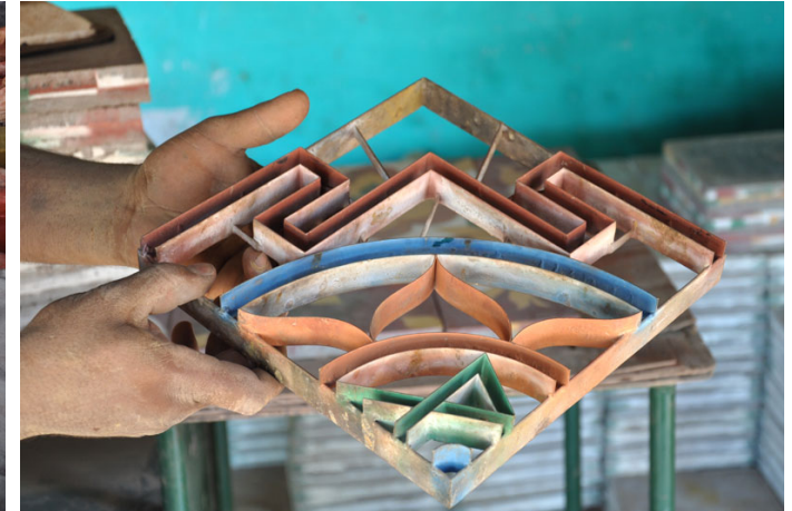
Different designs of frames are used to make designs.
