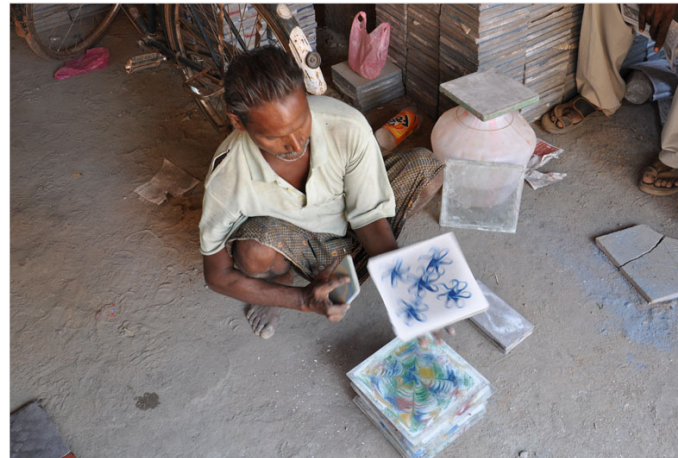
After that the tiles are taken out and the edges are smoothed with the help of stone.
