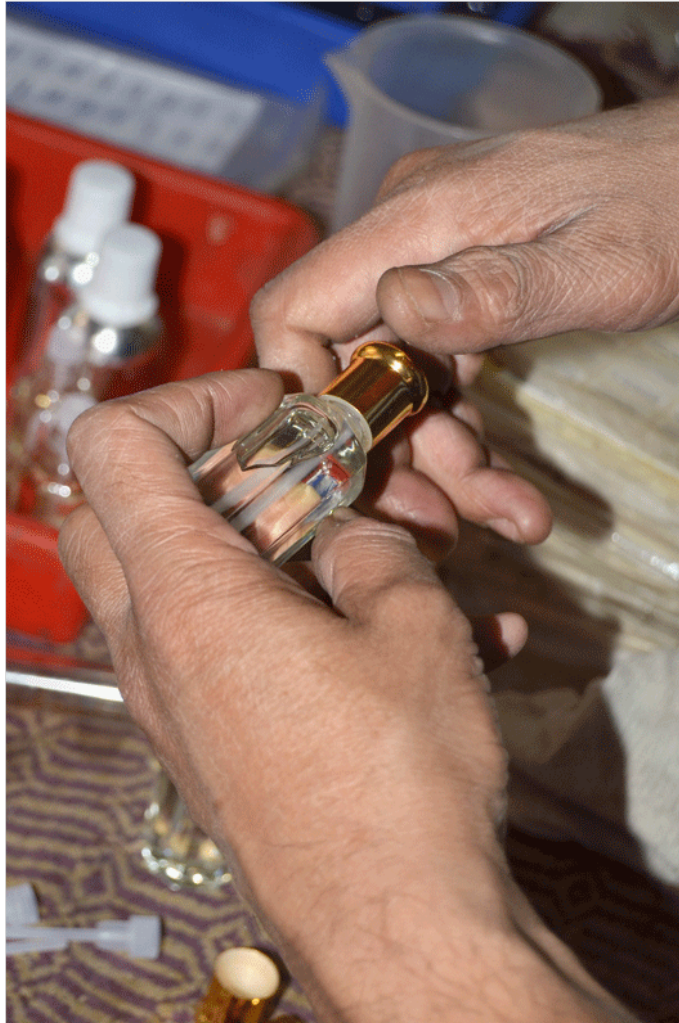
Metal caps being wound onto the glass bottles
