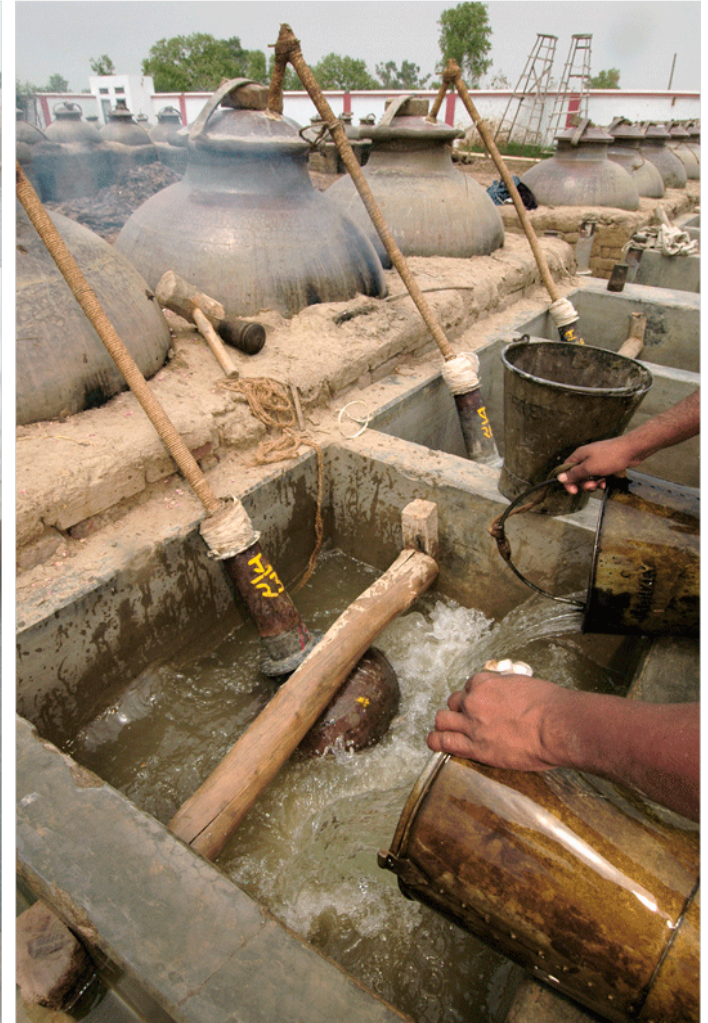
The vessel at the other end of the tube in which the 'attar' is collected
