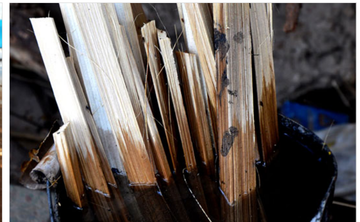
Bamboo is split into small strips and soaked in water.
