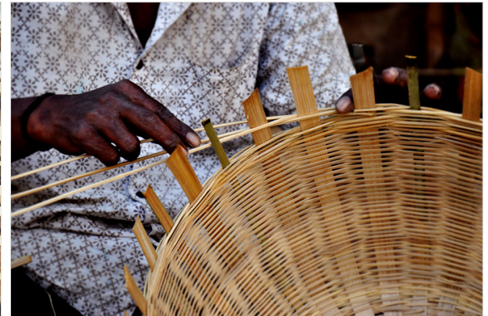
The inserted splits of bamboo are tightened by pulling.
