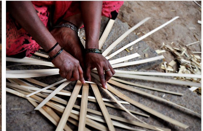
Small thin strip of bamboo is inserted to base to begin weaving.
