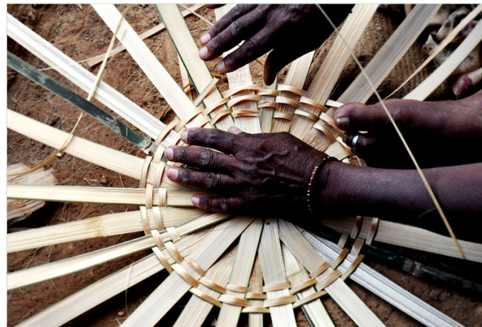
Aligning and tightening the base after every round of weave.
