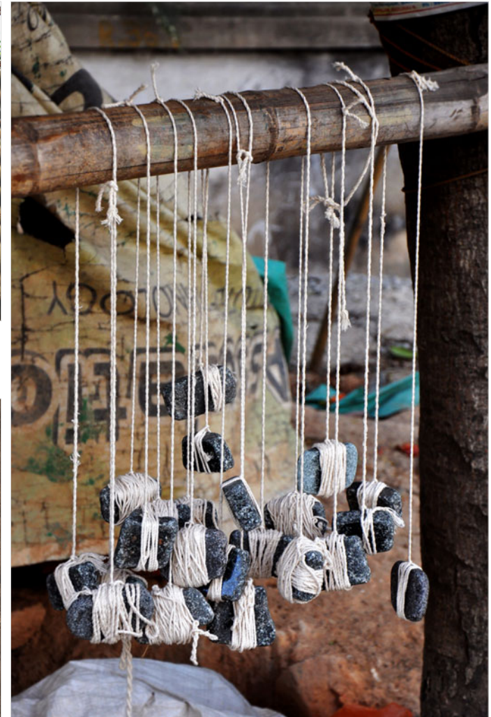
Suspended stone weights are used mat weaving process.
