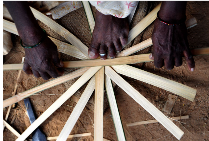
The strips are arranged to make base of the basket.
