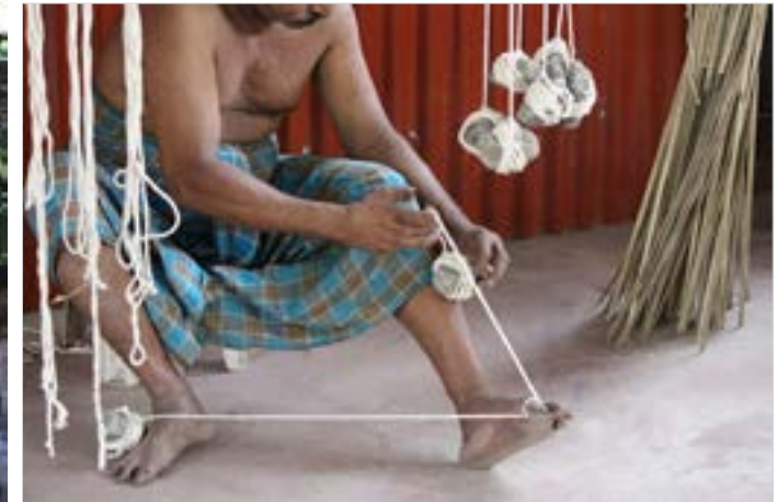
Artisan with the help of his feet takes the required length of thread.
