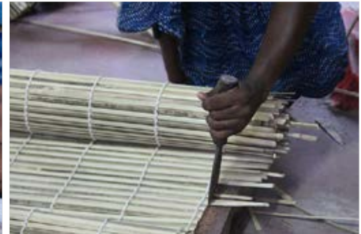
Unwanted length of strips are trimmed using chisels tools.
