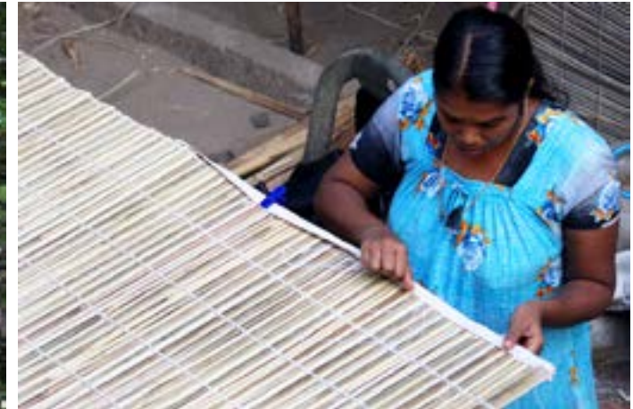
The edges of the bamboo curtains are getting stitched using cloth.
