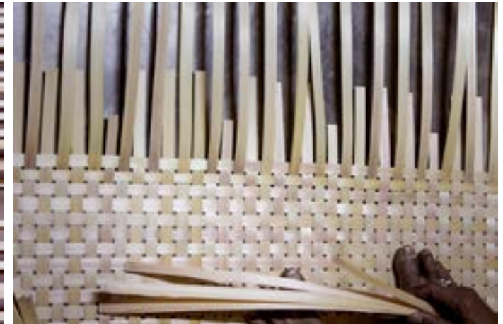
View of the half-finished mat.
