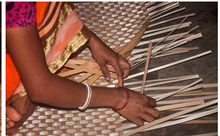
The artisan is weaving the bamboo strips for making the mat.
