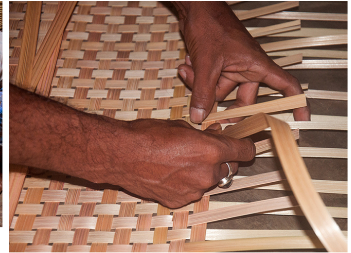
Artisan is arranging the thin bamboo strips for the mat weaving process.
