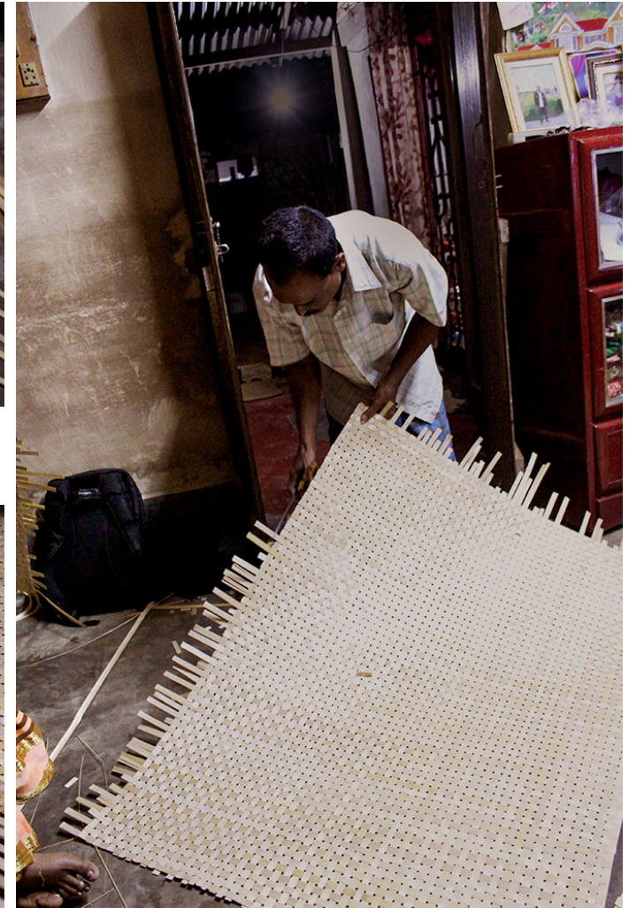
Artisan is using the scissor to cut the extra part of the bamboo mat strip.
