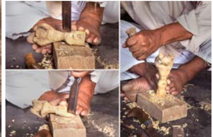
The craftsman is using the flat chisel on the bamboo surface for giving a proper shape.
