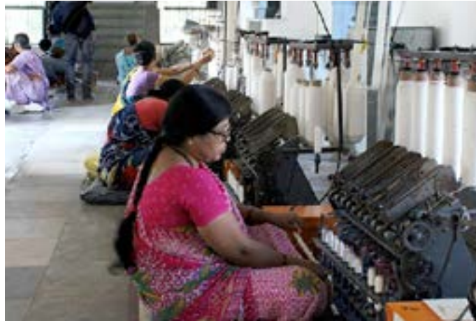
Female employees working on the spinning of threads, where thicker versions are made out of thin threads.
