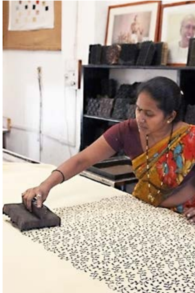
Block being pressed on the cloth.
