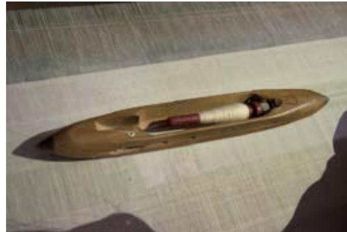
A shuttle is used in the weaving machine, which runs horizontally with the thread.
