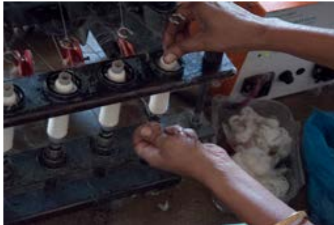
A view of the small rollers that receive the thread.
