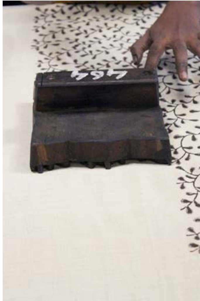
The block is hammered twice or thrice for a firm good impression.
