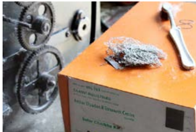
Regulator to operate the spinning machine.
