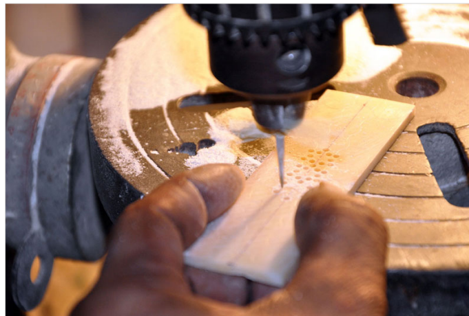
7. The holes are drilled as per the marked design.
