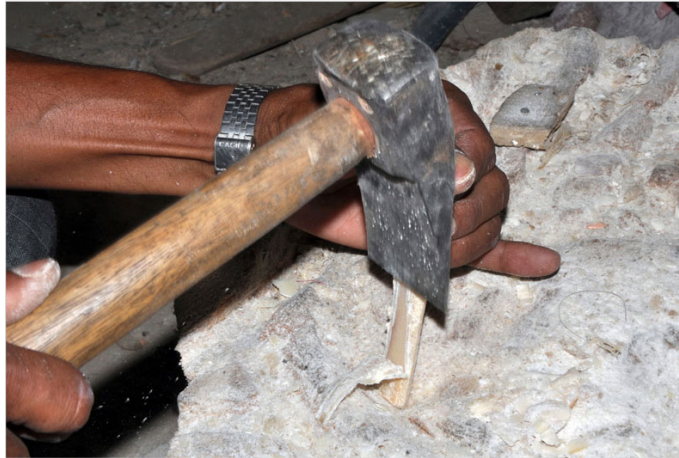
1. The raw bone is cut into small rectangular shape.
