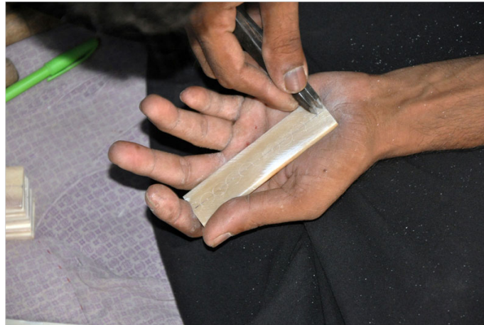
5. Initial designs are marked on the surface of the bone
