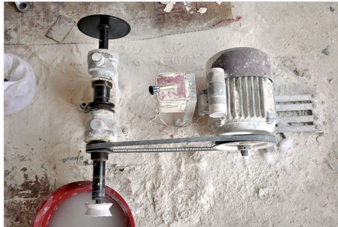
11. Over-view of buffing machine.
