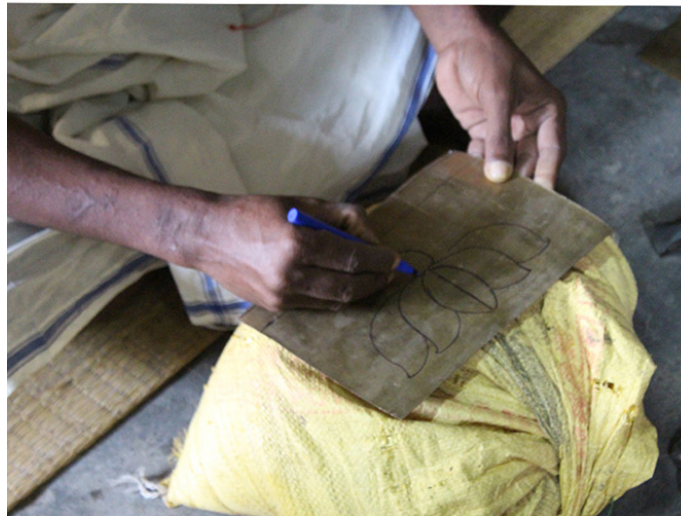
The rough sketch is drawn on the brass sheet using marker.
