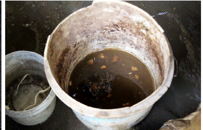
Tamarind used to wash the brass sheet.
