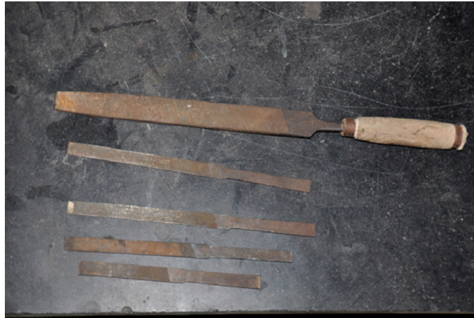
A hand file tool used to shape materials.
