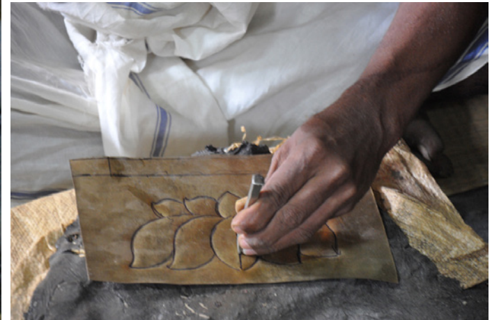
Detail work is embossed using small chisels.
