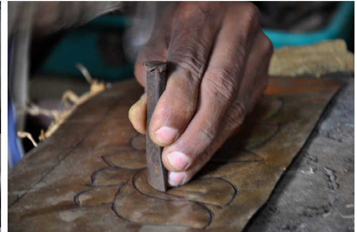
Artisan carves the design with chisel following the rough sketch.
