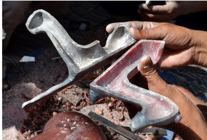
Two halves of the 'master-copy' for casting.
