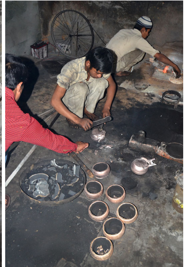
Gating' being hammered off from the cast.
