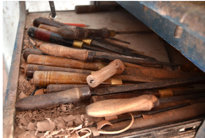
Tools for carving the wax and wooden moulds.
