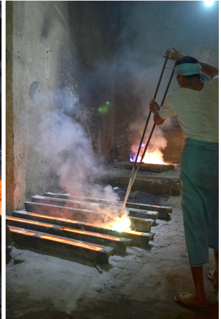
Molten metal being poured in the mould.
