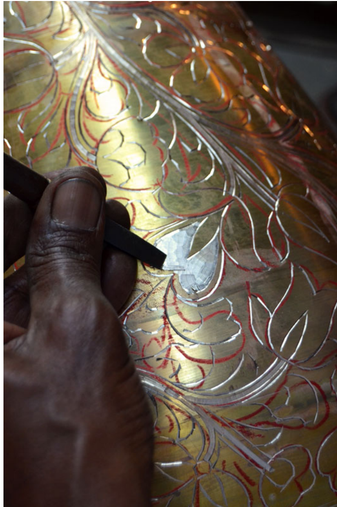
Pencil sketched design being engraved with varying depths for enamel.
