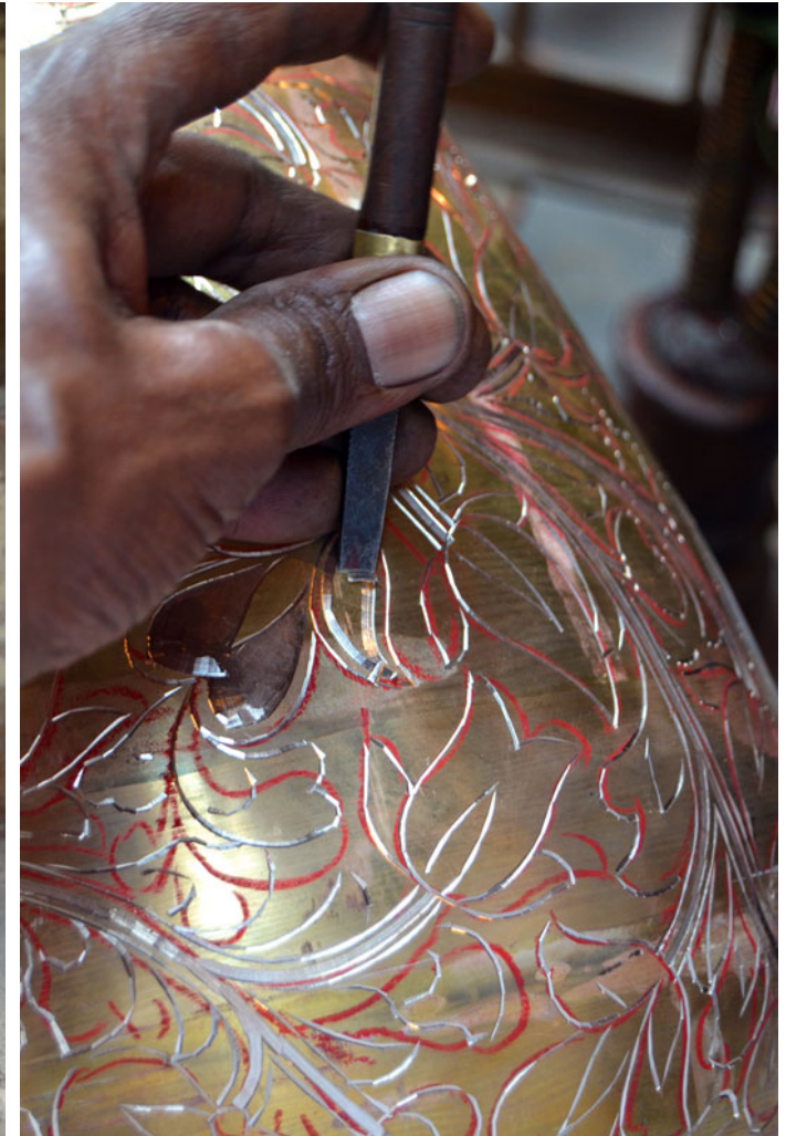
Pencil sketched design being engraved with varying depths for enamel.
