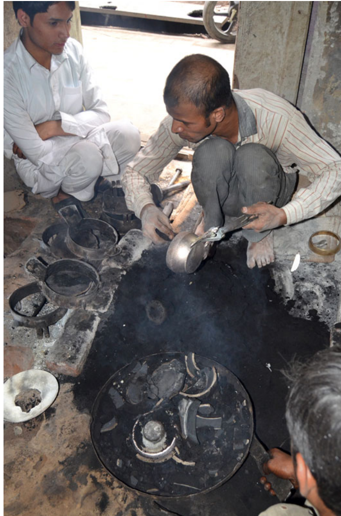
After cooling off, mould box is opened to remove the cast.
