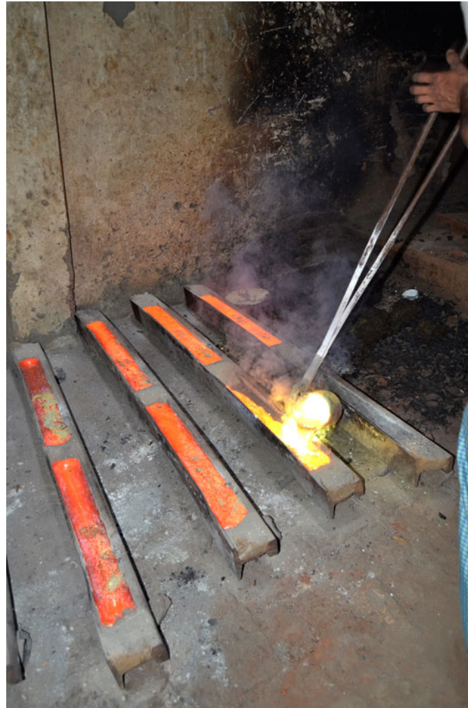
Molten metal being poured in the mould.
