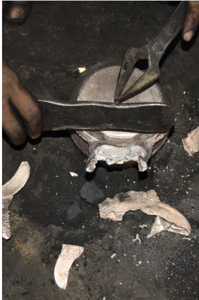
Gating' being hammered off from the cast.
