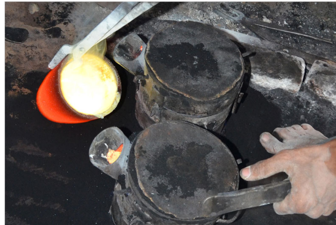
Molten brass being poured in the cavity.
