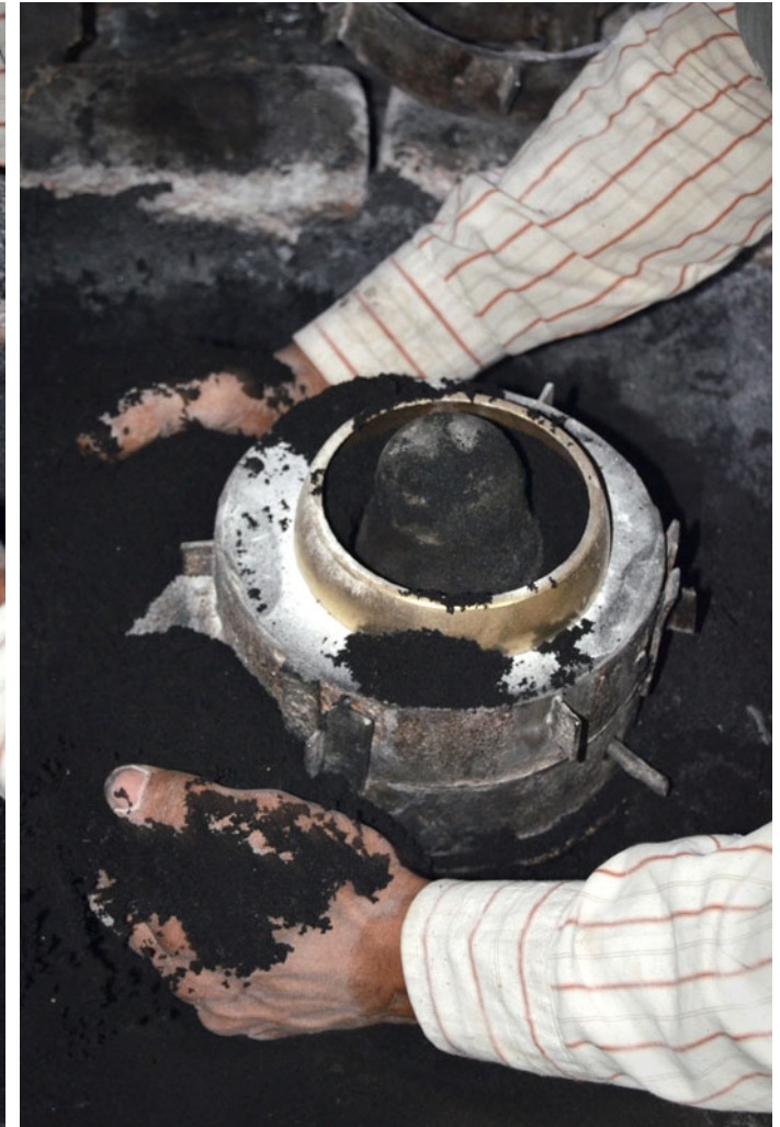
A karigar preparing the mould box with the 'master-copy' and sand.
