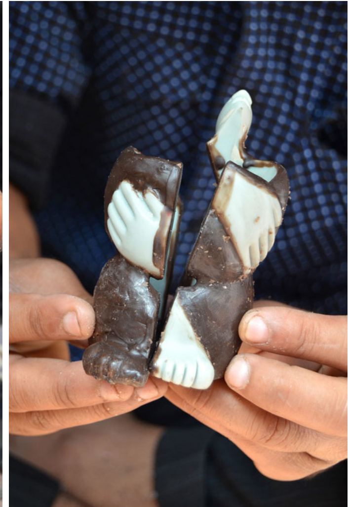
Mould for pen stand being made in wax.
