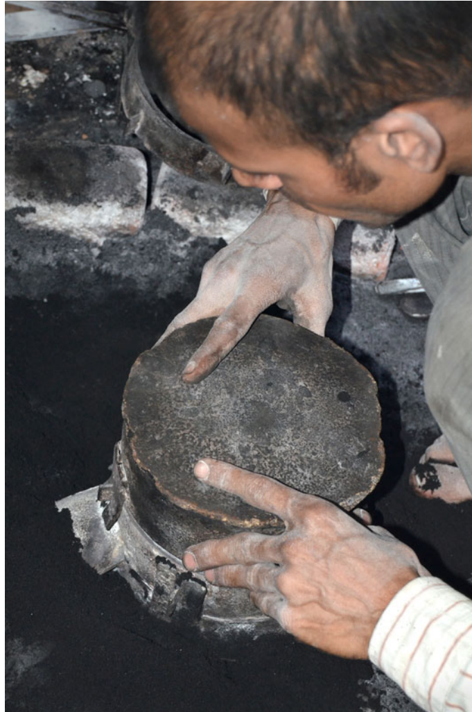
'Master-copy' is removed from the mould box and a cavity is created
