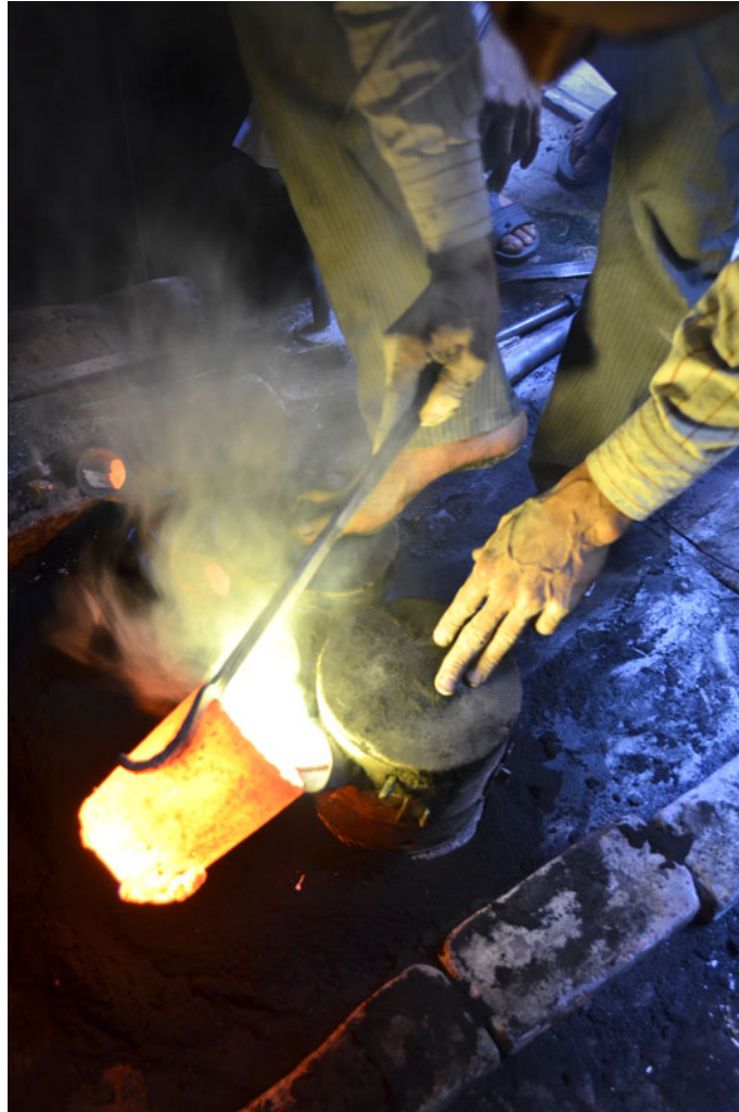
Molten brass being poured in the cavity
