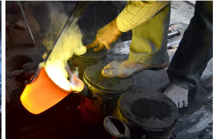
Molten brass being poured in the cavity.
