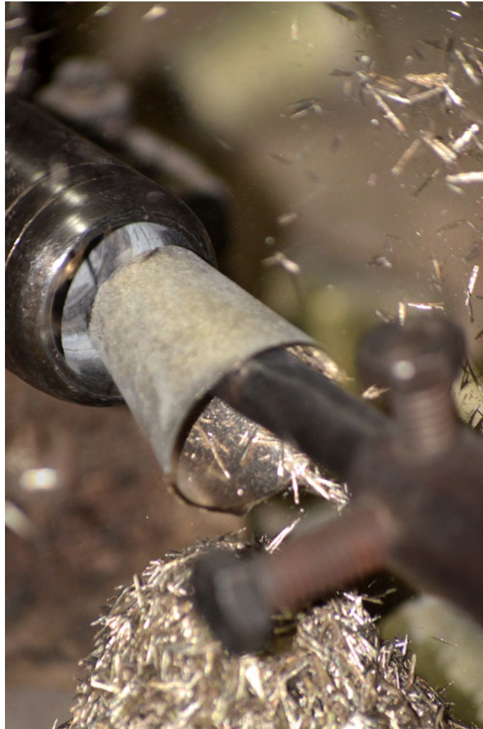
The filing tool attached to the lathe machine to scrap the tumbler.
