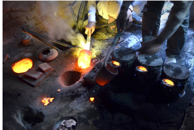
Molten brass being poured in the cavity.
