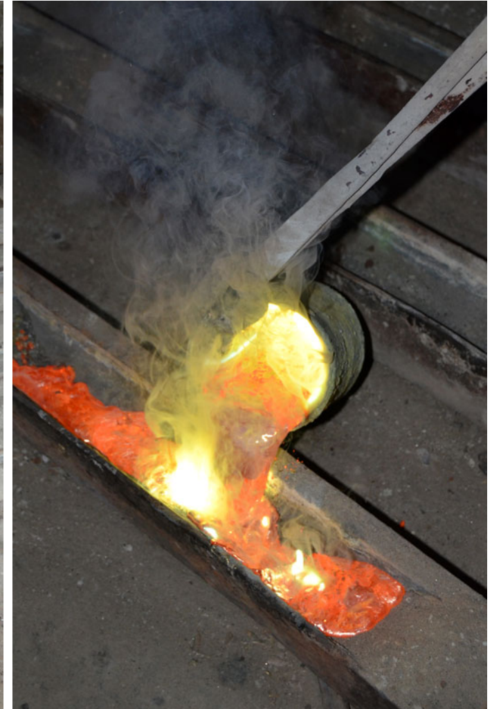
Molten metal being poured in the mould.
