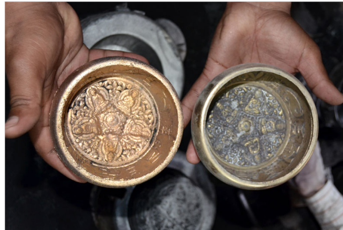
Brass mould ('master-copy') and cast.
