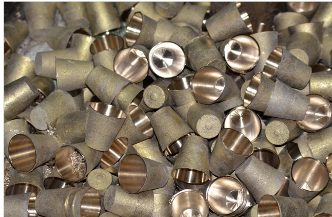
A mix of scraped and not-scraped tumblers.
