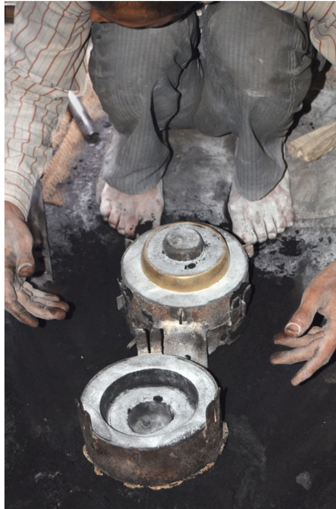
A karigar preparing the mould box with the 'master-copy' and sand.
