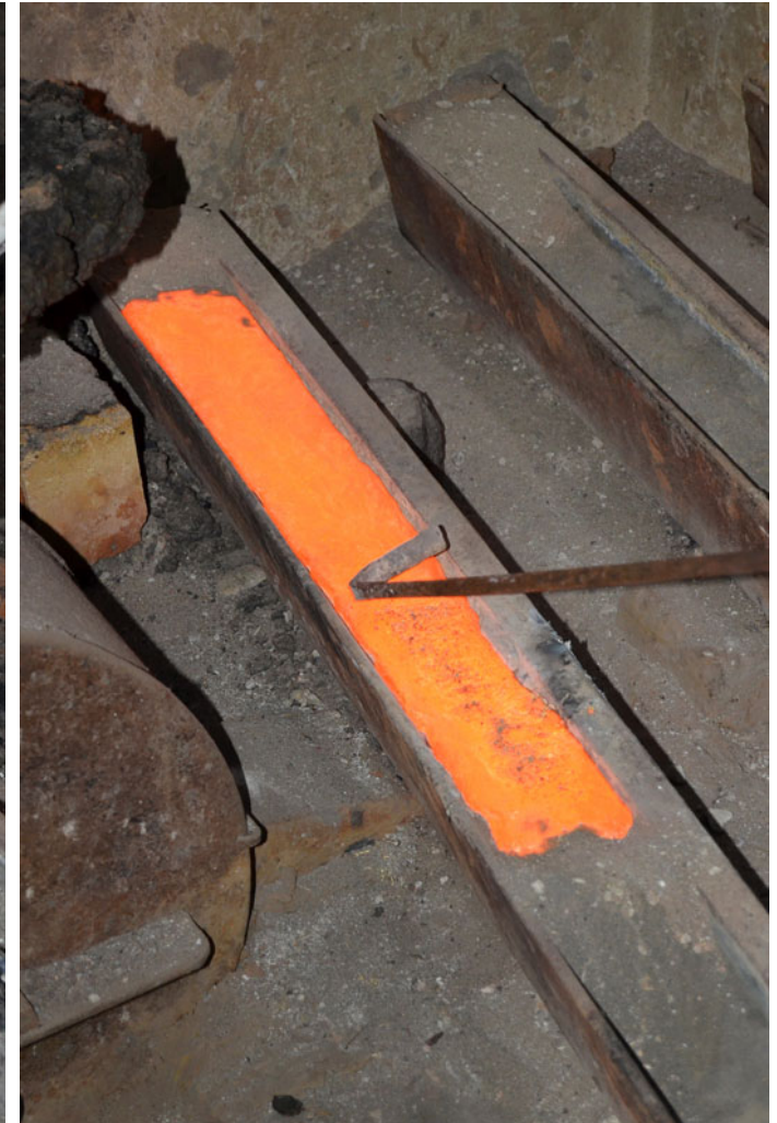
Molten metal being poured in the mould.
