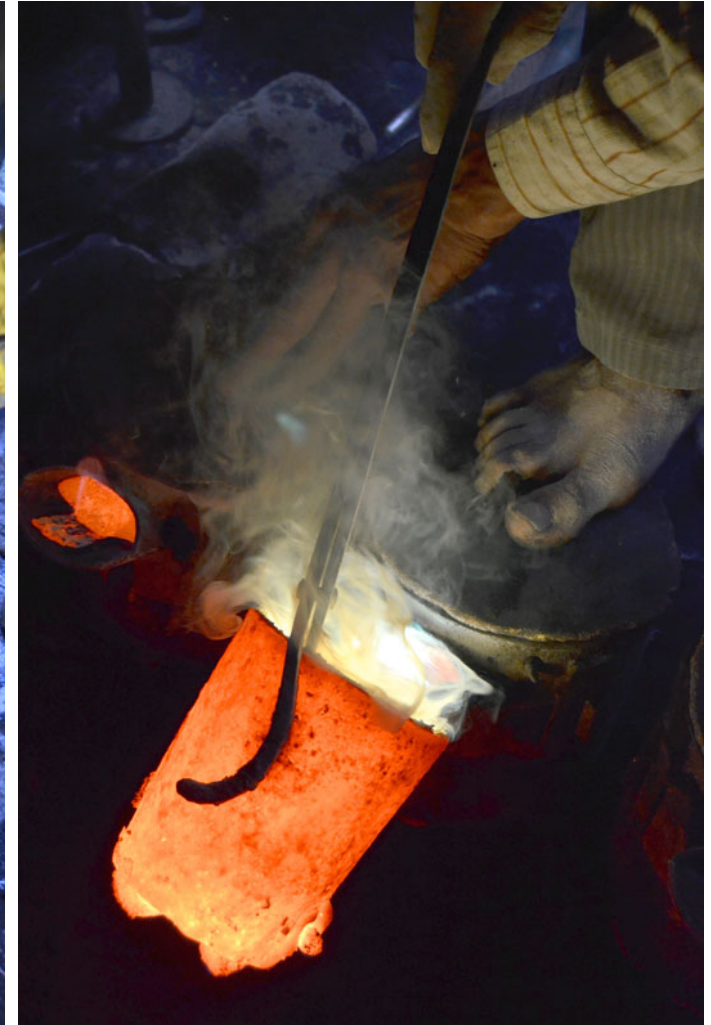
Molten brass being poured in the cavity
