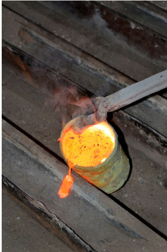
Molten metal being poured in the mould.
