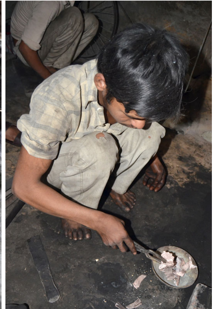
Hammered pieces of brass to be re-used in the next casting.
