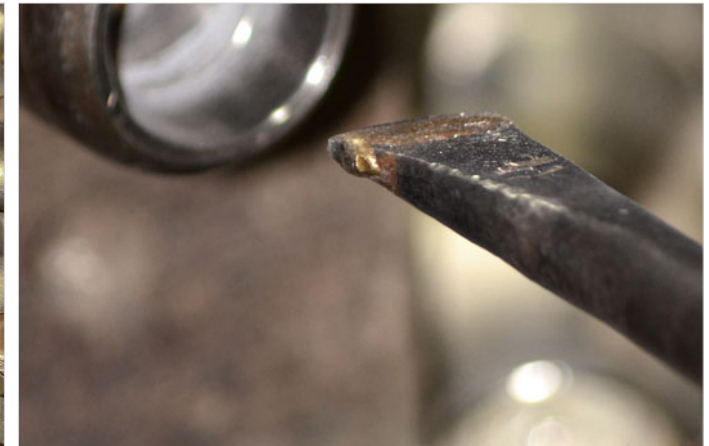
The filing tool attached to the lathe machine to scrap the tumbler
