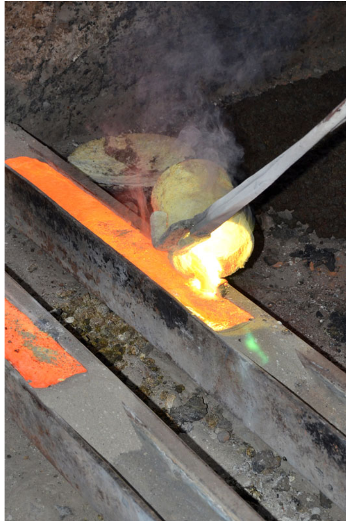
Molten metal being poured in the mould.
