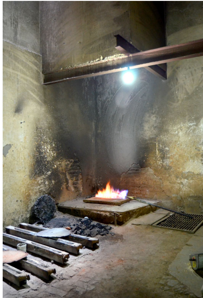
The furnace where brass is prepared by melting several metals
