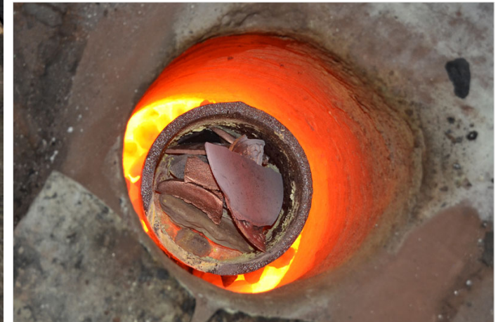
Pieces of brass being heated in the furnace for casting.
