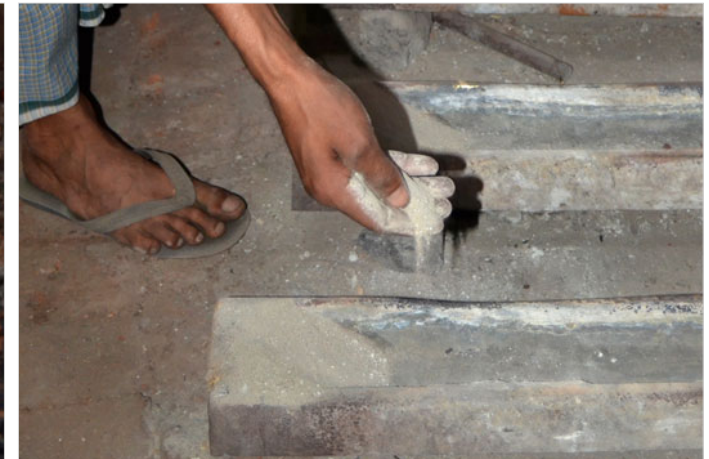
Putting sand in the mould to prevent molten metal overflow.
