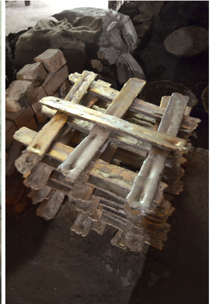
Brass metal strips after cooling.
