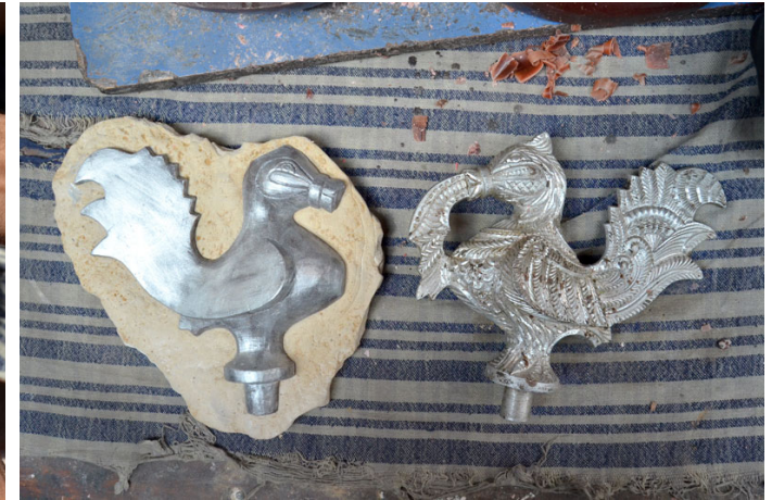
The 'master-copy' (mould) and its corresponding cast.
