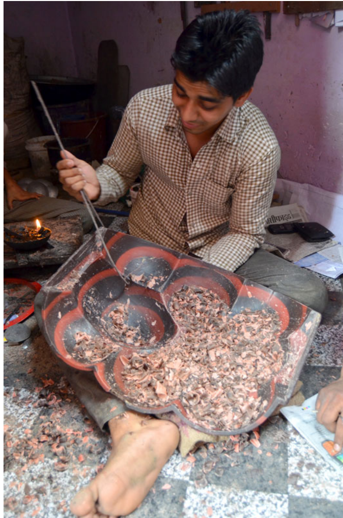
Mould being made in wax.
