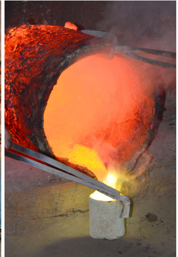
Karigars pouring out the remaining molten metal.
