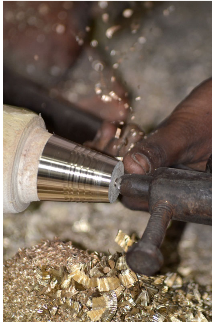
The wooden block attached to the headstock of the lathe machine to scrap the tumbler.
