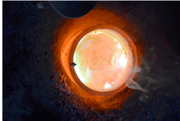
Pieces of brass being heated in the furnace for casting.
