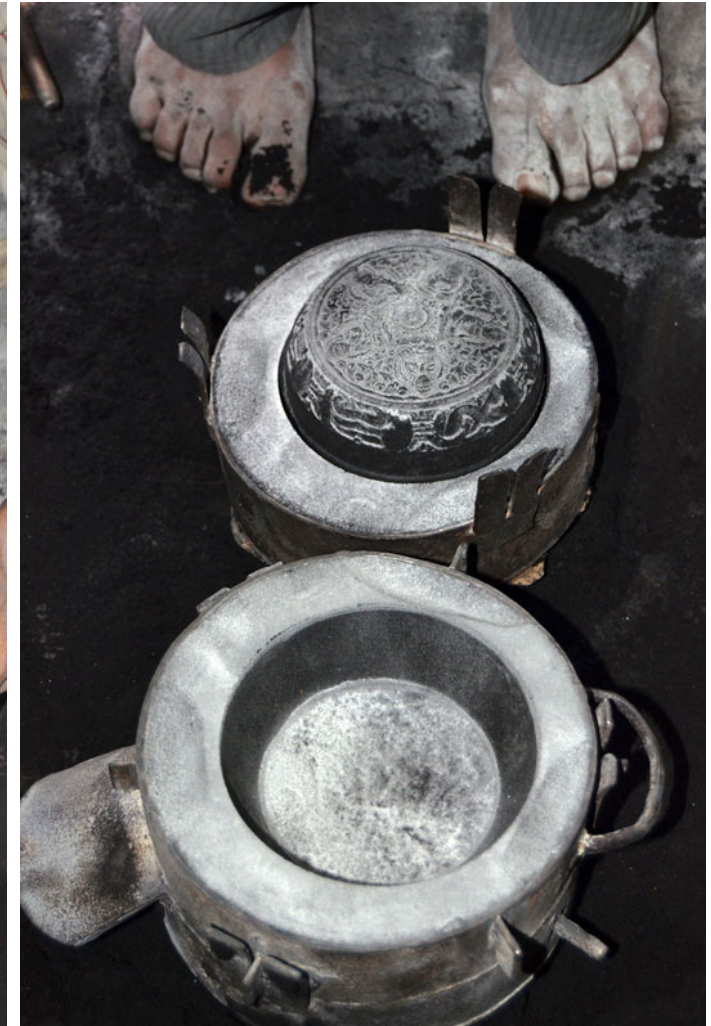
Master-copy' is removed from the mould box and a cavity is created.
