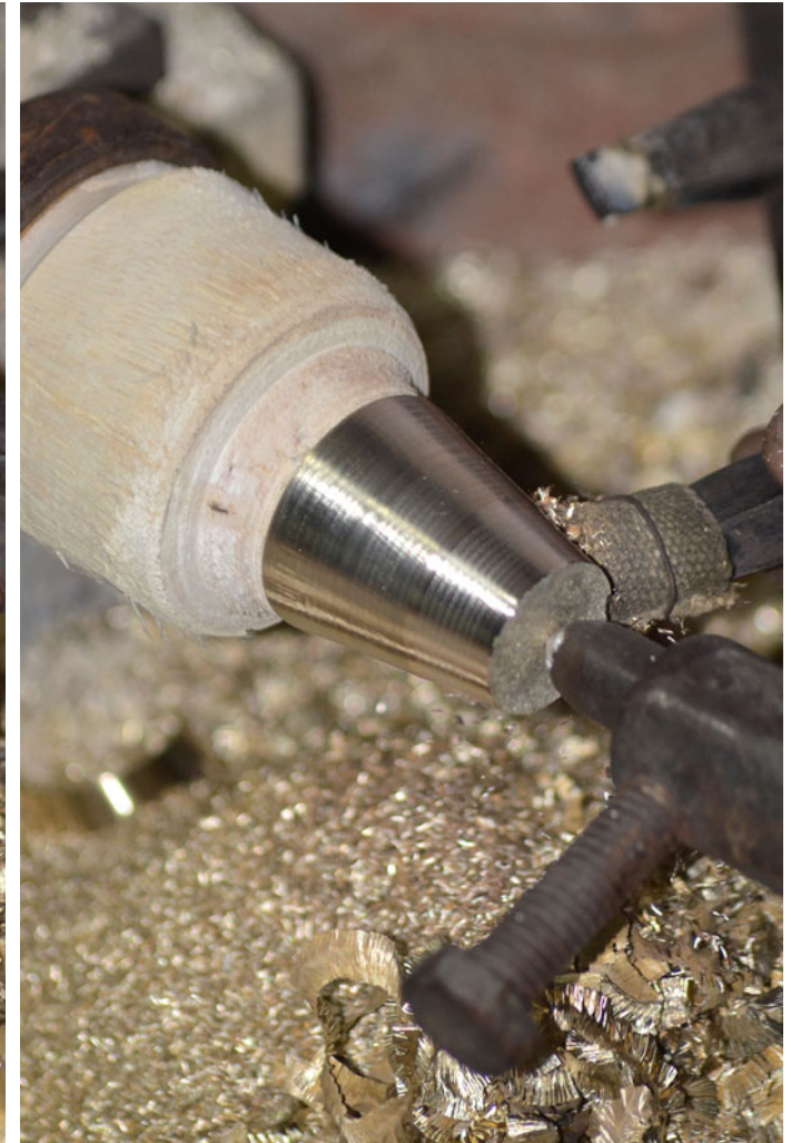
The wooden block attached to the headstock of the lathe machine to scrap the tumbler.
