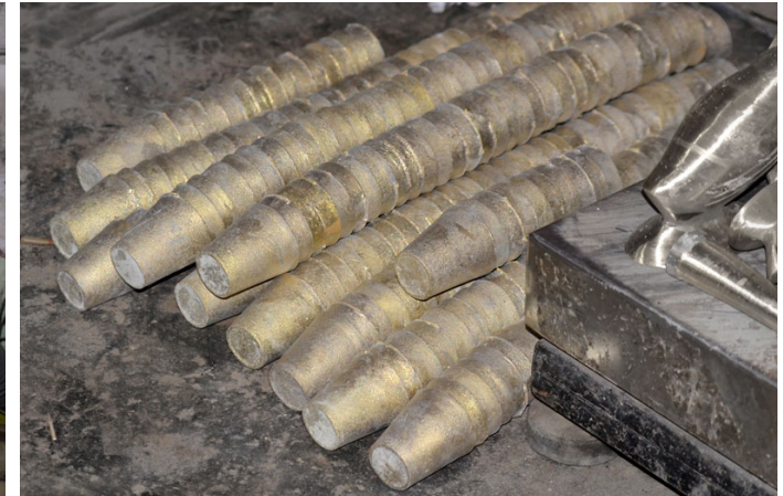
Small tumblers to be scraped on the lathe.
