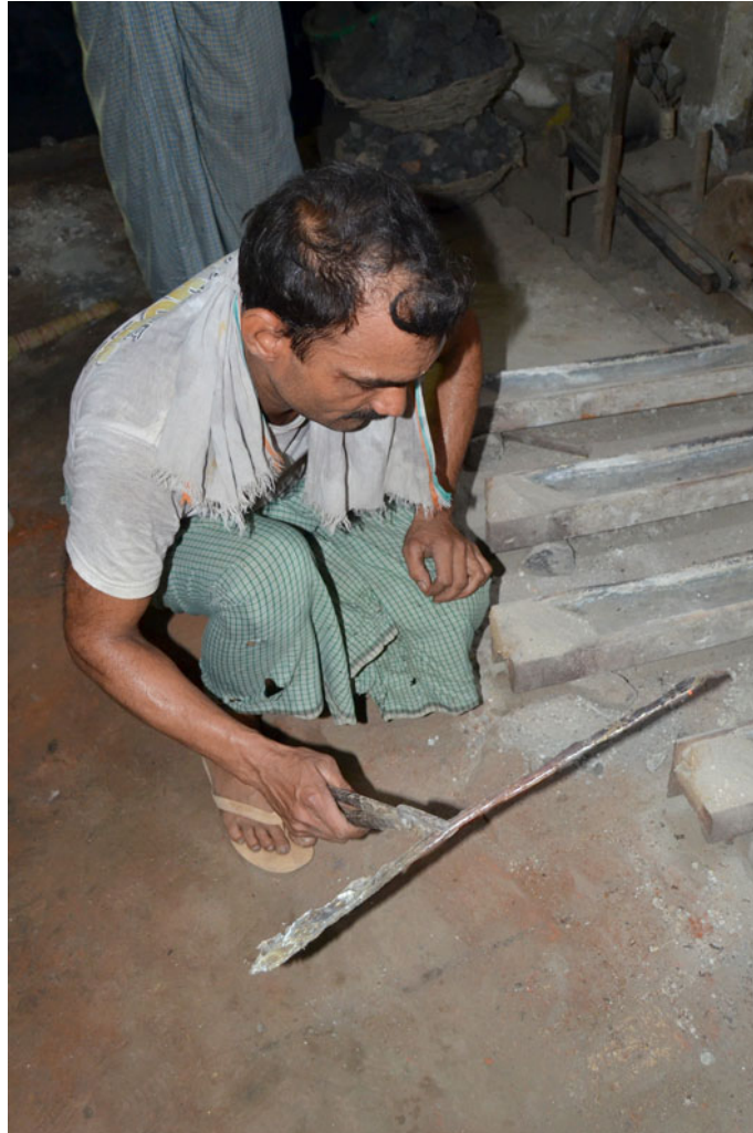
Testing the metal's ductility before pouring it out in strips.
