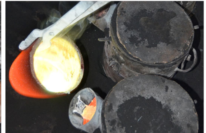
Molten brass being poured in the cavity.
