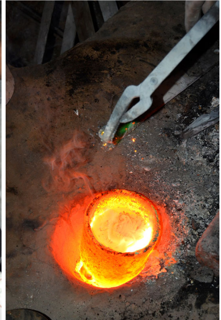
Molten brass is picked up from the furnace to be poured in the mould box
