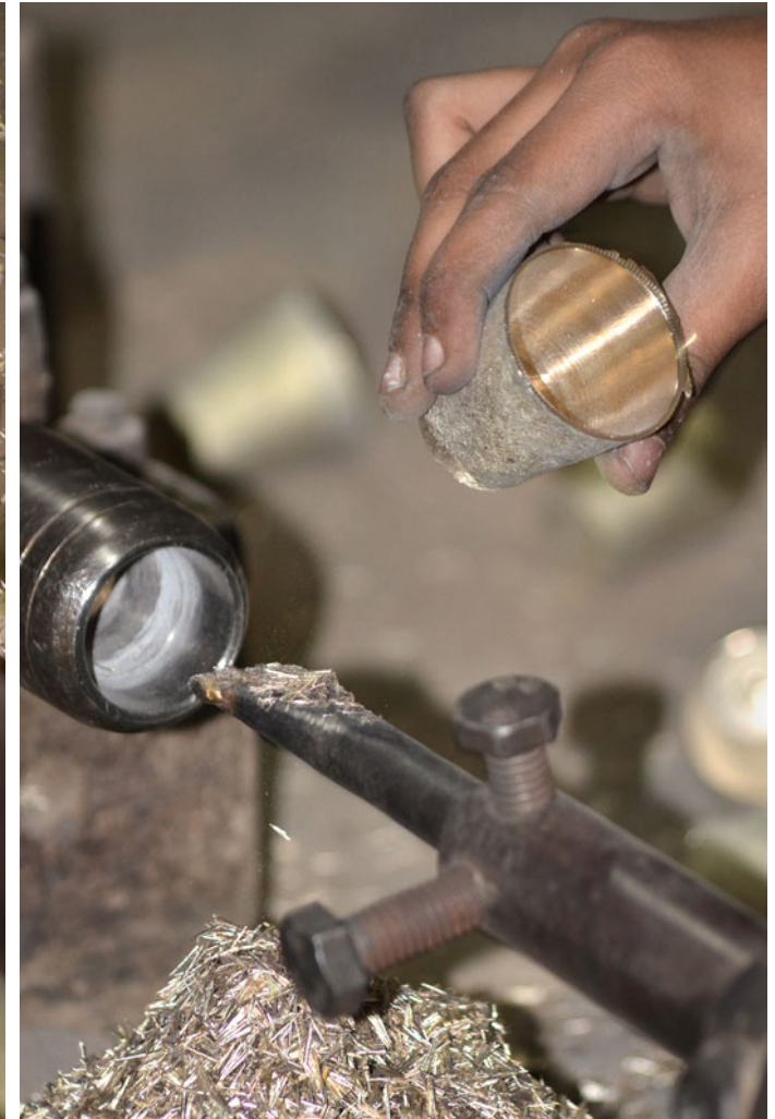
The filing tool attached to the lathe machine to scrap the tumbler.
