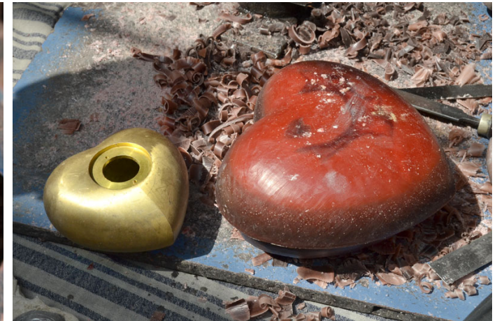
A brass cast heart and its corresponding wax mould (different size).
