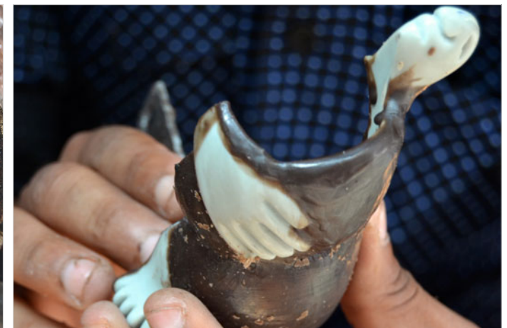
Mould for pen stand being made in wax.
