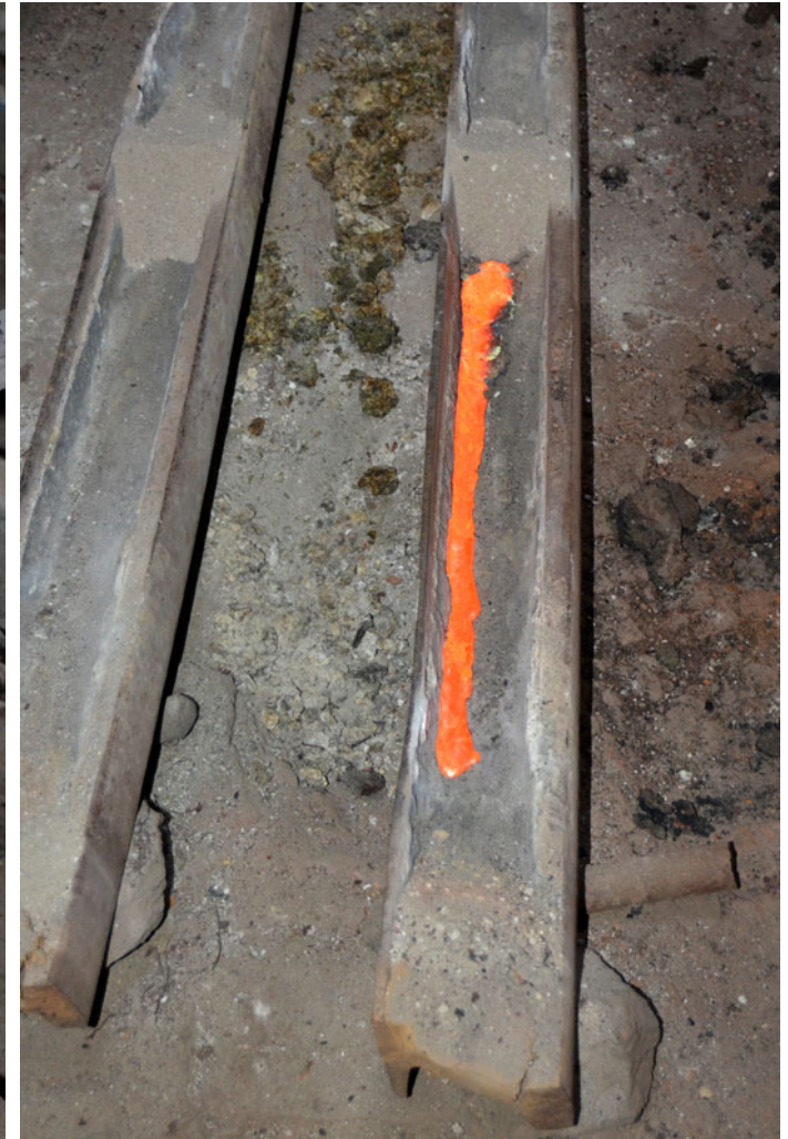
Molten metal being poured in the mould.
