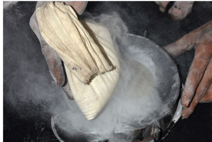
A karigar preparing the mould box with the 'master-copy' and sand.
