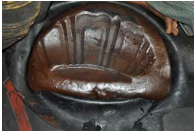
Shellac is used to stick the brass pot to the power machine.
