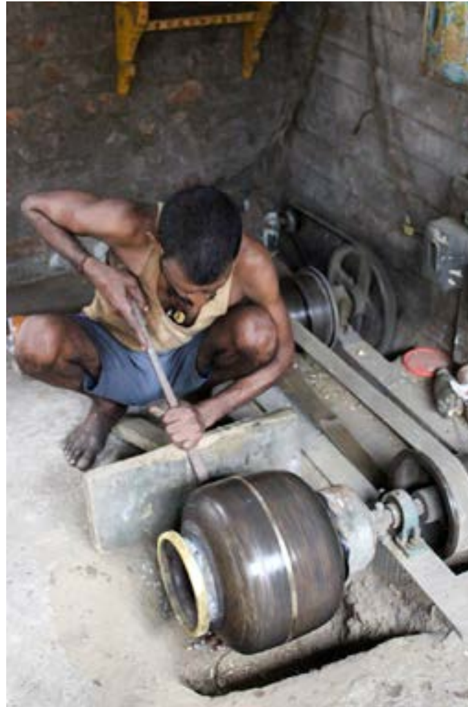
The artisan is placing the sharp iron rod closer to the brass pot and turns on the machine.
