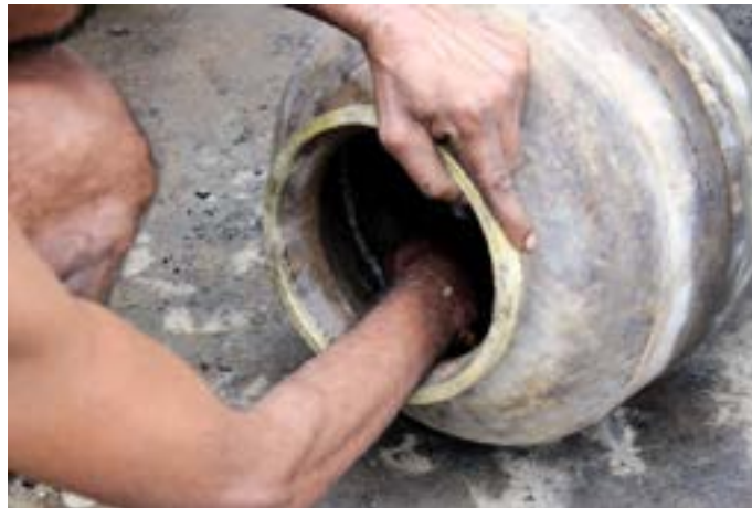
The adhesive paste is being applied to the joint of the upper and lower body part of the pot.
