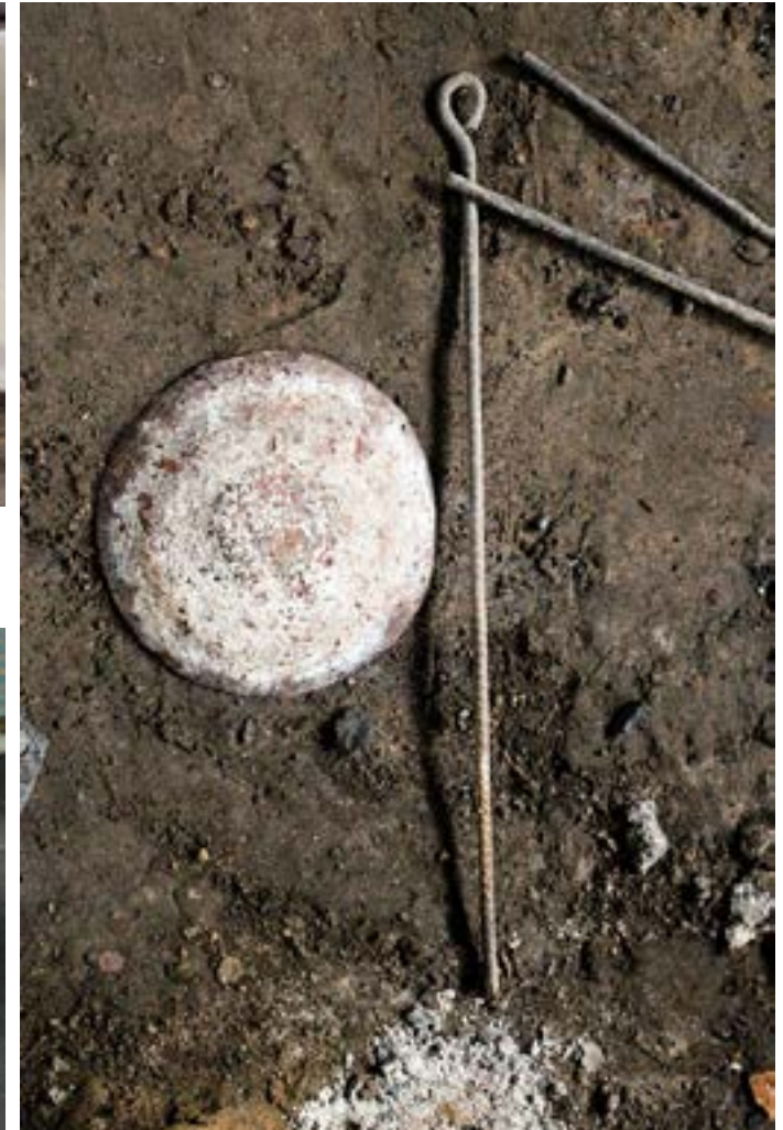
The iron rods are used to rub over the attached part of the pot while heating.
