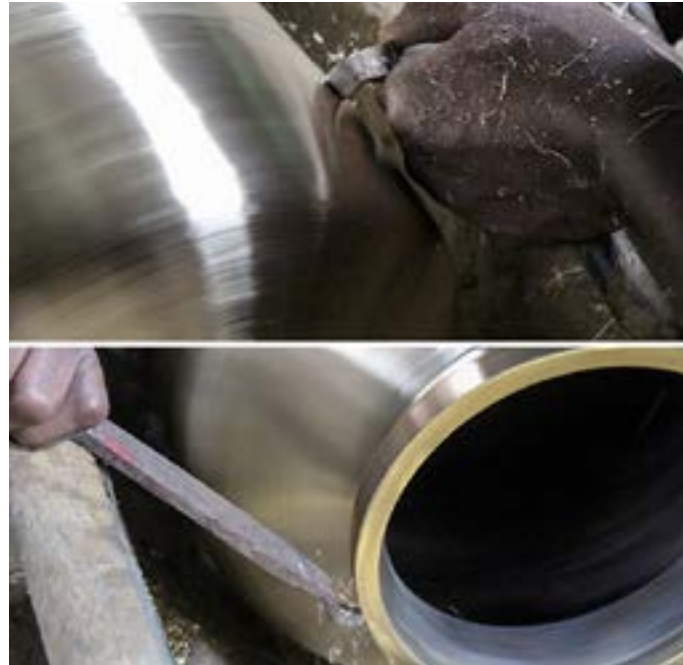
The artisan is scraping out the waste layer over the brass pot.
