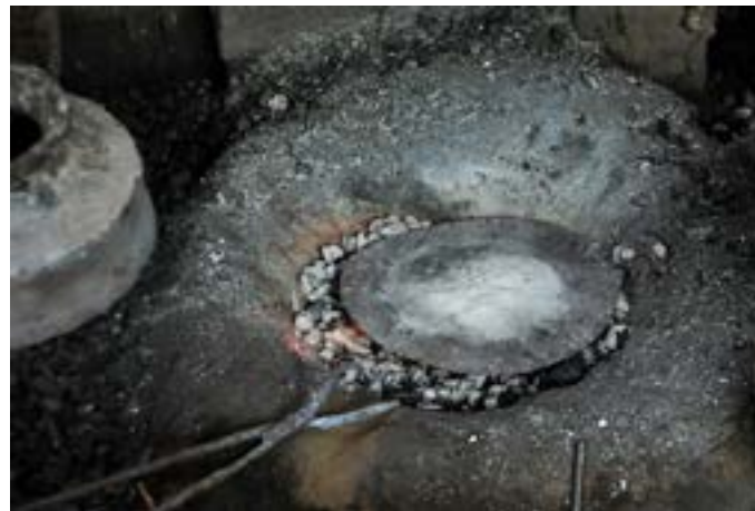
Copper and zinc powder are being heated at an average degree temperature.
