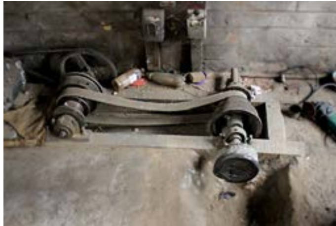
A power machine is used to stick the pot's bottom by using shellac to the machine and rotate in speed.
