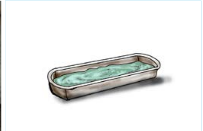
Tamarind water is used to clean the dark layer and the surface of the brass plate.
