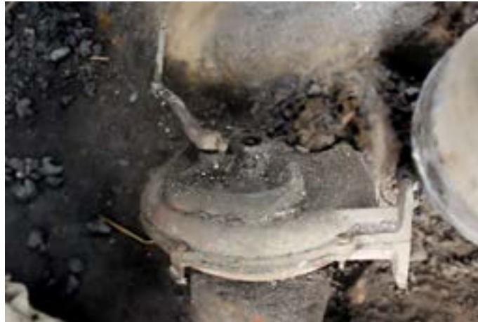
An air blower is used to increase the density of fire.
