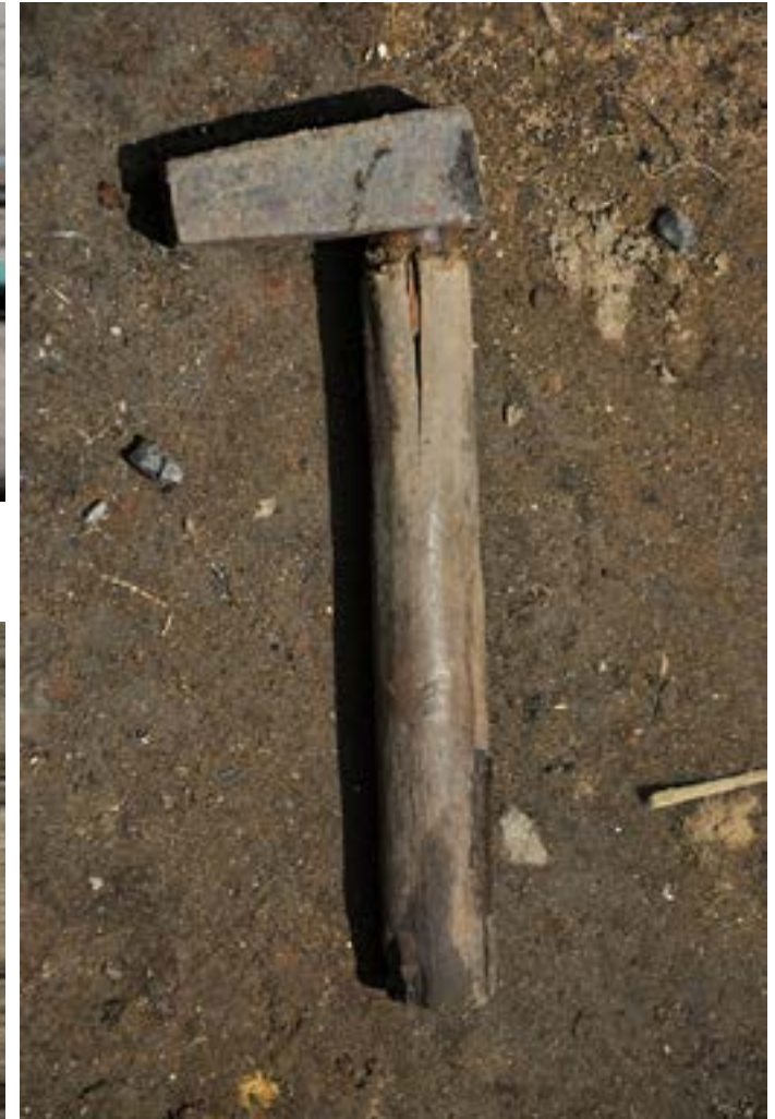
Cross and Straight pein hammer used to shape the pot.
