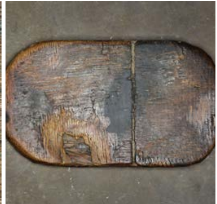
A piece of wood which is used to smoothen the surface of the iron rod.
