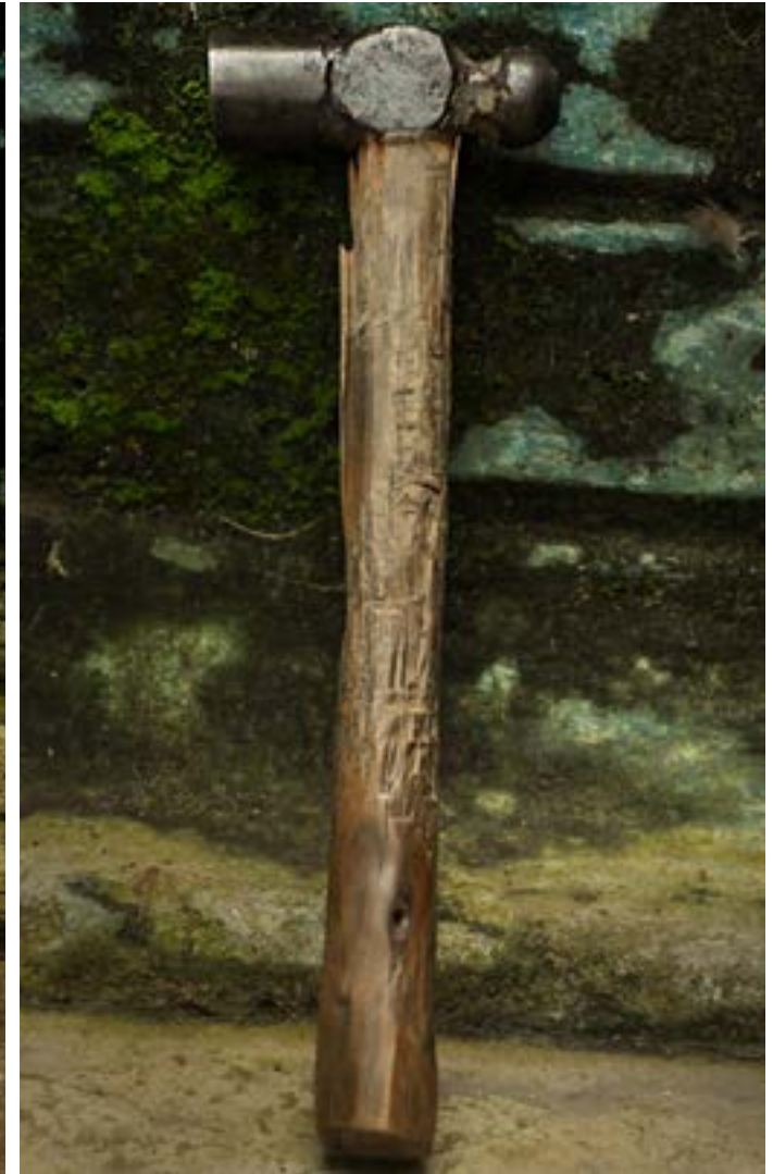
Ball Pein hammer is used to shape the circular brass to a plate.
