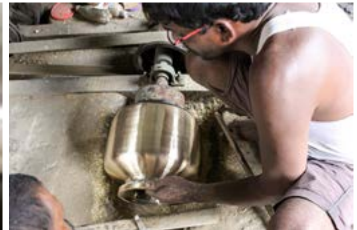
Once the scrapping is completed, an artisan is removing the brass pot from the power machine.
