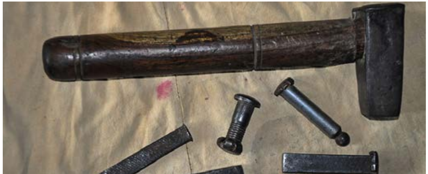
Cross and Straight Pein hammer with small stamping rods to emboss the design.
