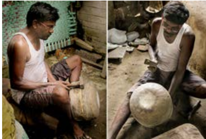
Artisan is hammering the pot with the help of level to straighten it.
