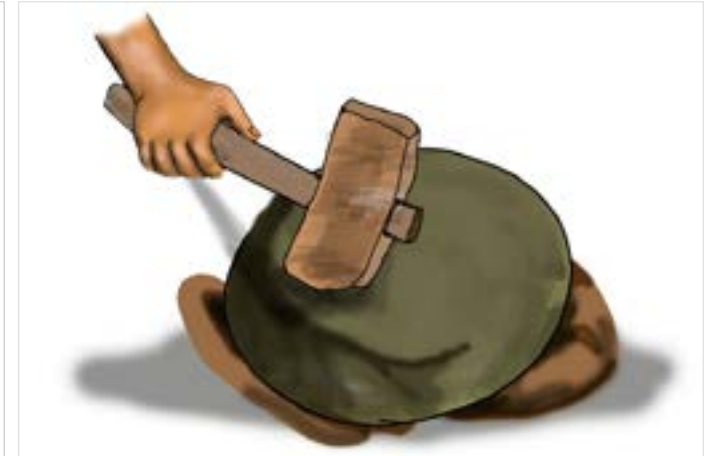
The artisan is hammering the trimmed brass sheet using a wooden hammer.
