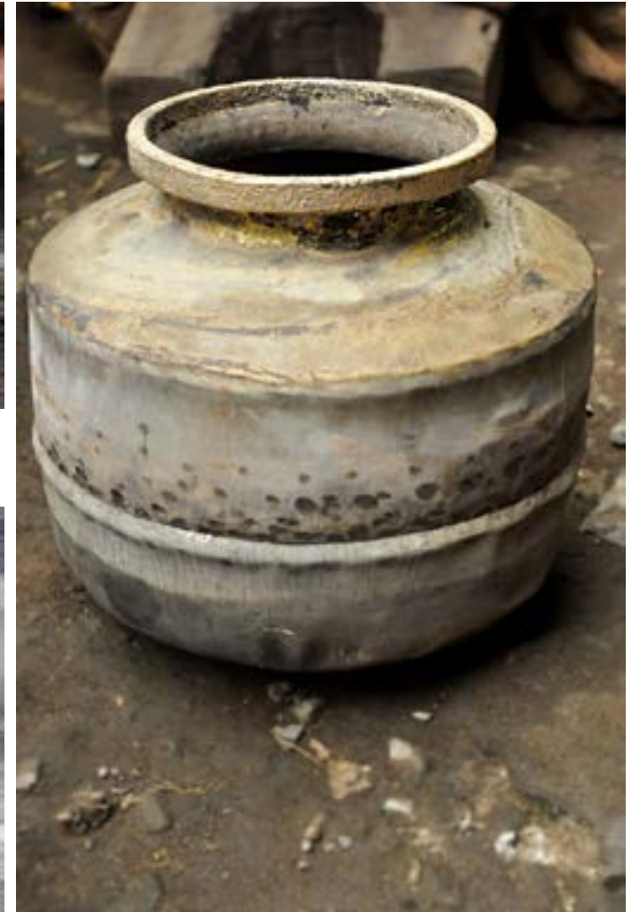
After applying the adhesive, the pot is kept to dry.
