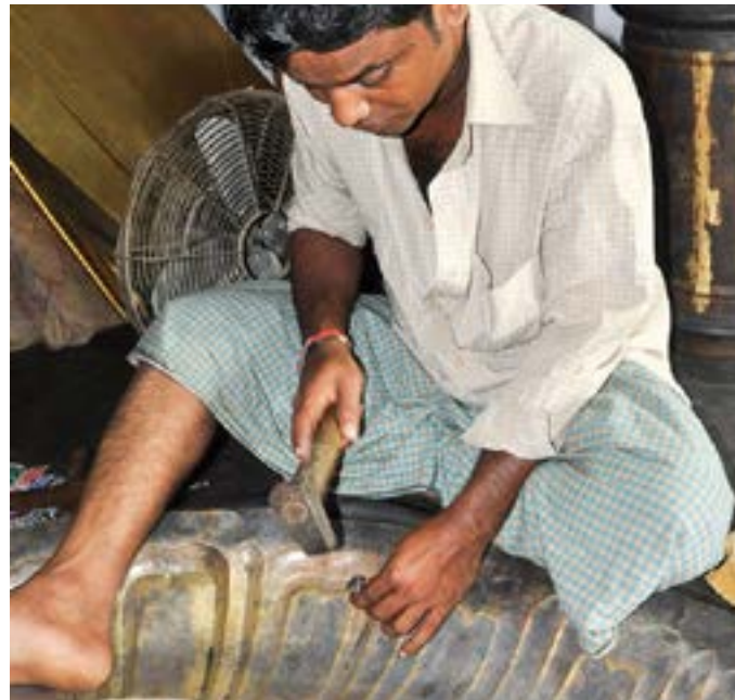
Artisan is embossing the bigger products made up of brass.
