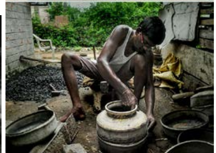
Artisan is aligning the upper and lower body part of the pot together.
