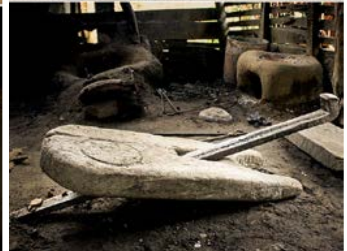
The level tool which is used to shape the pot after heating process.
