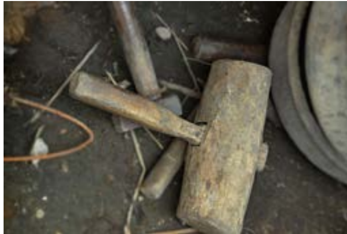
A wooden hammer is used to give a shape for the brass plate.
