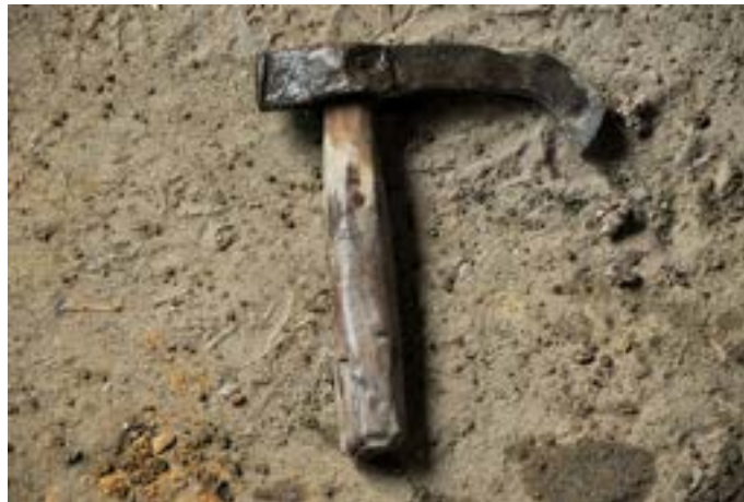
A half hatchet hammer is used to remove a dent on the pot.
