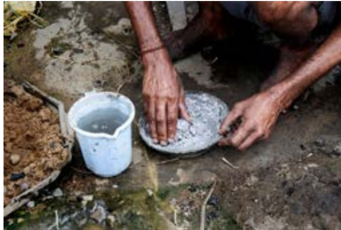
The copper and zinc powder is being mixed with the water to make it into the adhesive paste.
