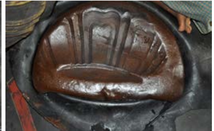
Shellac is used to fill inside the jug to emboss as per the required design.
