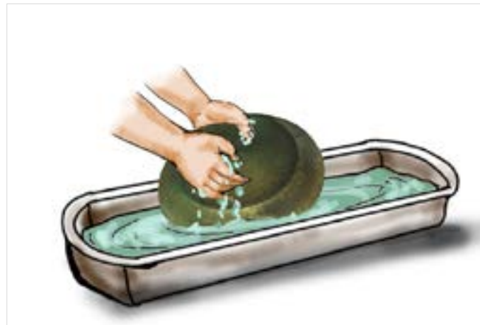
The dark layer from the brass plate is scrubbed out by using tamarind water.
