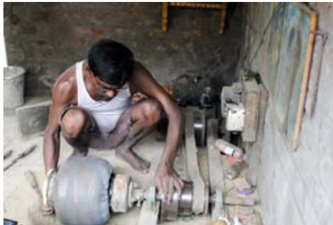
The pot is being fixed to the power machine with the help of shellac.
