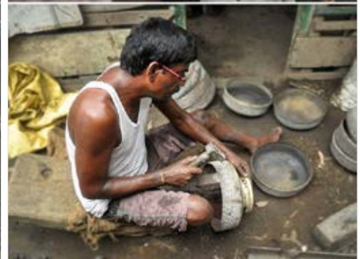
The artisan is hammering the upper body of the brass pot to get a circular shape.
