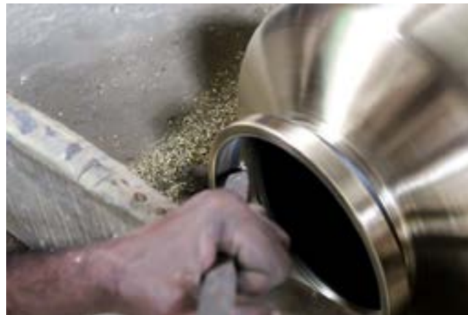
Artisan is scraping the inner layer through the head of the brass pot.
