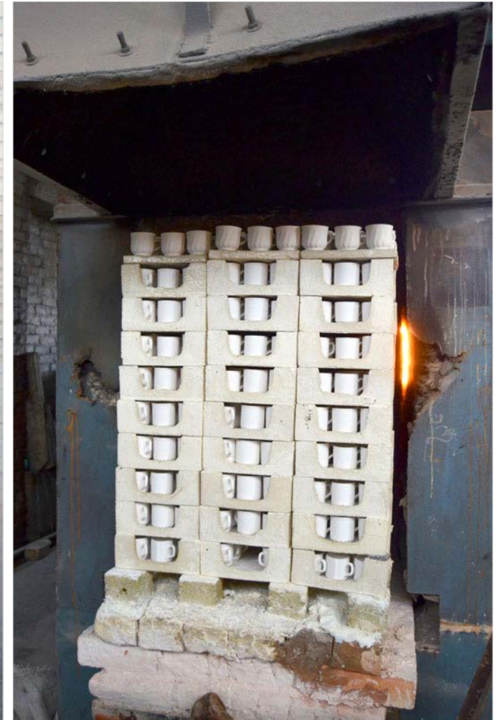
The fully loaded car entering the pre heating zone of the furnace
