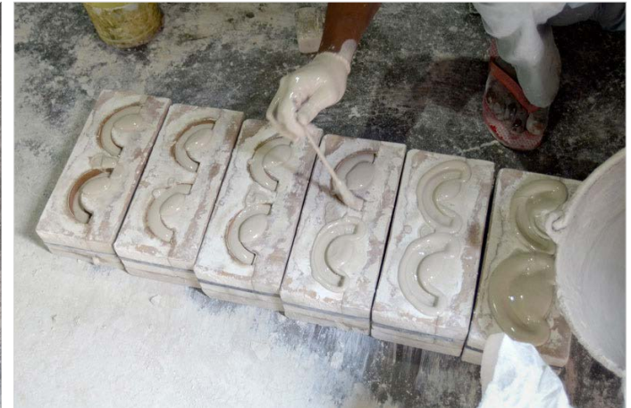
Air bubbles being removed from the POP liquid
