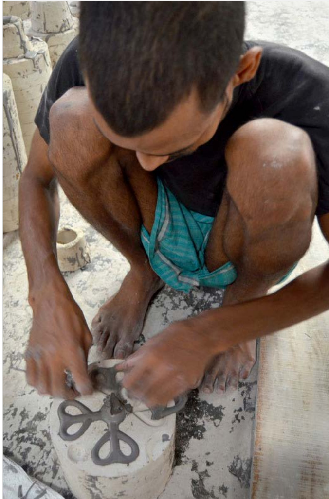
Clay handles being removed from the mould
