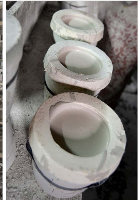
Slip (clay mixed in water) poured into the plaster moulds
