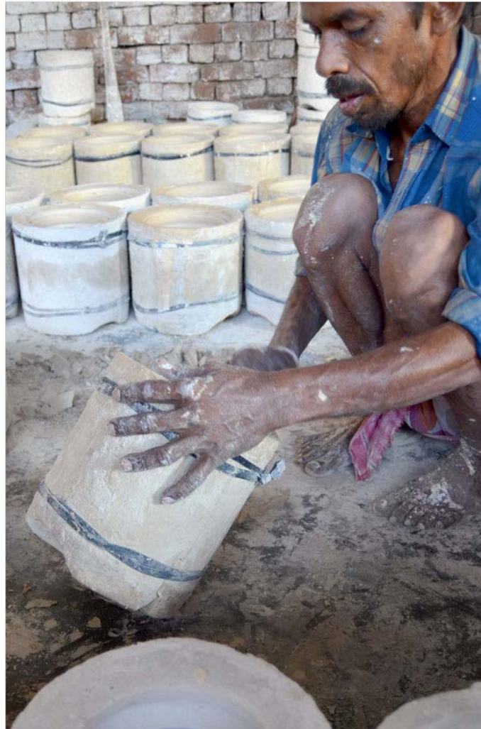
A karigar opening up parts of the mould that were held together with rubber bands
