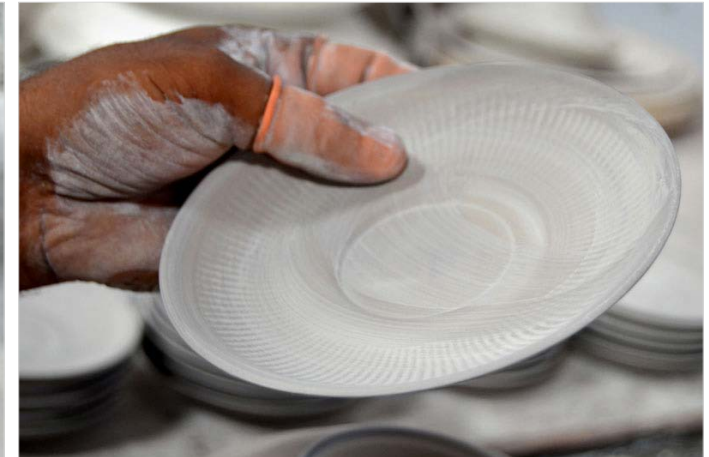
A saucer cast from a mould
