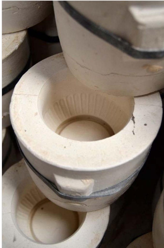
POP mould ready to be used to cast clay
