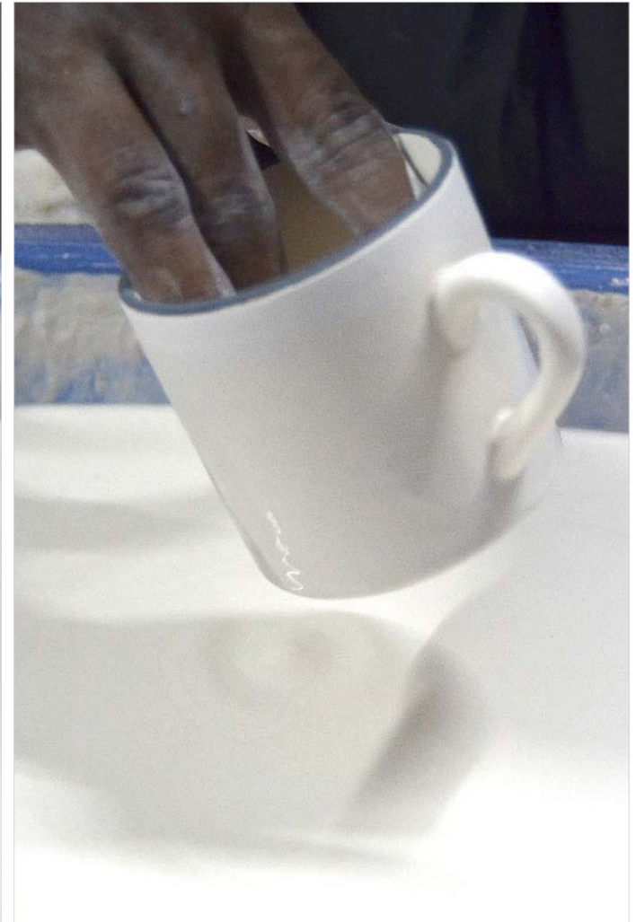
Hand-painted cups being dipped in clear glaze
