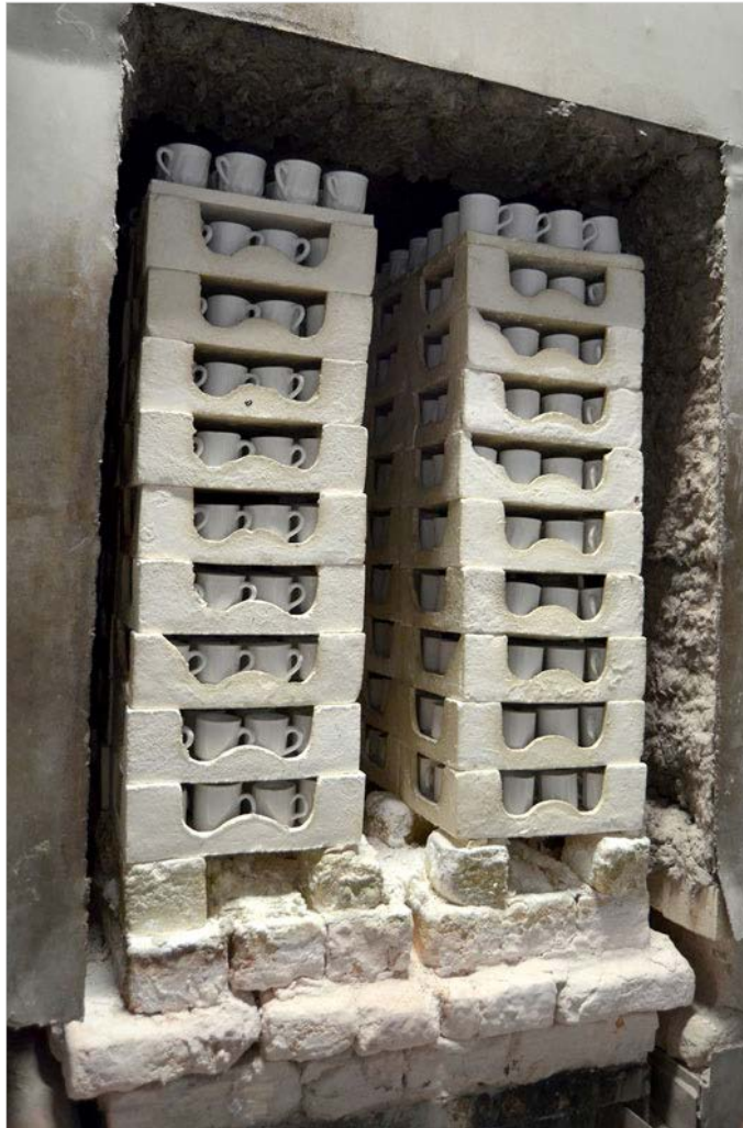
The fired cups to be removed from the cooling end of the furnace
