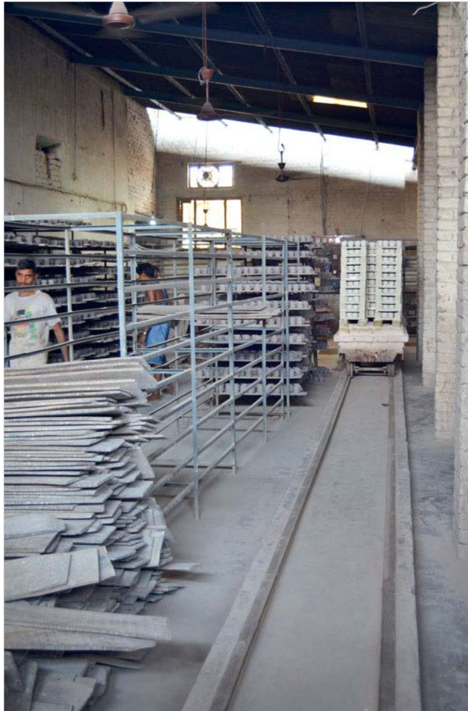
The fully loaded car of the furnace
