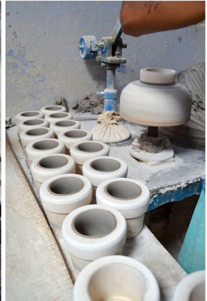
Clay being 'thrown' in along the walls of the mould using a hand tool on a rotating wheel-head
