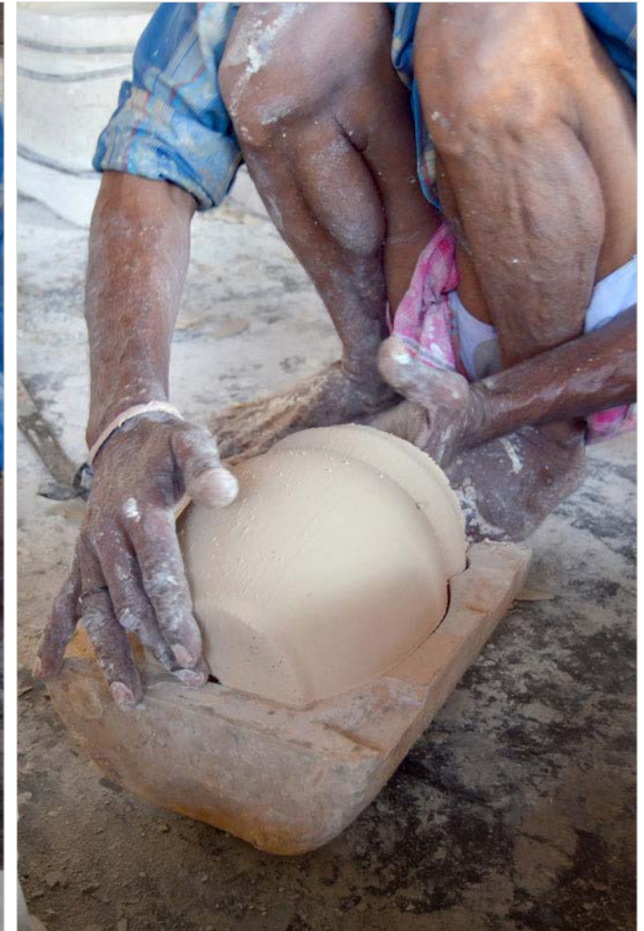
The karigar removing the clay pot from the mould
