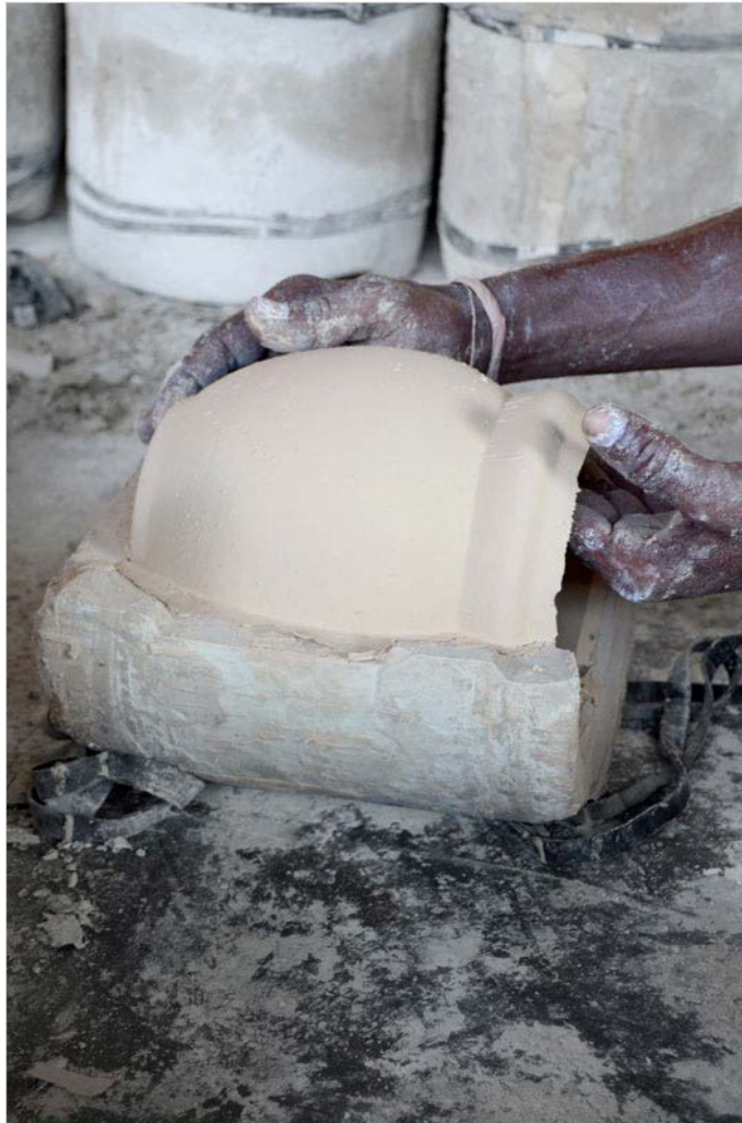
The karigar removing the clay pot from the mould
