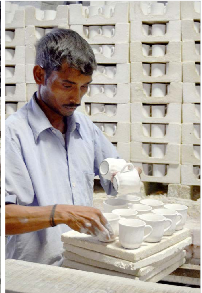
A karigar loading the car trays with cups
