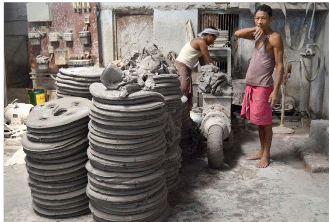
Clay cakes (discs) made by the filter press alongside a pug-mill
