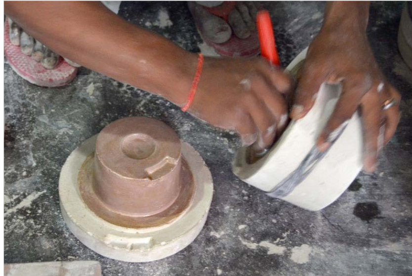
Soap and oil being brushed on the mould
