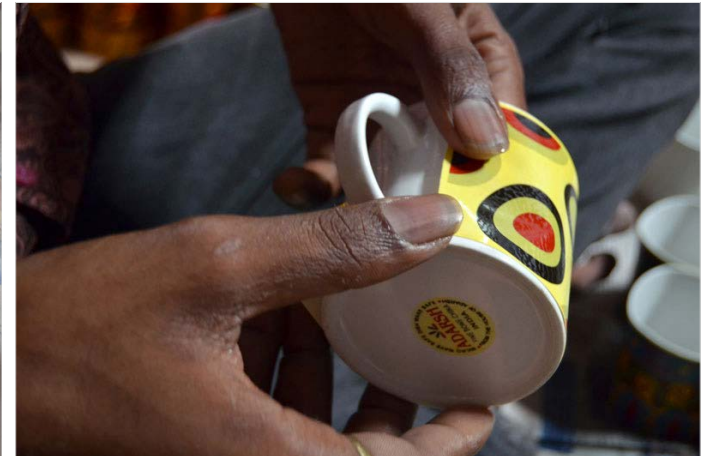
Sticker peel being placed on to the cup
