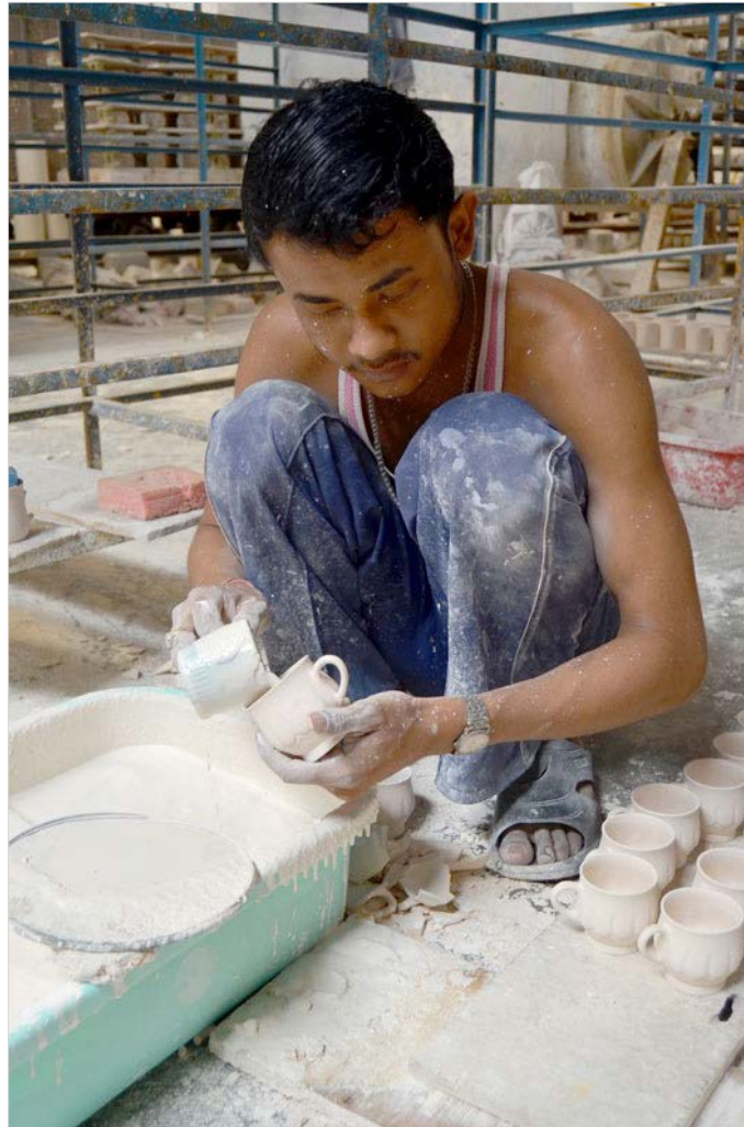
Clear glaze being poured inside as well
