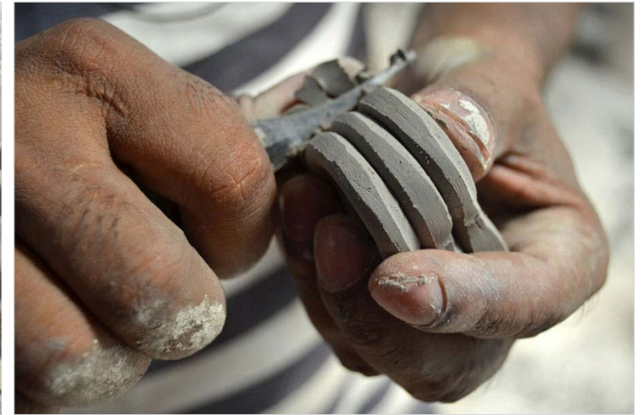
Clay handles being trimmed and finished
