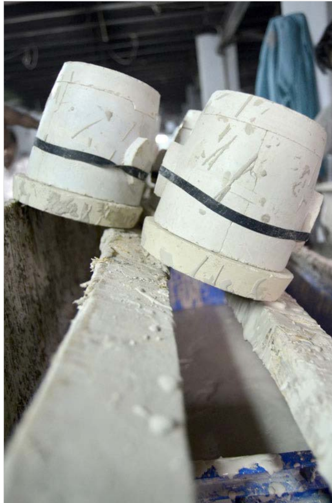
Excess slip being poured out from the mould
