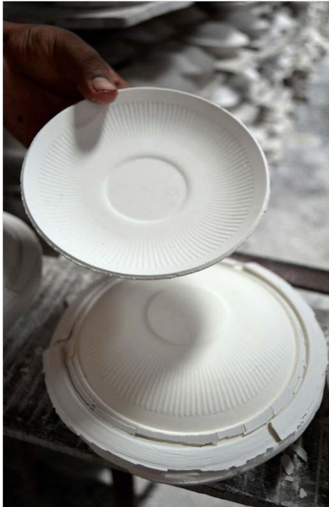
A saucer cast from a mould
