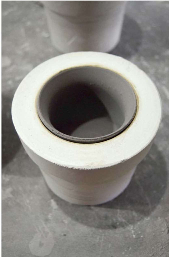
Clay, dry enough to be removed from the mould
