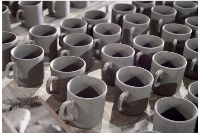
Clay handles just joined on cups
