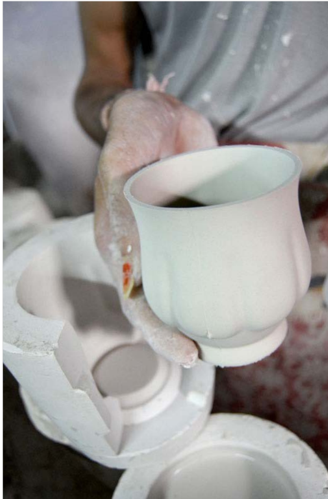
Clay cast being removed by opening up parts of the mould that were held together with rubber bands
