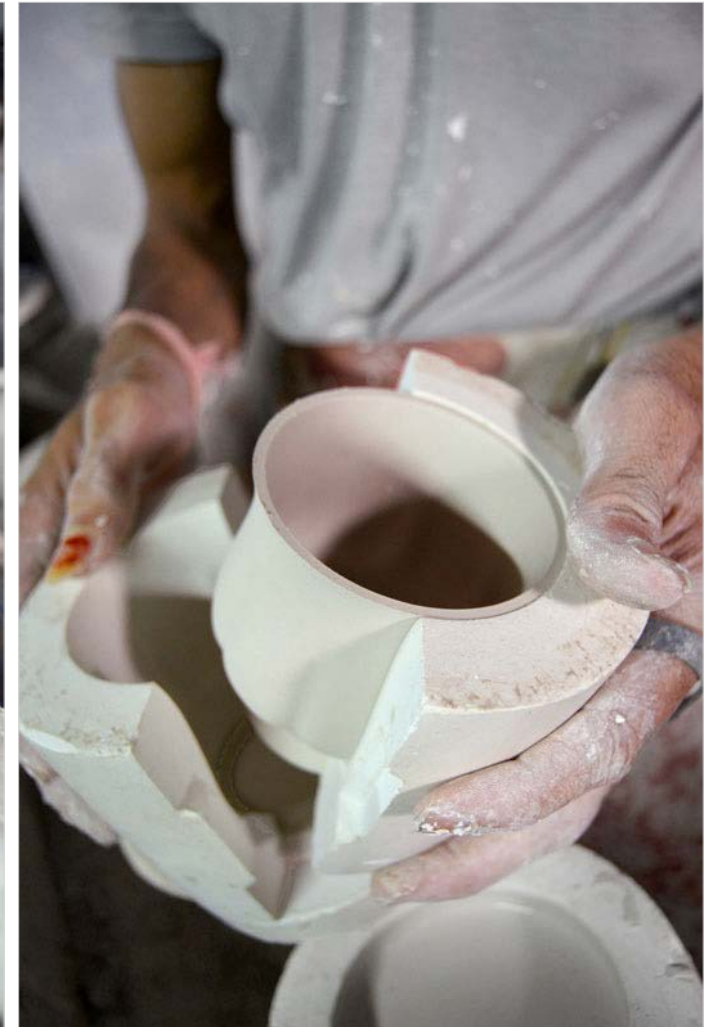
Clay cast being removed by opening up parts of the mould that were held together with rubber bands
