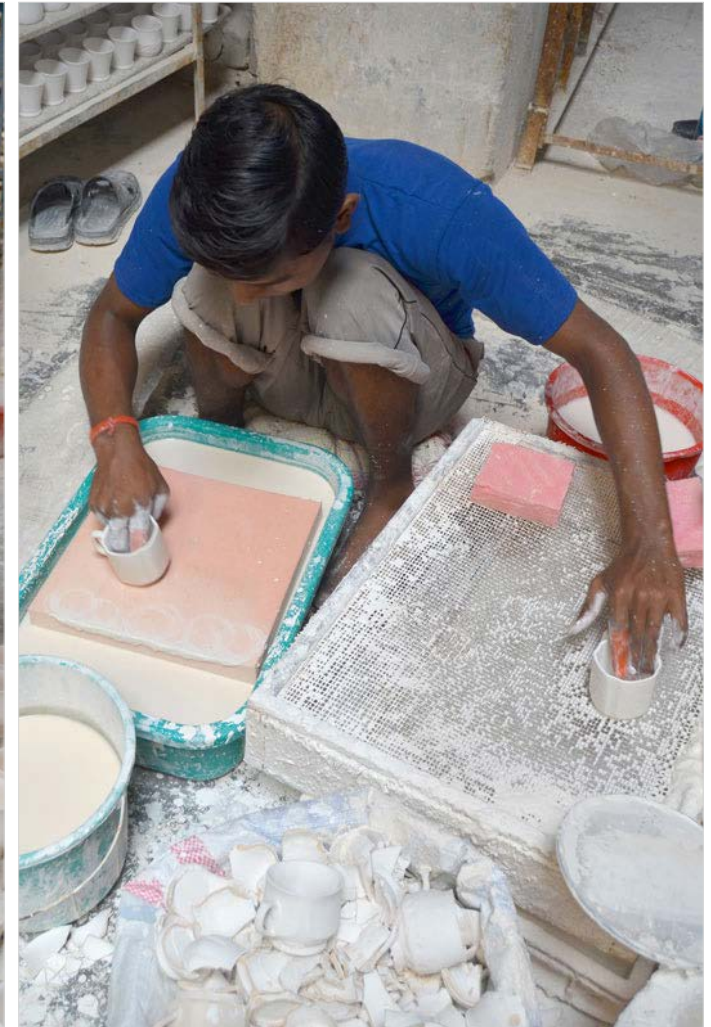
A karigar rubbing off the glaze from the bottom to prevent it from sticking on the furnace shelf
