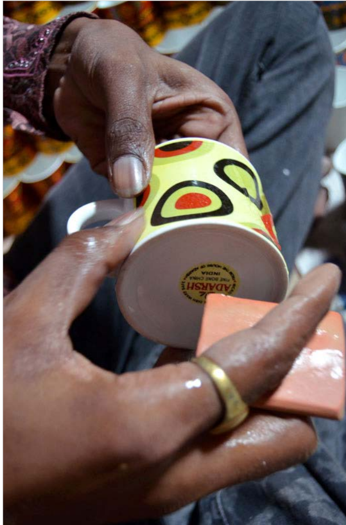
Sticker peel being placed on to the cup
