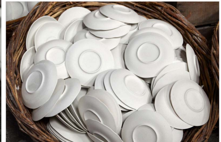
Saucers cast from a mould
