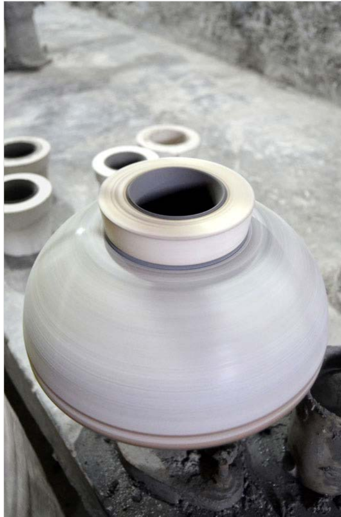
Clay being 'thrown' in along the walls of the mould using a hand tool on a rotating wheel-head
