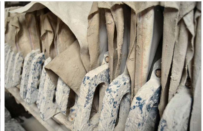
Clay discs in the filter press (pressed between metal plates and canvas)
