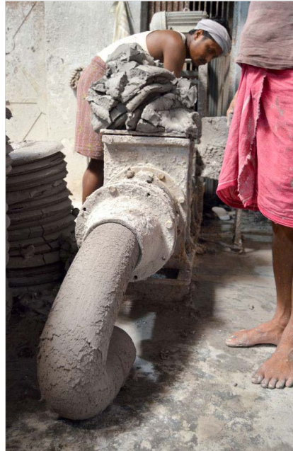
Clay being rolled out from a pug-mill
