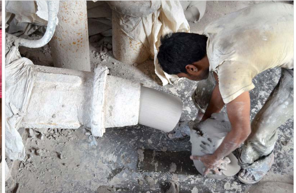
Clay being rolled out from a pug-mill
