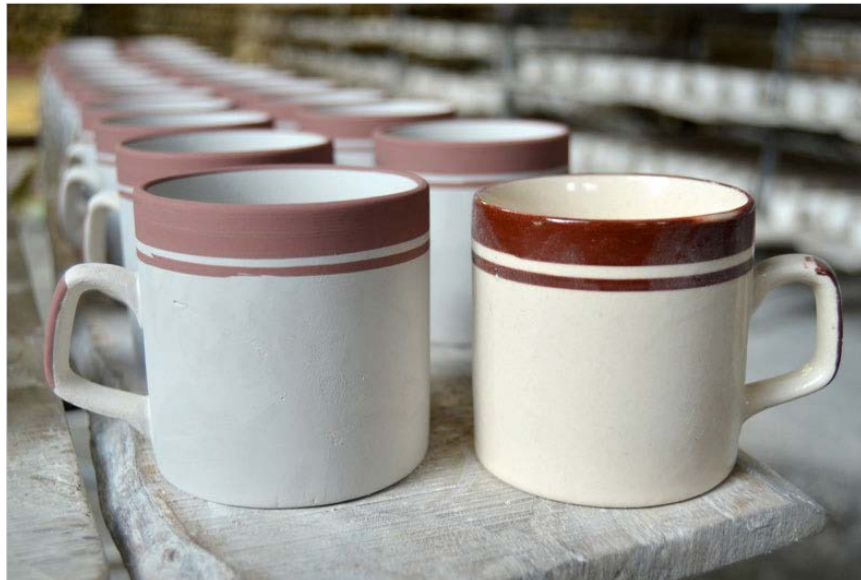
Difference between an unglazed and glazed cup
