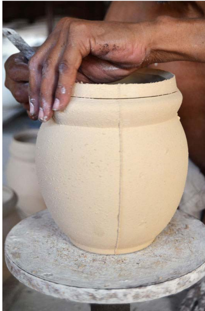
The karigar trimming the rim of the pot
