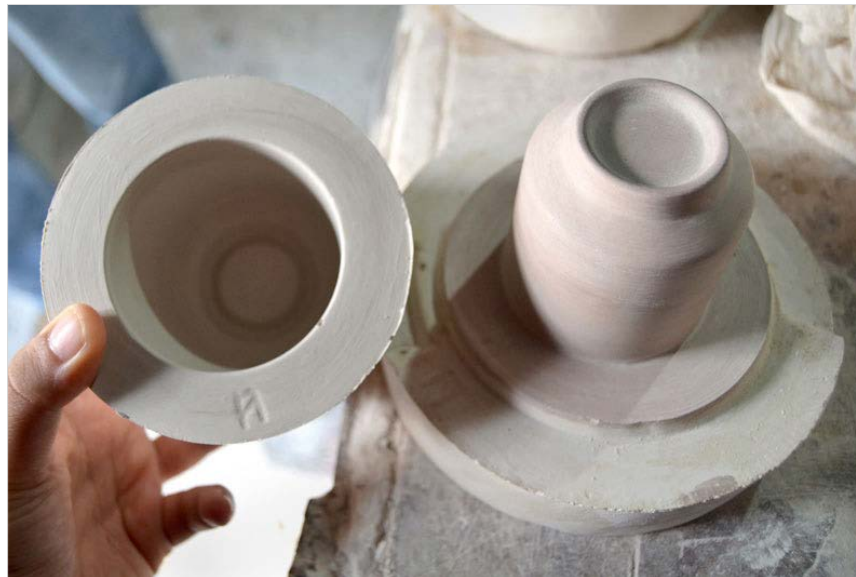
POP mould ready to be used to cast clay
