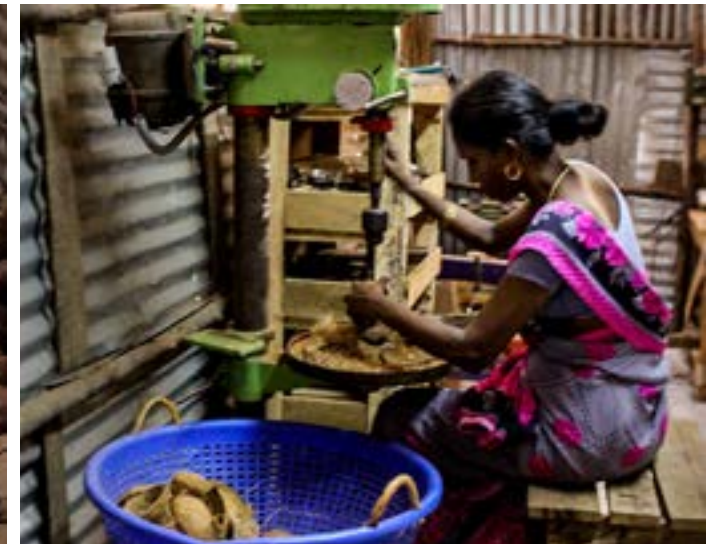
Artisan uses jigsaw machine for making hole in the coconut shell.
