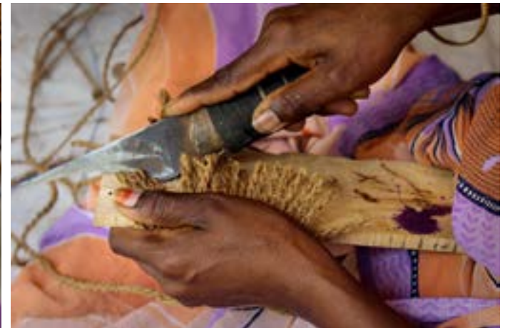
The rolled thread is cut using a sharp knife.
