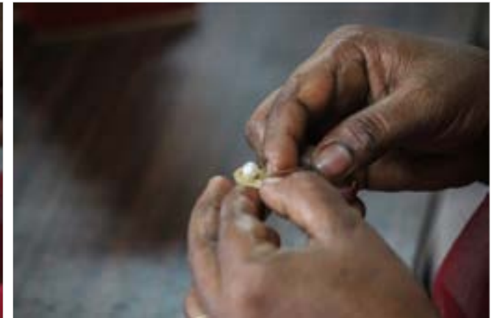
Pearl is sewn by using needle and coir fiber.
