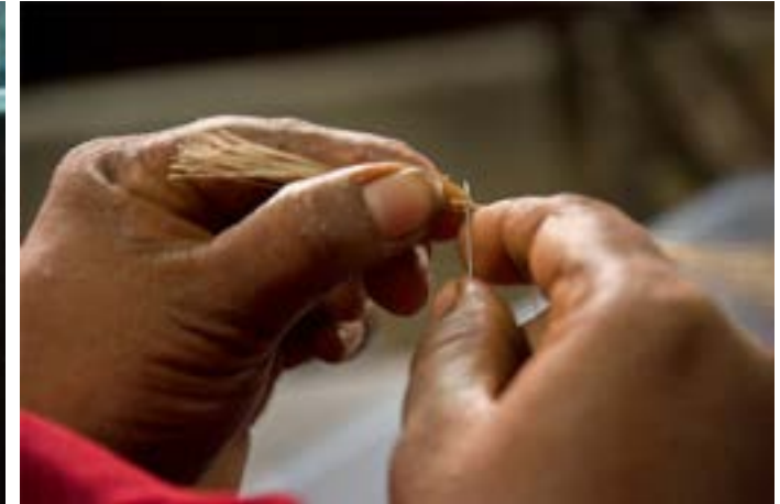
Sewing the coir bundle using needle.
