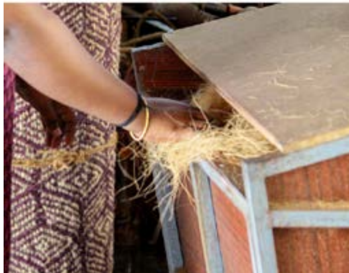
Coir fibers are softened using coir softening machine.
