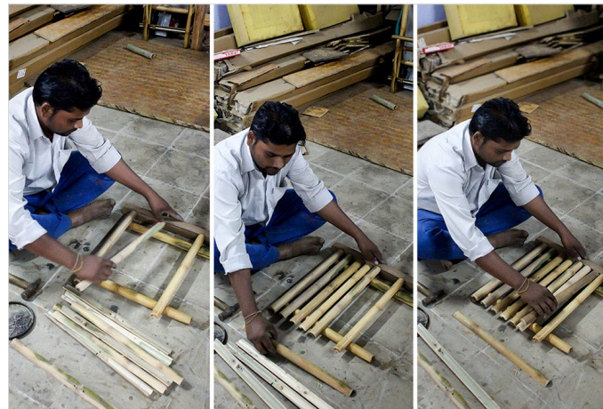
The newly sliced bamboo pieces being arranged on the ready frames.
