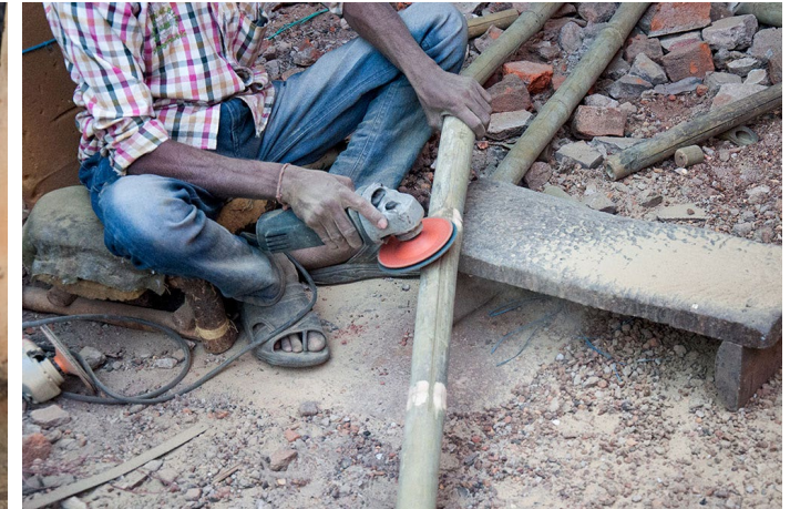
The artisan is using a power sander to remove the roughness of the raw bamboo.
