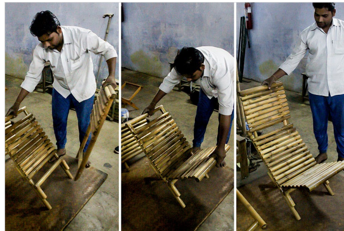
After the bamboo frames dry, the artisan fixes them together to form a strong chair.
