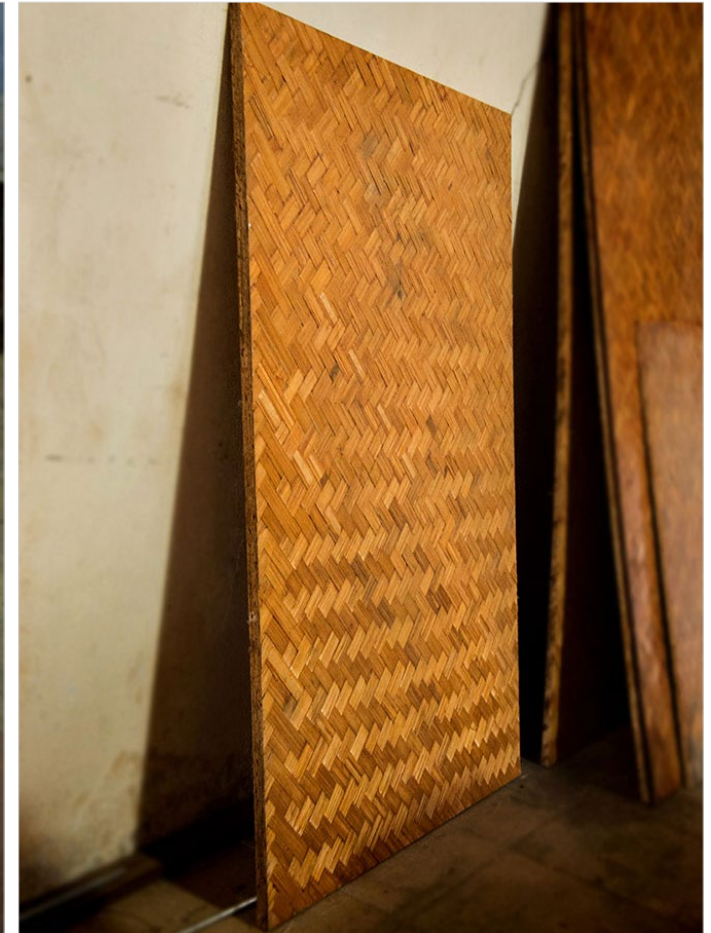
A bamboo shade is used to cover open spaces and walls, to protect against harsh climate.
