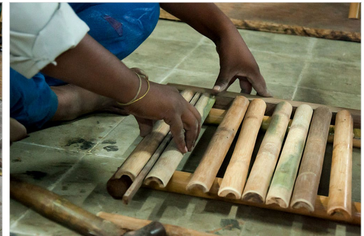
Artisan is measuring equal gaps between bamboo pieces.
