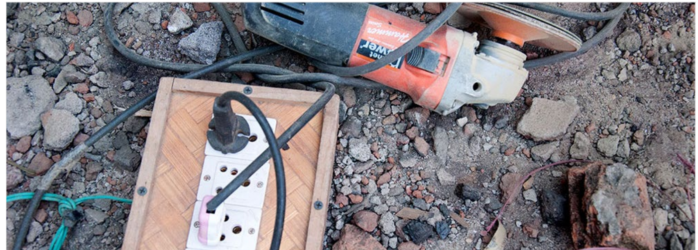
A power sander used to grind roughness from the raw bamboo stem.
