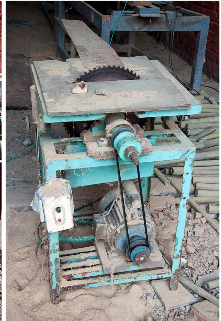
A table saw is used to cut large bamboo stems.
