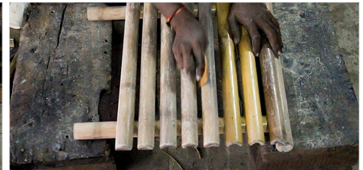
After measuring the difference, the artisan nails bamboo pieces over the frame.
