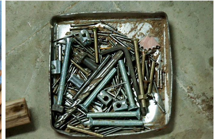
Iron nails, bolts, nuts, and Allen keys used to join different parts of bamboo pieces into a furniture item.
