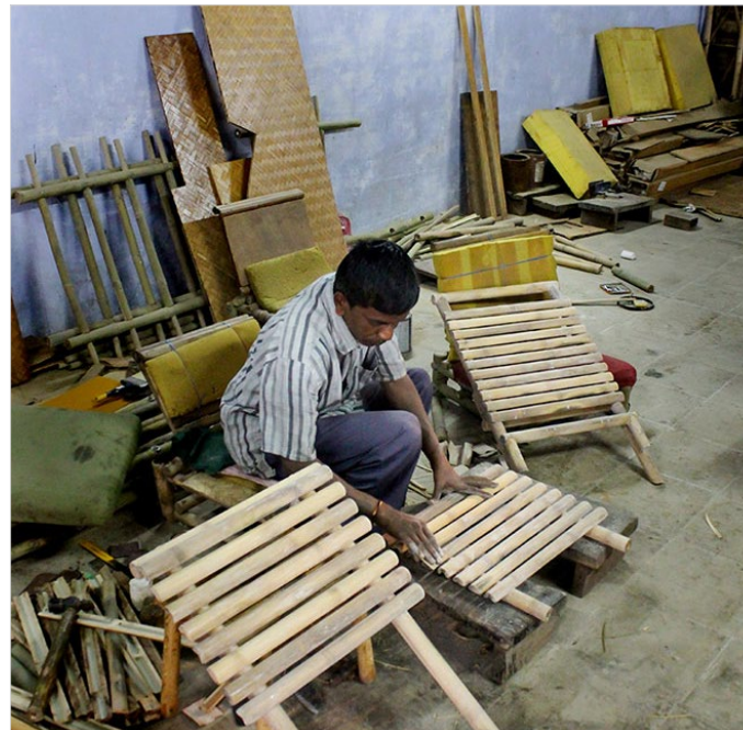
Artisan smoothing the nailed bamboo pieces using sandpaper.
