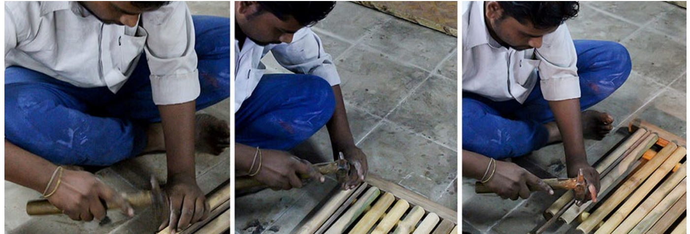
After measuring the difference, the artisan nails bamboo pieces over the frame.
