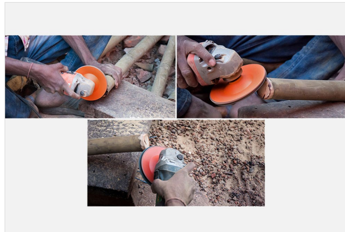
Artisan smoothing the corners of the trimmed bamboo using a power sander.
