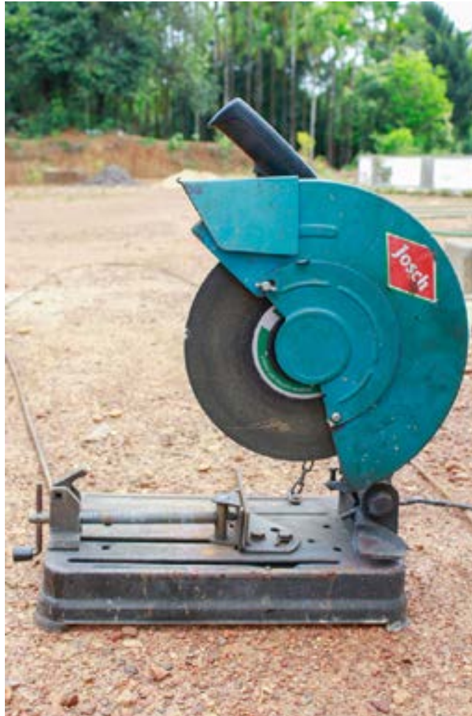
Iron bars are cut using rod cutting machine.
