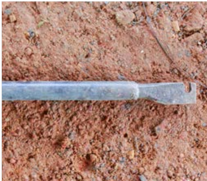
Bar bending key is used to bend the iron rods.
