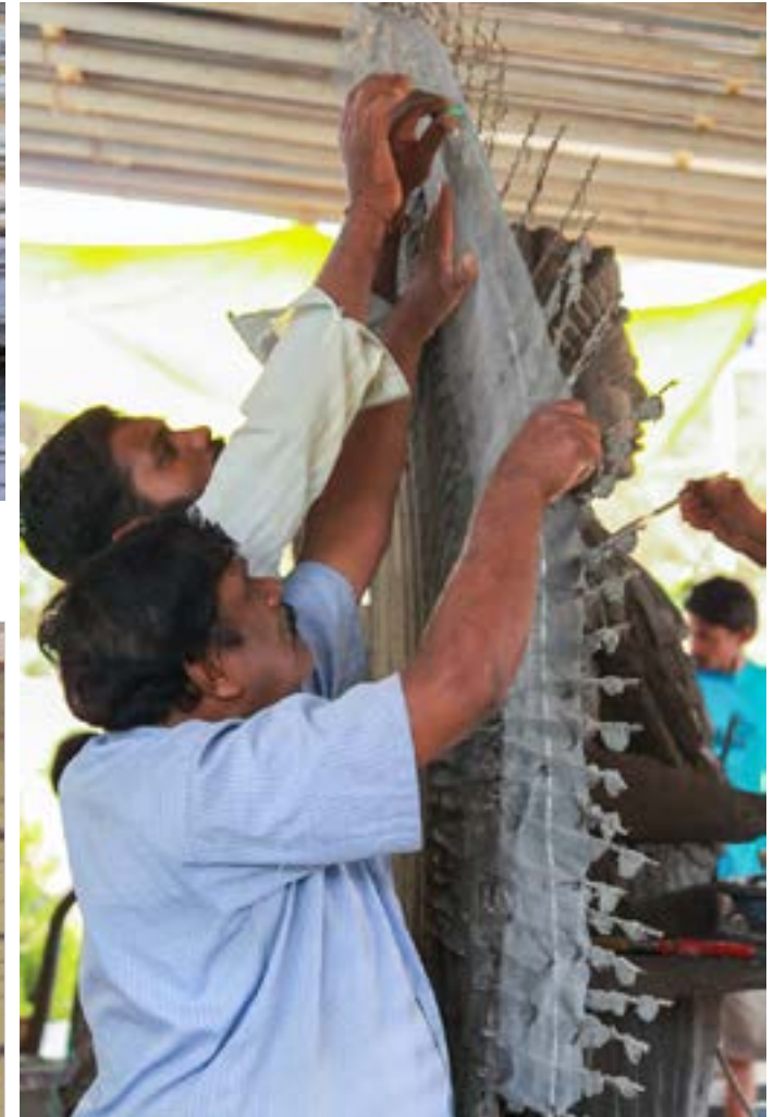
Fine Mesh is tied to the armature of sculpture to apply cement layers.
