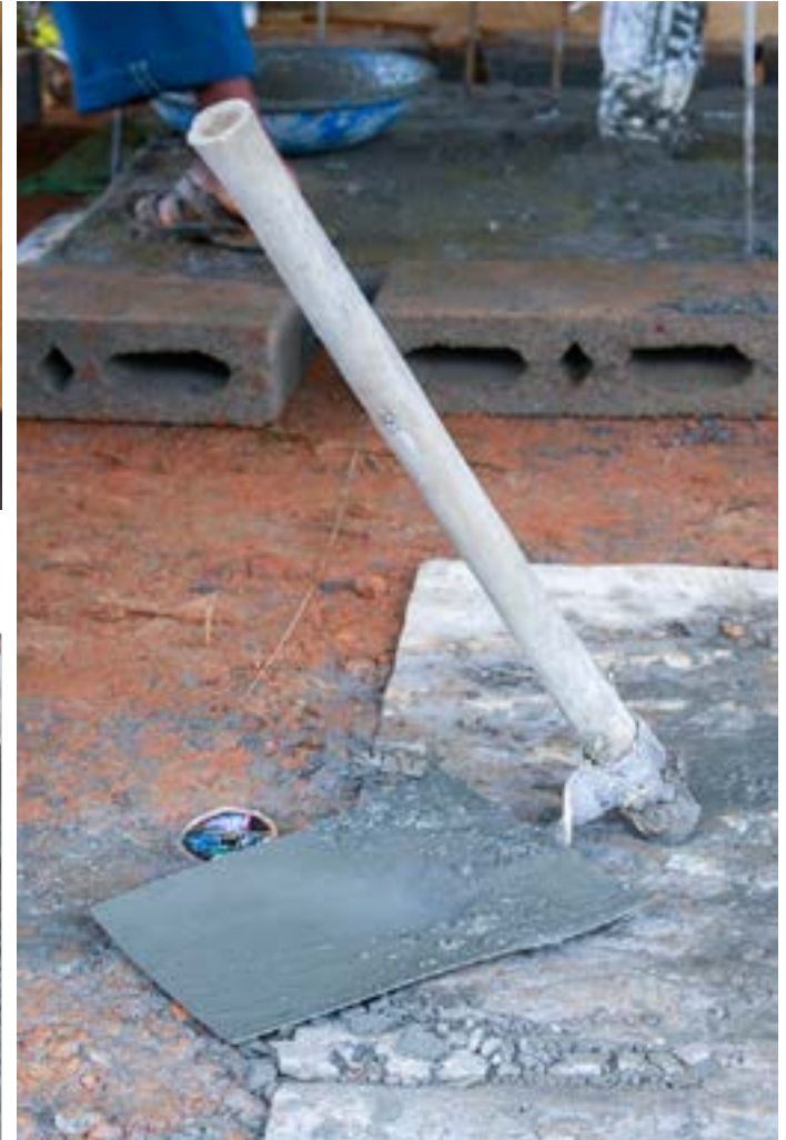
Grubber is used to mix cement.
