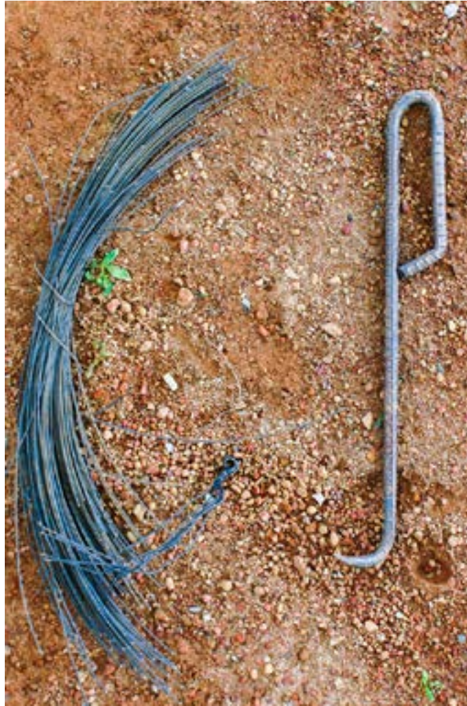
Iron hook is used to bend the binding wire.
