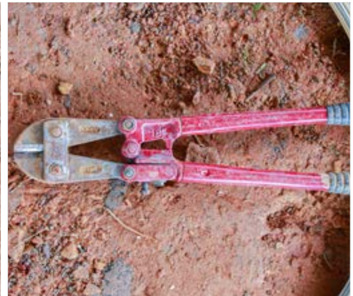
Binding wires are cut using cable cutter.
