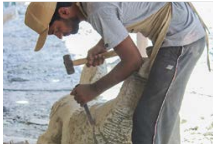
Rough carvings are smoothed by using tooth chisel.
