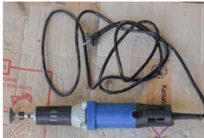
Die Grinder: The tool is used for making the designer cuttings into the stone.
