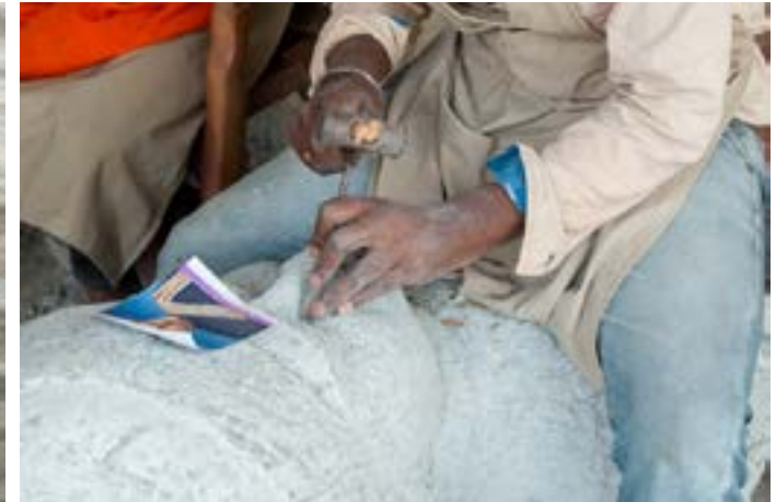
Rough shaping is done using customized chisel that helps for the further detailing.
