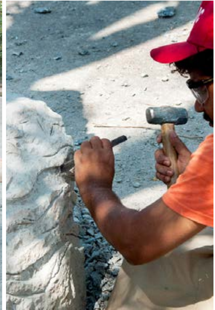
Artisan smoothing the rough surface using tooth chisel.
