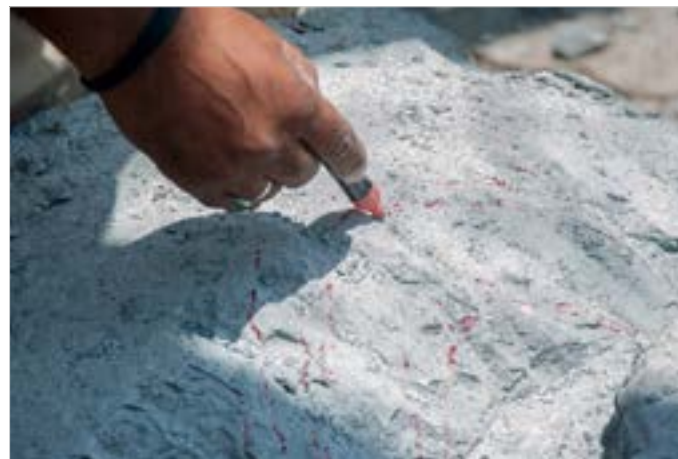
Marking on stone is done by using marker for the further carving.
