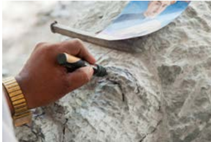
Marking on the roughly shaped stone with the help of marker.
