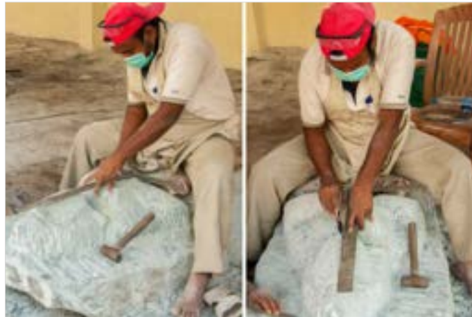
Marking a stone using L-shaped scale and marker.
