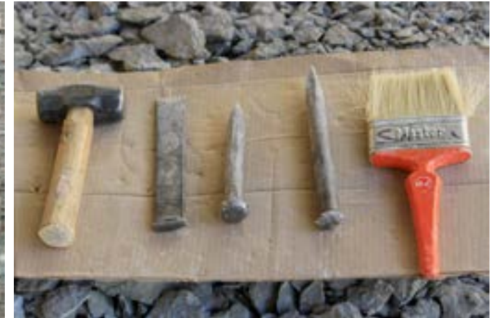
Brush: After chiseling by using various sized chisels and hammer, the brush is used for dusting the stone.
