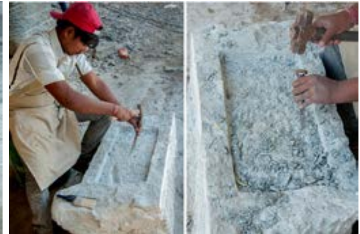
Artisan placing a point chisel on the stone to sculpt with the help of the hammer.
