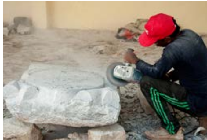
Electric cutter is used to cut the stone into required shape.
