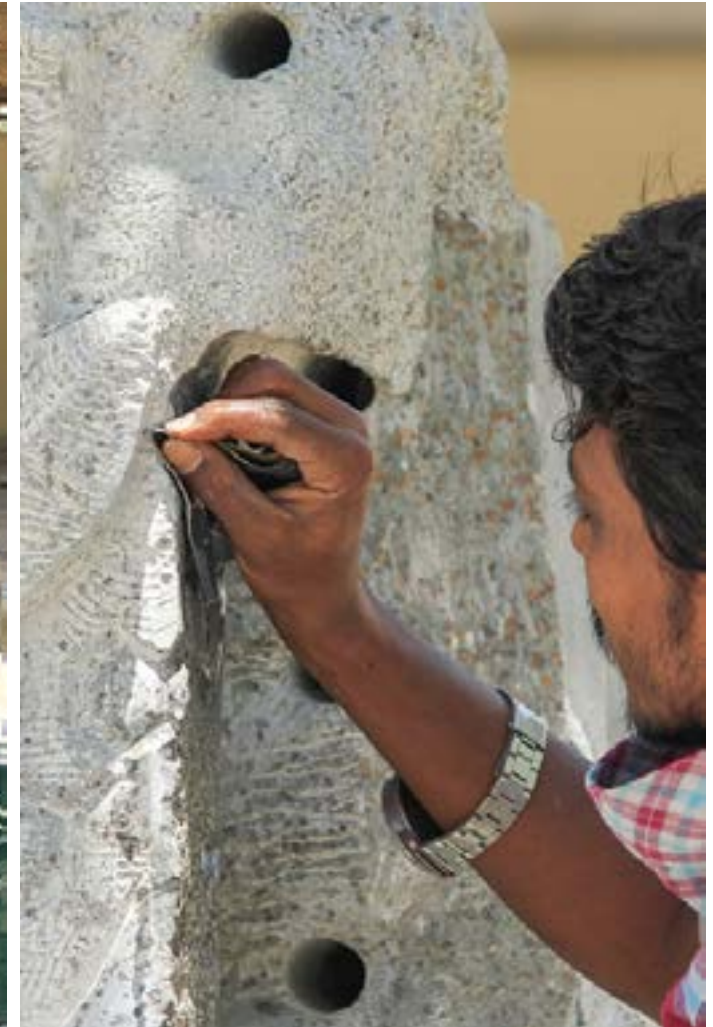
On the wet surface, sandpaper is scrubbed thoroughly to get the smooth finishing.
