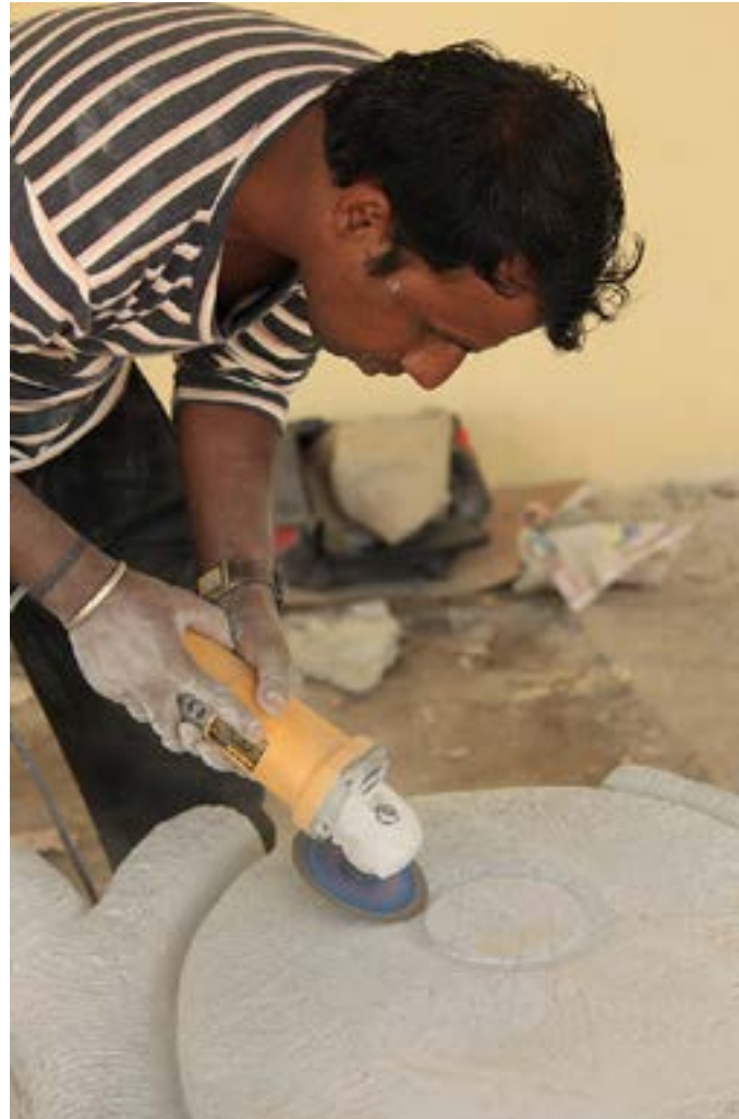
Stone is carved into the circular shape using the electric stonecutter.
