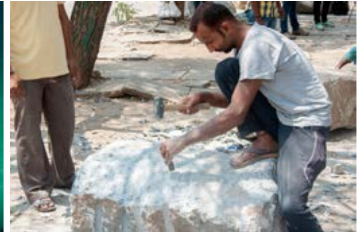
Removing unwanted stone using varieties of chisels and hammer.
