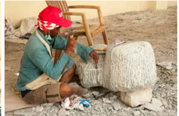
Bull point tool is hammered repeatedly by artisan.
