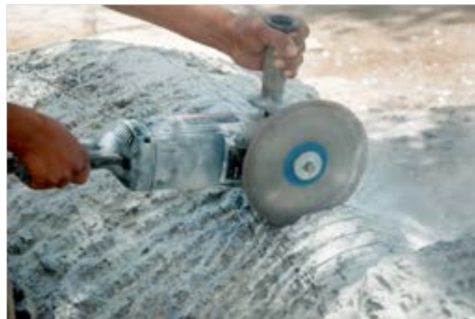
Buffing machine is used to make an impression for carving.
