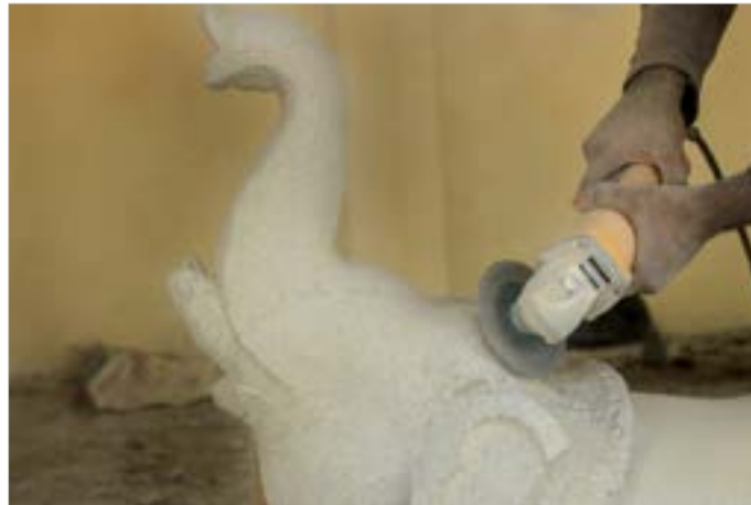
Smoothing the surface using buffing machine.
