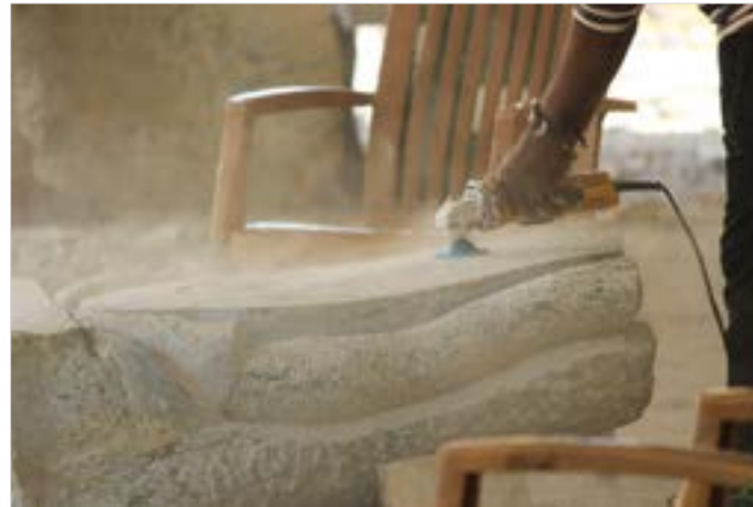
Buffing machine is used to smoothen the stone surface.
