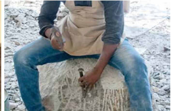
Marked areas are carved using a bull point tool.
