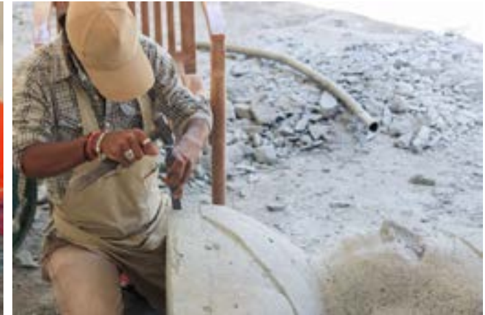
Removing the unwanted stone carefully for the neat finish.
