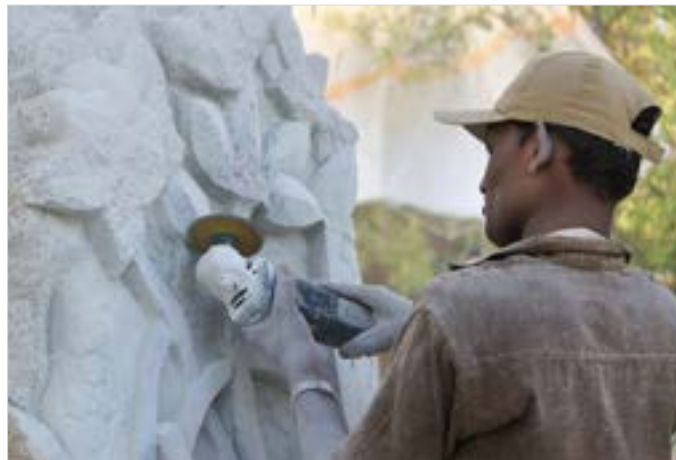
The designs are given sharp margins by using motorized cutting tool.
