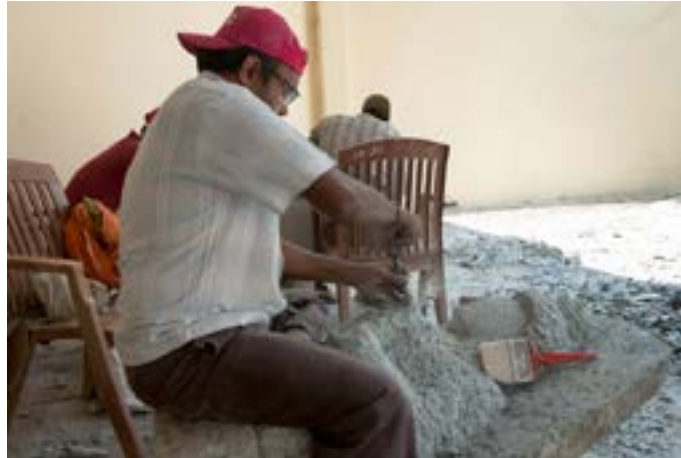
Roughing out the stone by hammering a bull point chisel.
