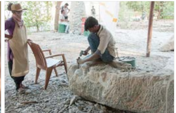
As per the marking, preliminary round of carving is done.
