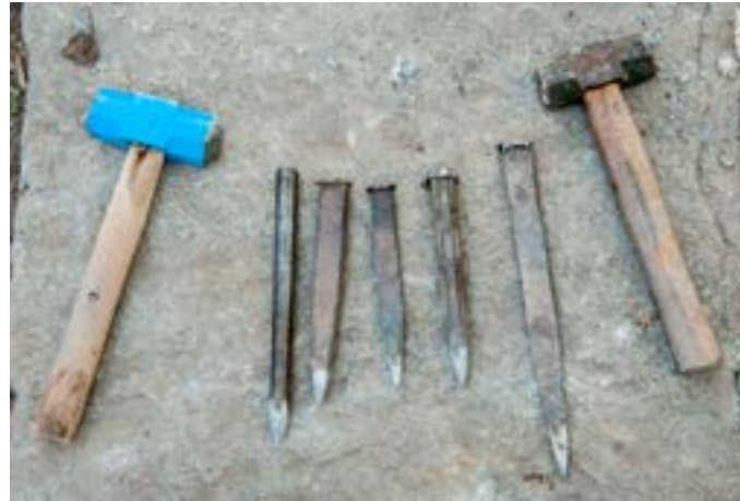
Chisels and Hammers: These tools of various sizes are used for sculpting the stone.
