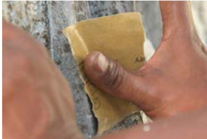
Sand Paper: It is used for polishing the surface.
