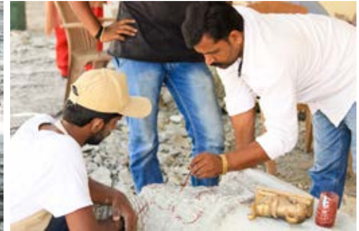
Marking on a roughly carved stone using round brush and red oxide.
