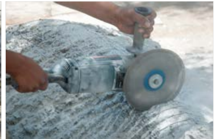
Cutting Machine: It is used for cutting out the excess stone.
