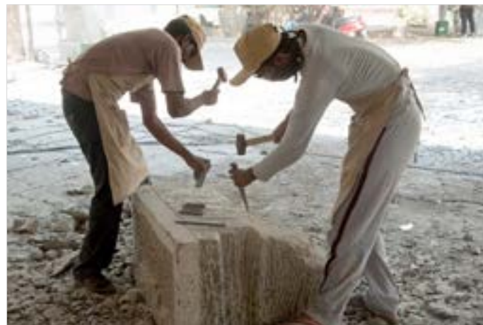
Sculptors roughing out the stone to get a basic shape.
