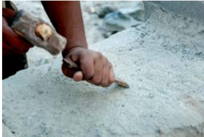
Flat chisel is used in flattening and leveling the surface of the stone.
