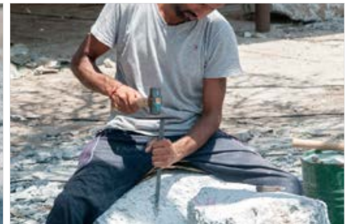
Striking the chisel to remove unwanted area.
