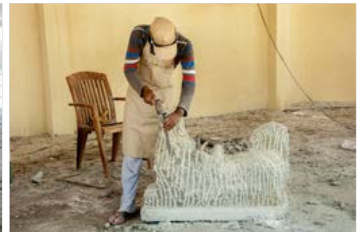
Stone is roughly carved using chisel and hammer.
