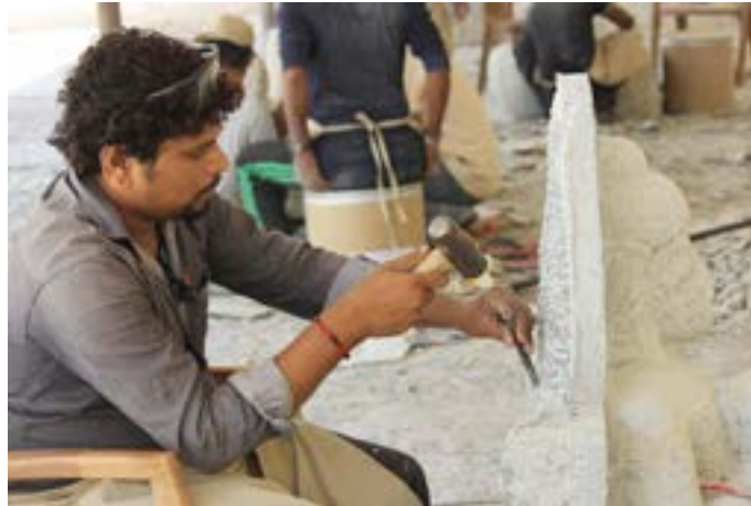
Sculptor is using point chisel to remove unwanted stone.
