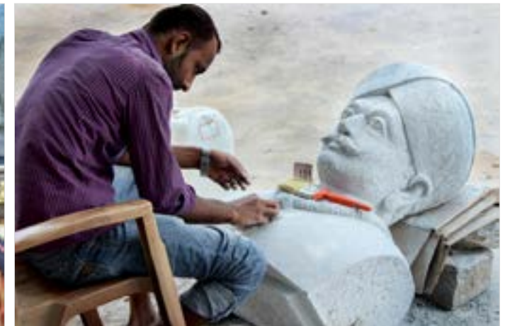
Emery paper is used to smoothen the surface.
