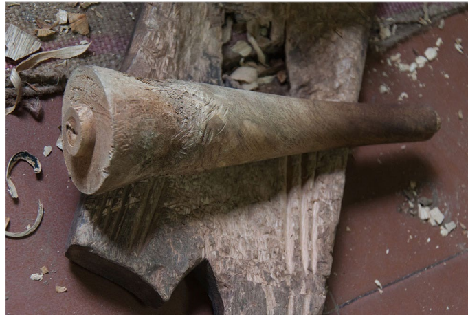
Cone-shaped wood is used as a hammer to carve the wood.
