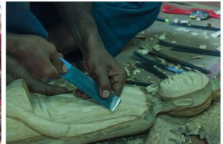
Finer details are carved using a flatter chisel.
