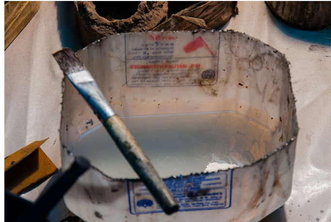
Melamyne Thinner is used for giving a glossy finish to the wood surface.
