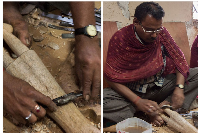
Using a wood scraper, wood is scraped off for smooth surfaces.
