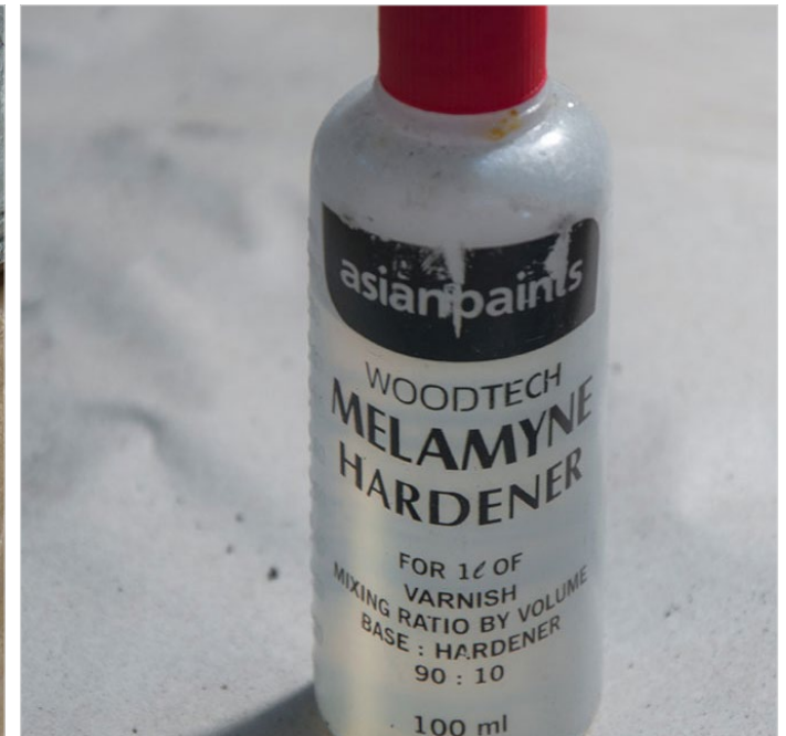
Melamyne Hardener is coated over the wood for better finishing.
