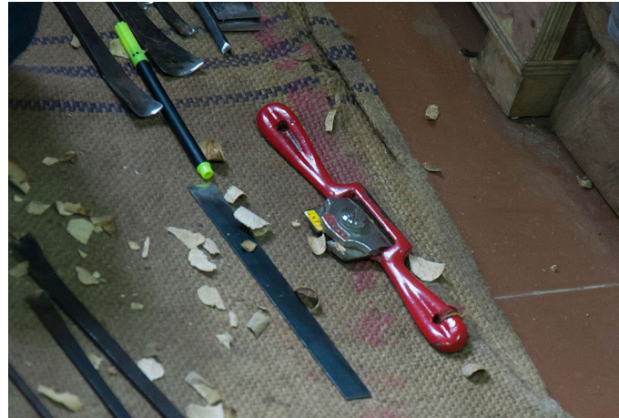
Wood scraper is used for scraping fine layers of the wood.
