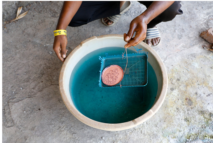
The plate is dipped into sulfuric solution.
