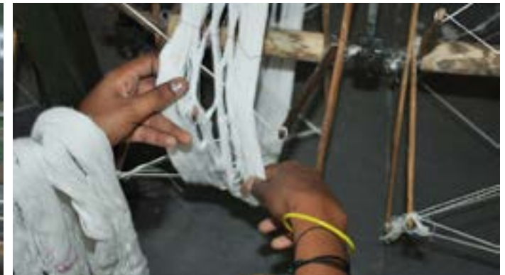
The bundle is placed and spread on the reeling wheel.
