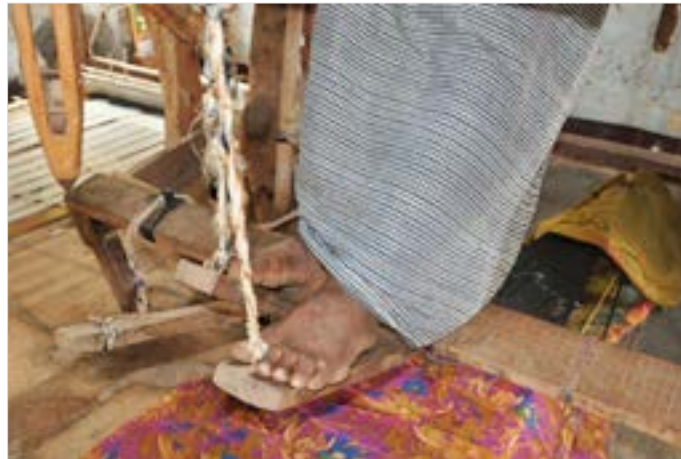
Pedal movement helps to handle warp allowing fly-shuttle to operate.
