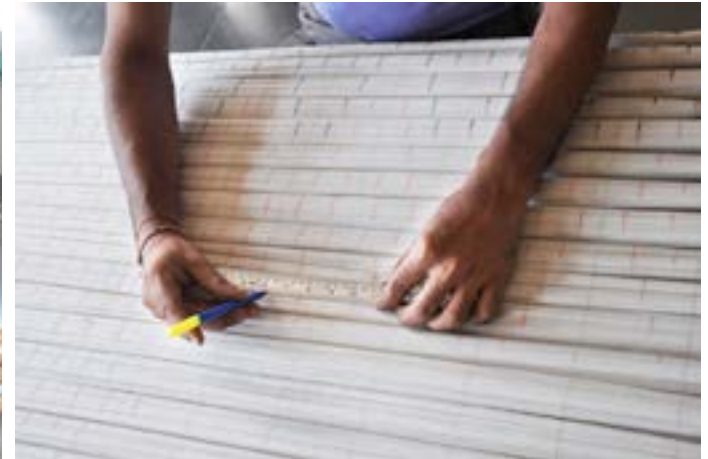
The design is marked on the warp threads with exact measurements.
