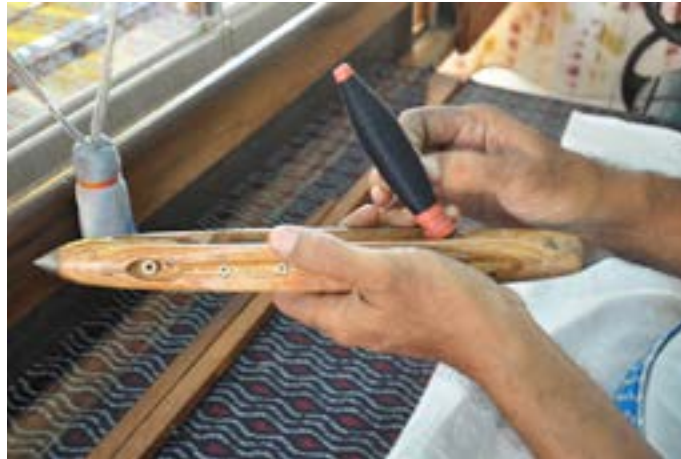
Spindle is inserted in the fly shuttle for weaving.
