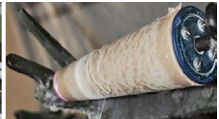
Thread is reeled on the cone.
