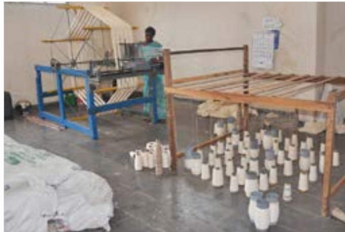
Spools are connected to warping wheel.
