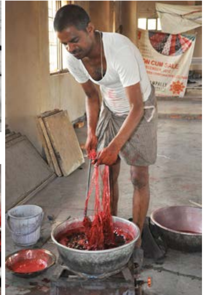
Initially, lighter colours are dyed and then darker colours are dyed on them.
