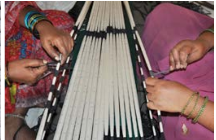
The design is tied with rubber strips.
