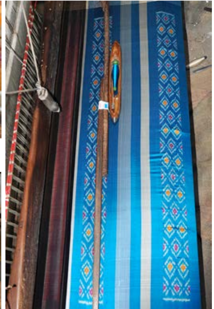
Finished sari is rolled on weavers beam.
