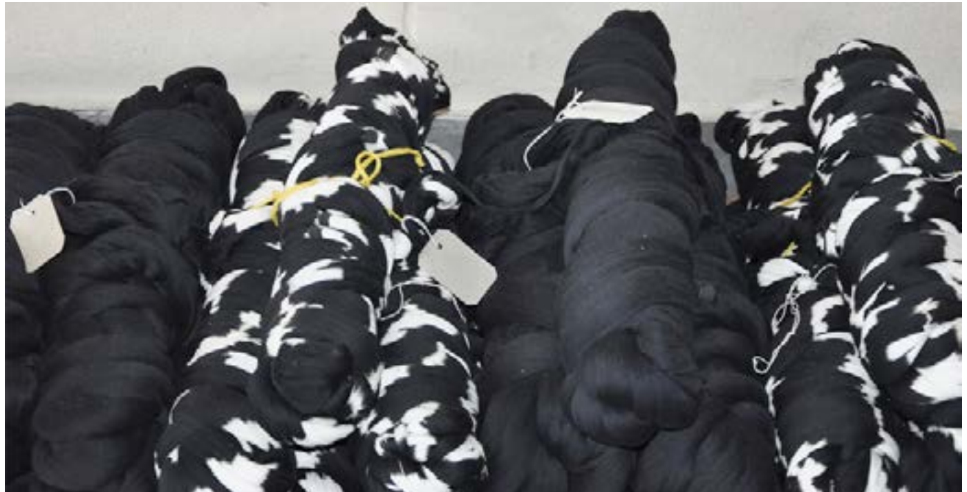
Warped threads are bundled and sent for jointing process.
