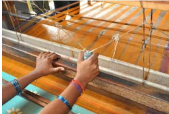
Pulley helps to operate fly-shuttle.
