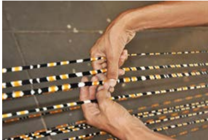
The warp threads are inspected for breakages and cleared.
