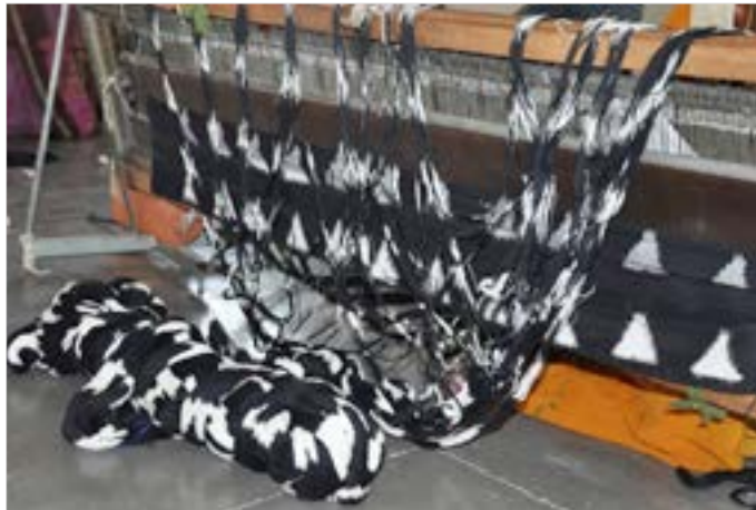
Warp thread are attached to reed.
