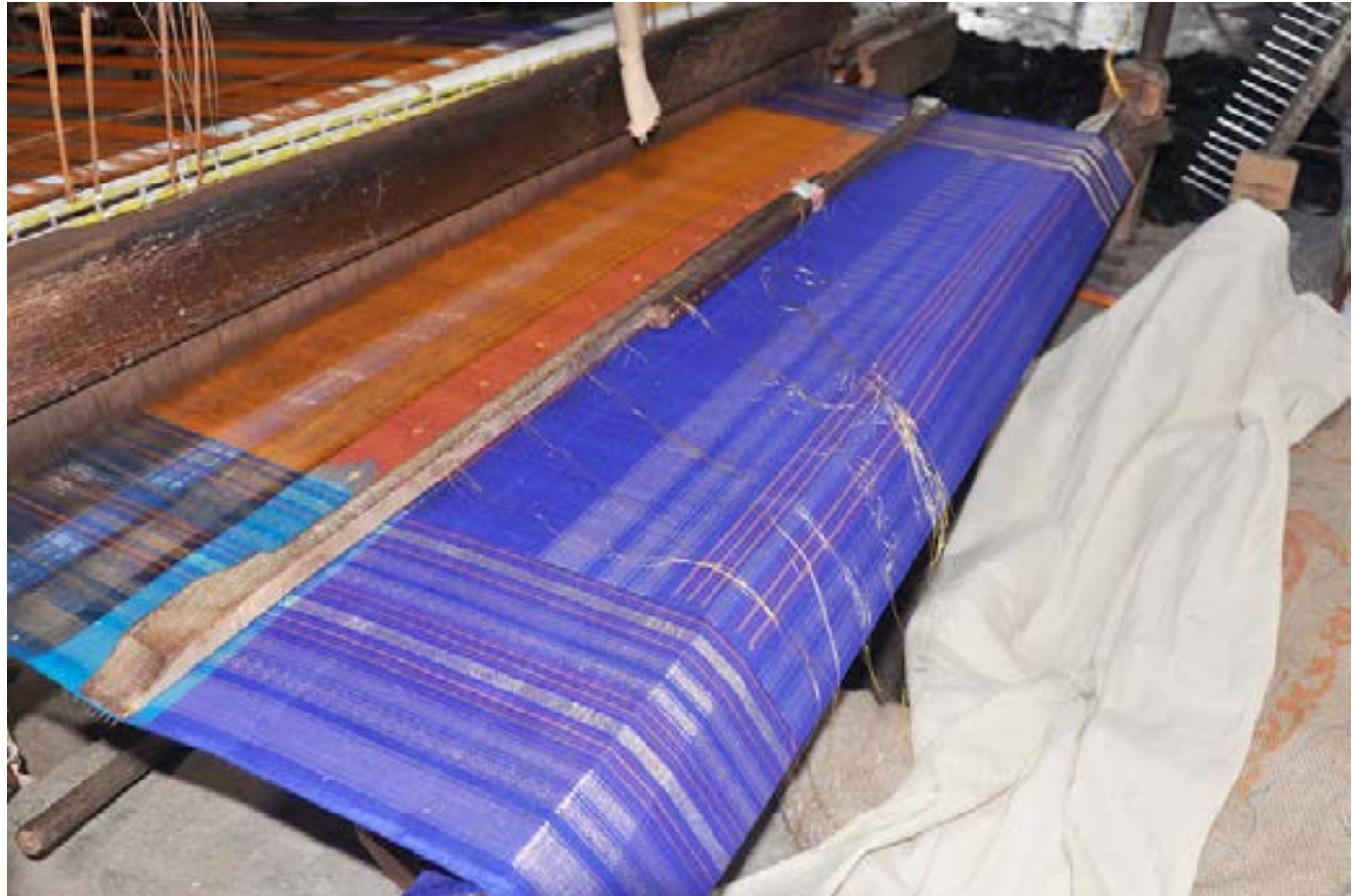
Zari threads are used to create motif designs.
