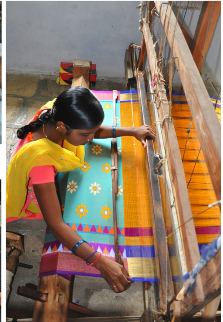
Different colours of motifs are obtained by adding external weft threads through spindles.
