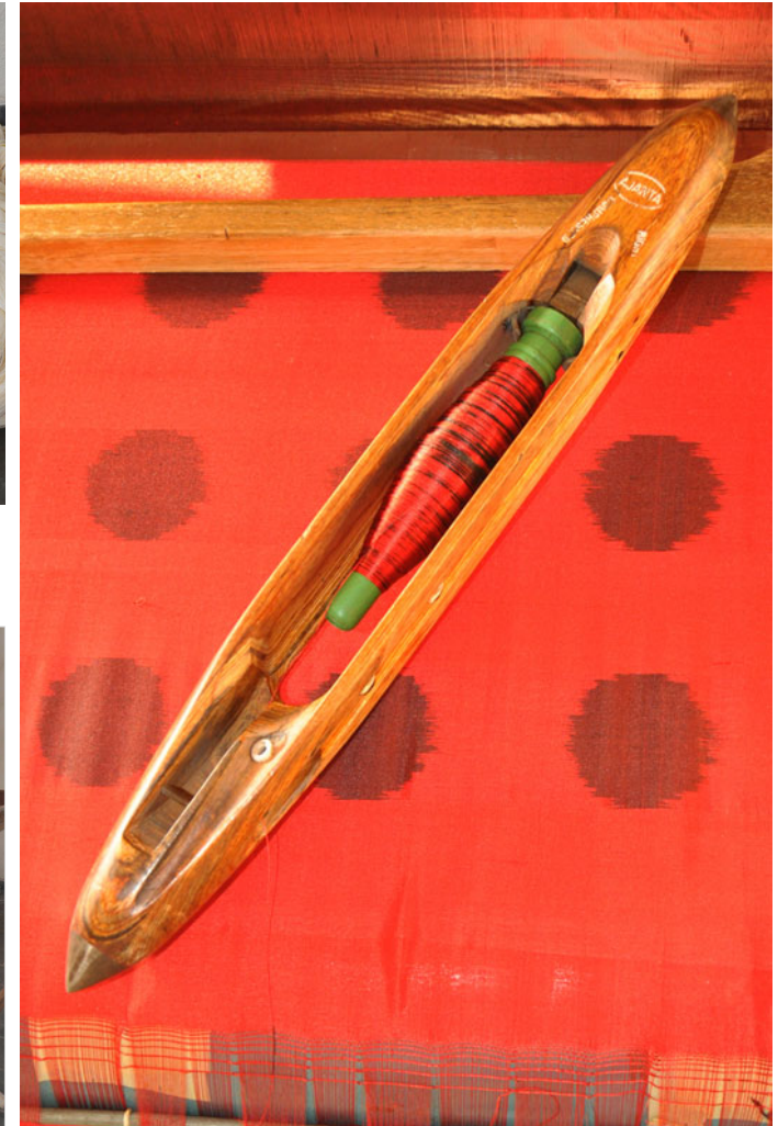
Spindles are inserted in fly shuttle while weaving.
