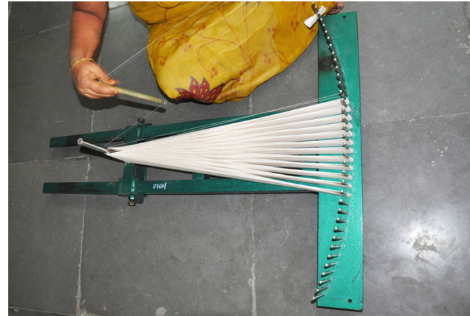
A different method of warping for smaller products like stoles and shawls.
