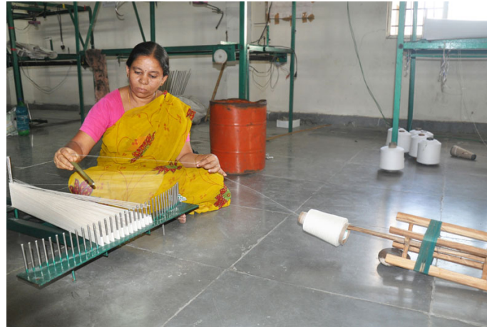
Cotton threads are spun to prepare warp.
