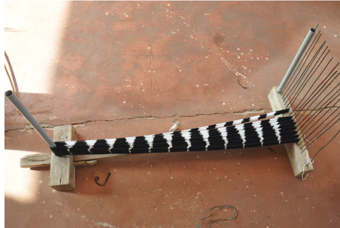
Cotton thread is reeled on smaller warping frame.
