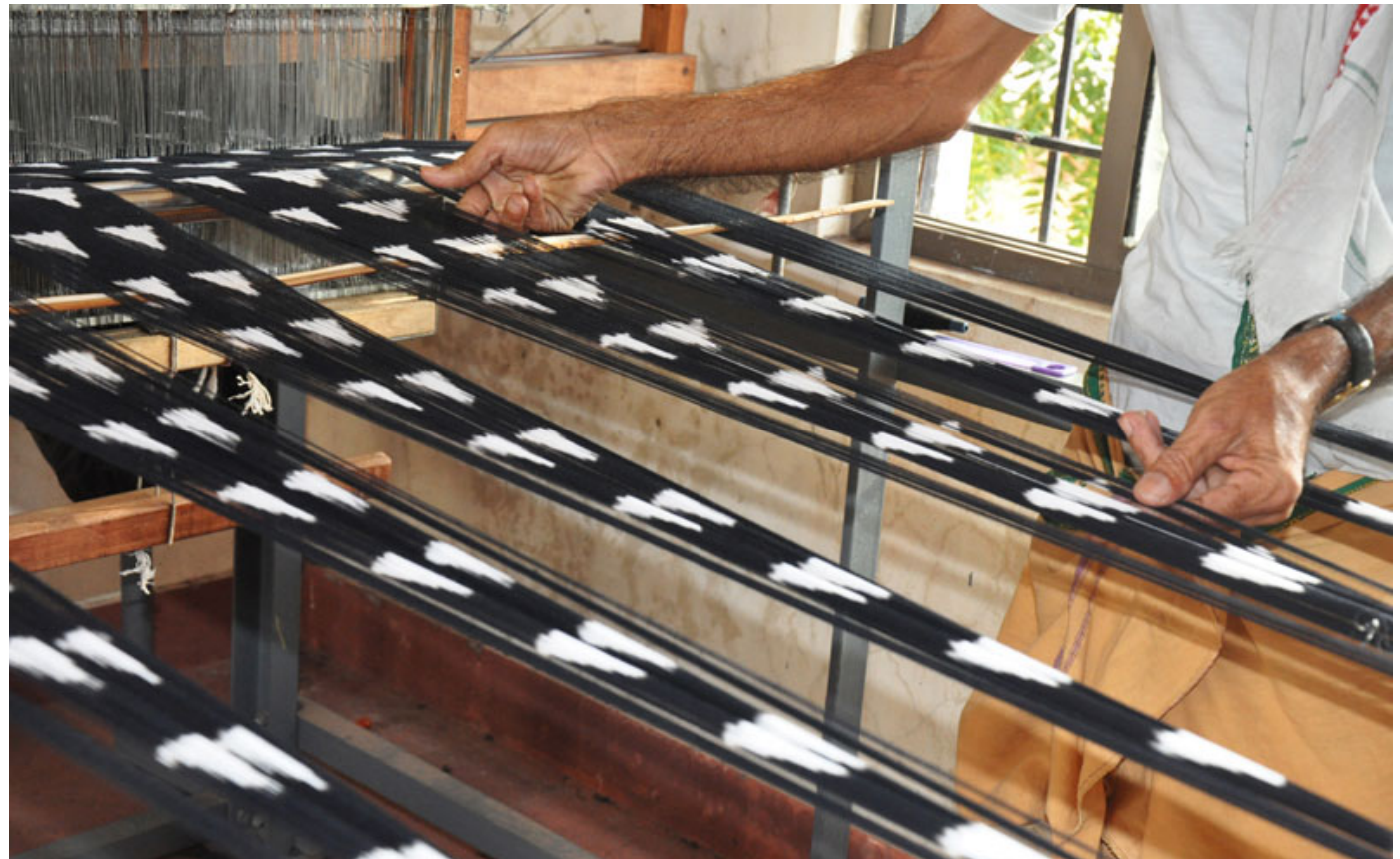
The prepared warp with reed is stretched and connected to loom.
