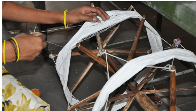
The end side of the thread is pulled out and connected to cone.
