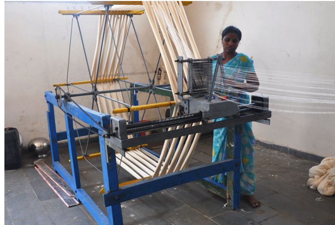
The warping wheel is rotated to prepare a minimum length 18 to 20 meters of yarn.
