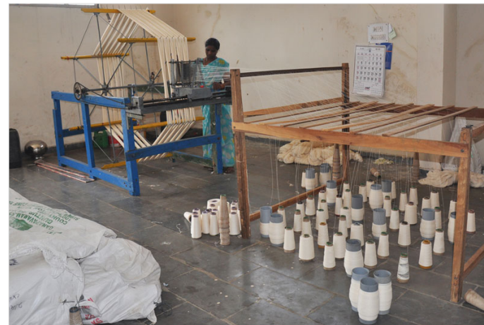
Spools are connected to warping wheel.
