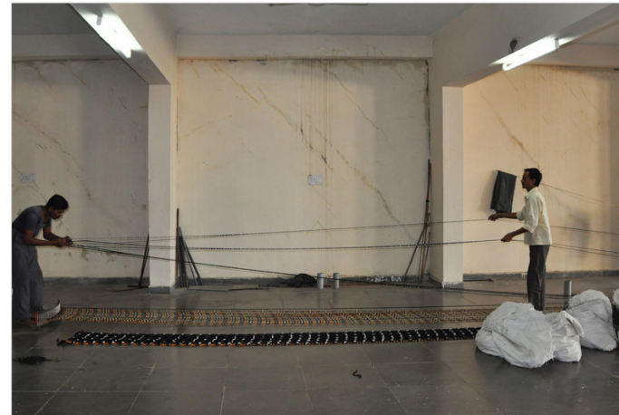
Dyed threads are again brought for another level of warping.
