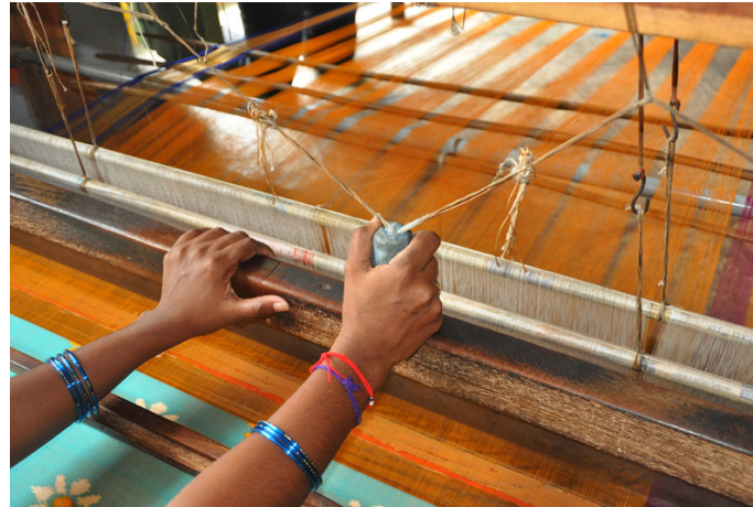
Pulley helps to operate fly-shuttle.
