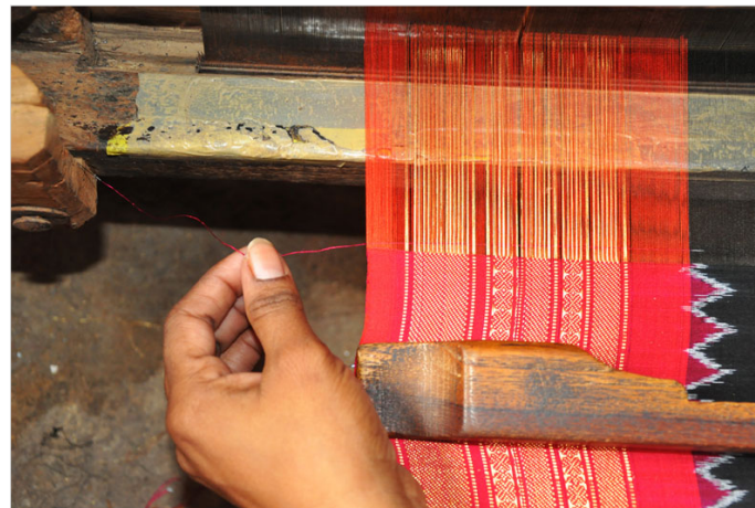
After every single weave, the strand is pulled on sides to tighten the weave.
