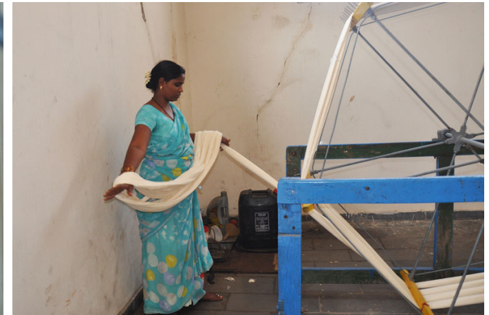
Prepared warp is sent for tie and dye process.
