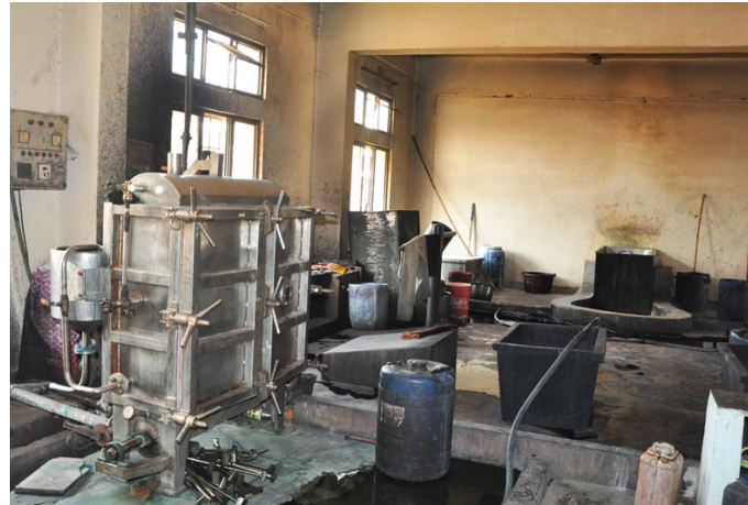
Automated dyeing machine to dye silk and cotton threads in large quantity.
