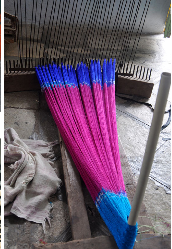
Warp is dyed in vibrant colours.
