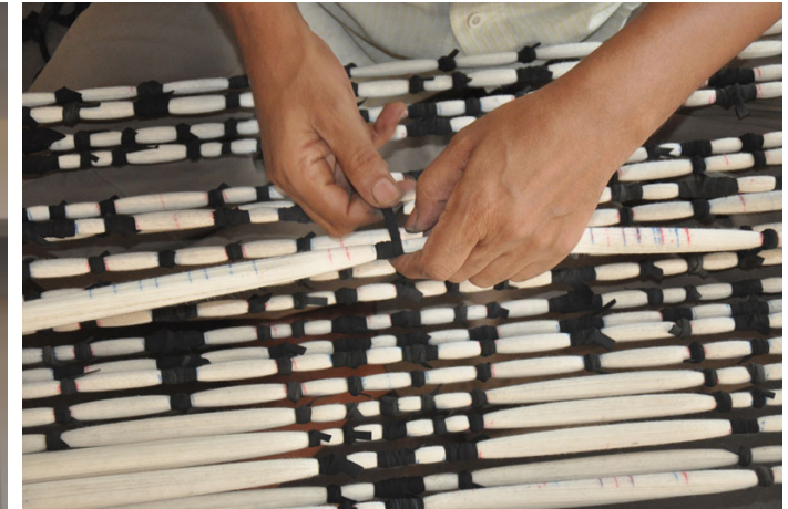
Rubber strips are used because it holds the threads tightly.
