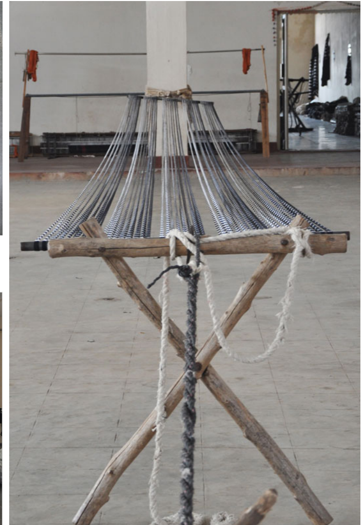
Warp is stretched and tied between two poles.
