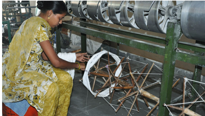
Placing the yarn bundle on the reeling machine.
