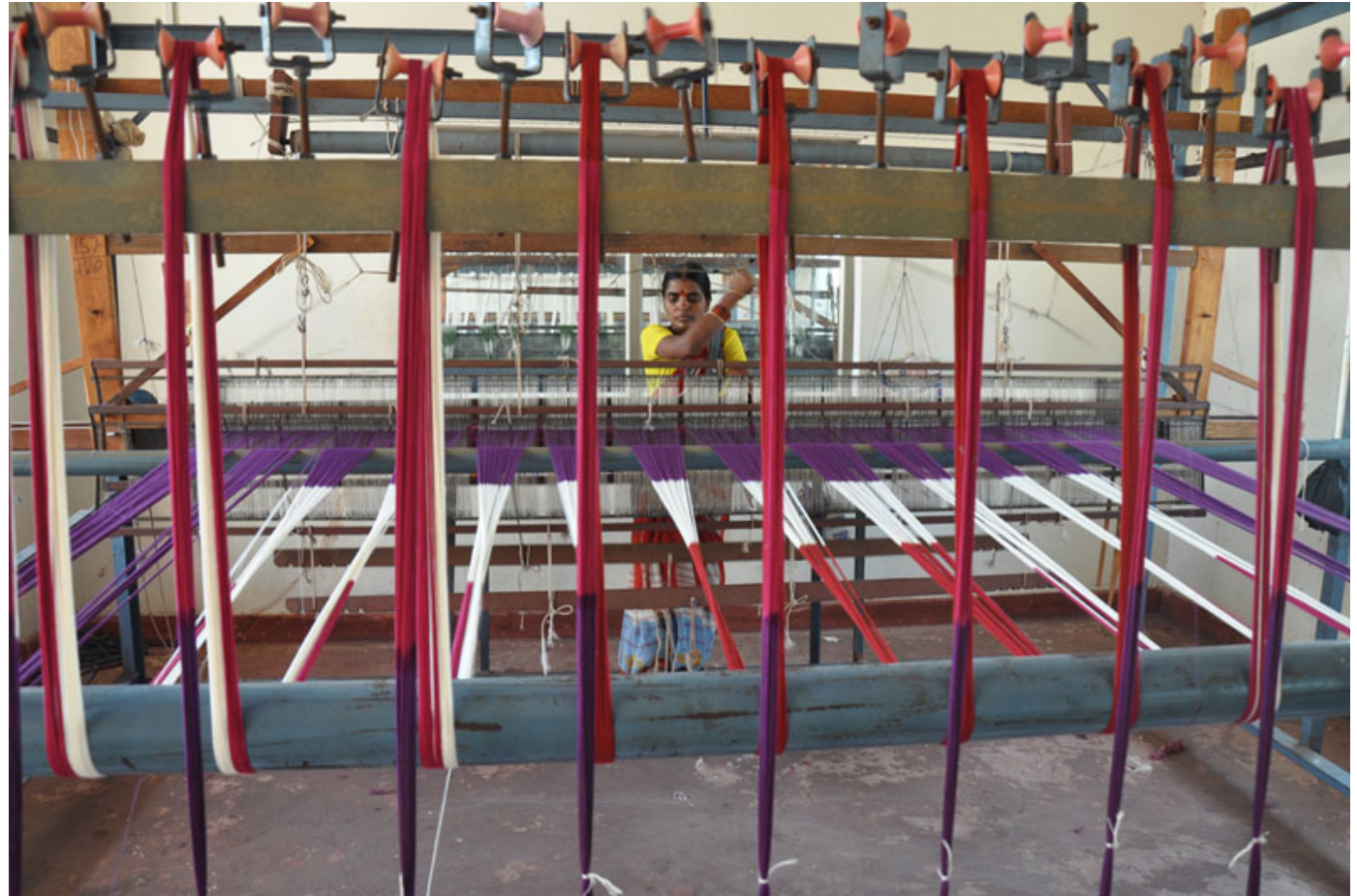
The bigger loom in handloom factory is setup to weave wider products.
