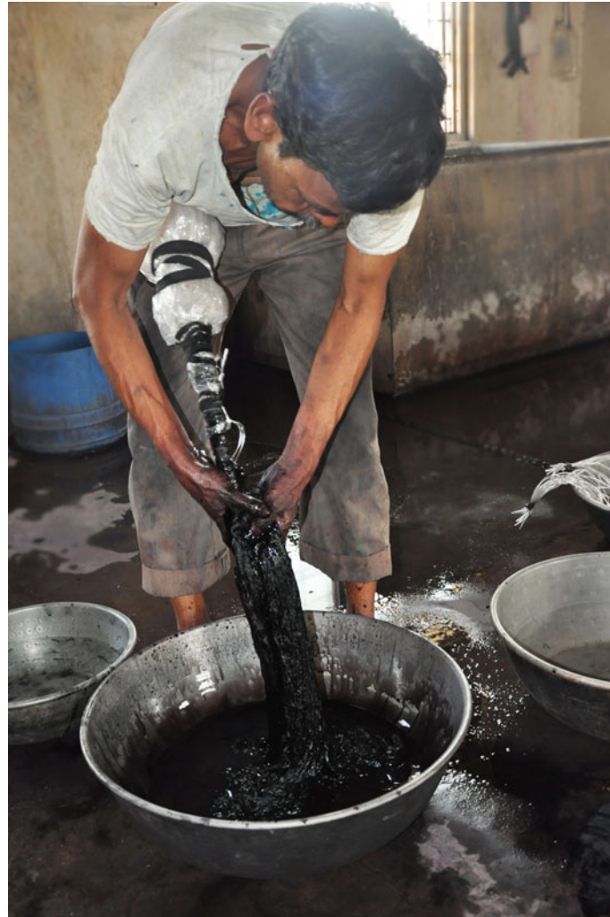
The previously tied area is removed and exposed to dye in another colour.
