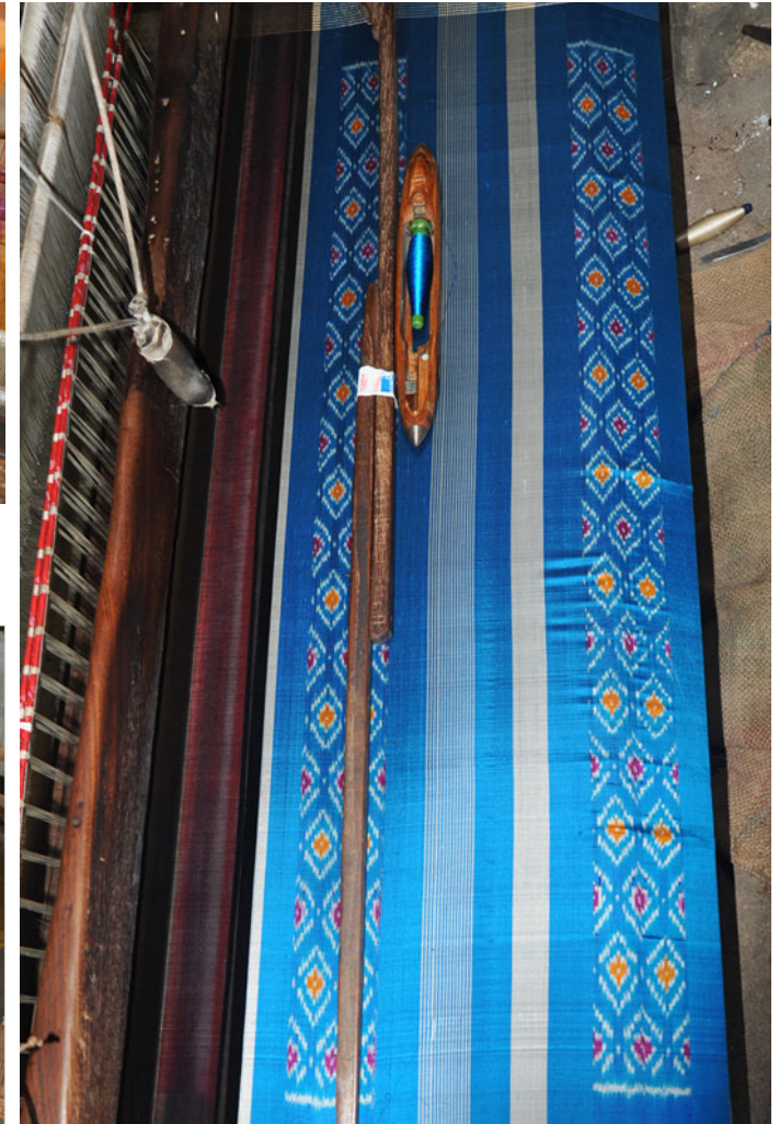
Finished sari is rolled on weavers beam.
