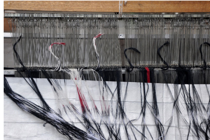
Threads are connected and reed is loaded into weaving loom.
