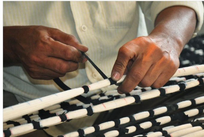
The marked design on the warp is tied using rubber tubes.
