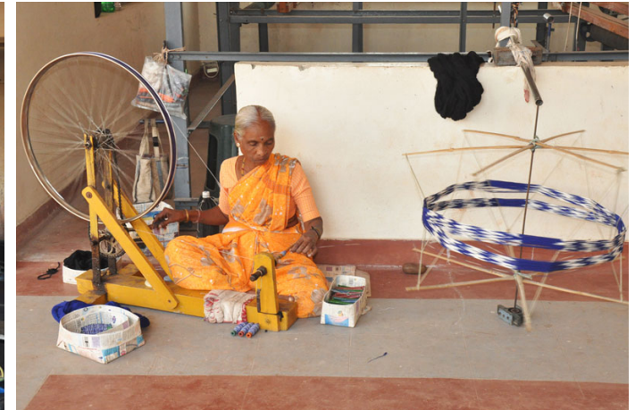
Traditional method of spinning to make spindles.
