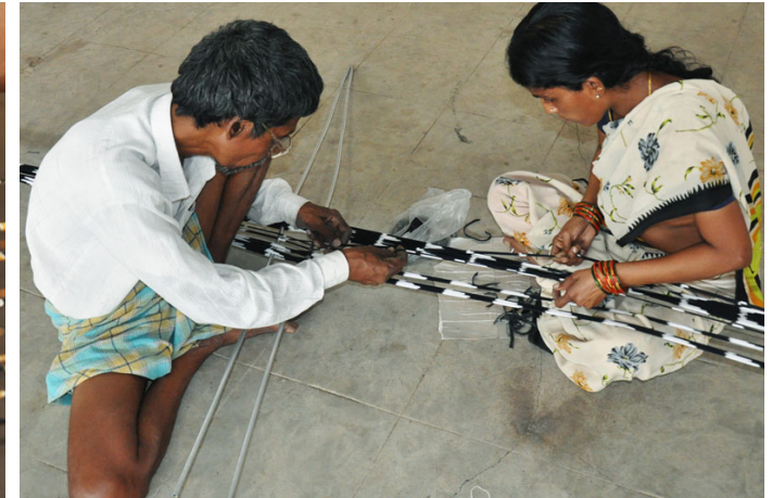
Warp threads are aligned as per the design.
