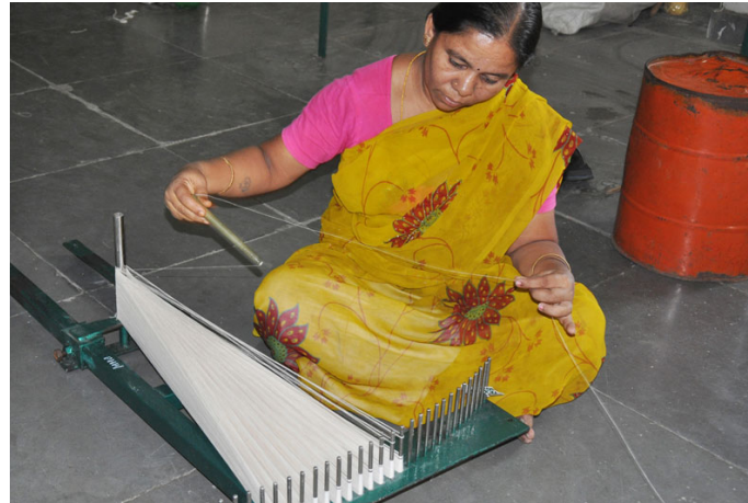
Yarn is wrapped manually in a “to and fro” movement using warping frame Aasu.
