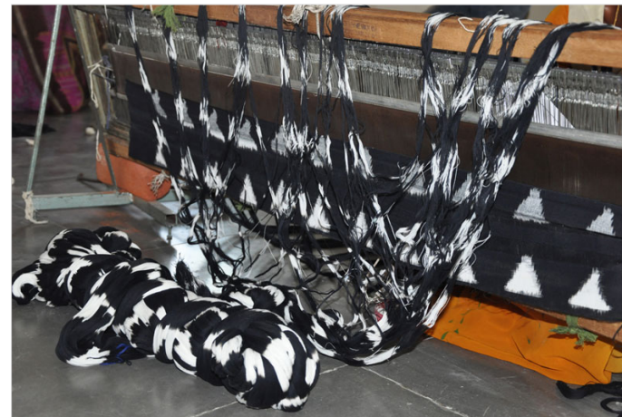
Warp thread are attached to reed.
