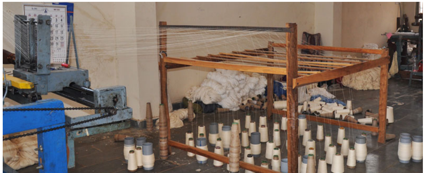
Threads from multiple spools are taken and connected to the warping wheel.
