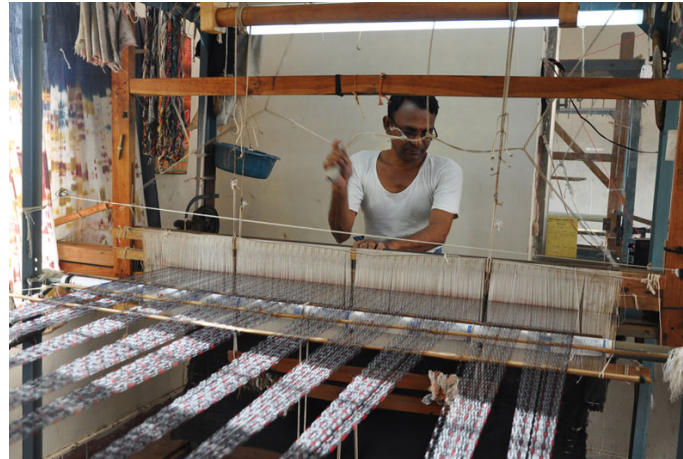
Stretched warp is tightly pulled and connected to weavers beam.
