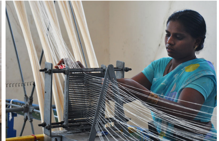
Broken threads are joined together and continued reeling.
