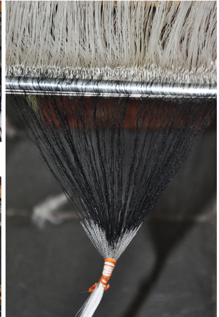
After tying, the amount threads are tied with cotton thread to avoid breakages.
