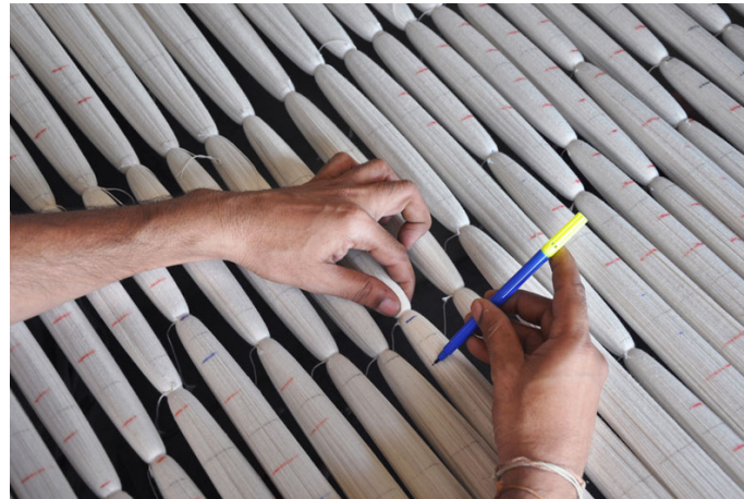
Once the design is marked, it is first tied with cotton thread.
