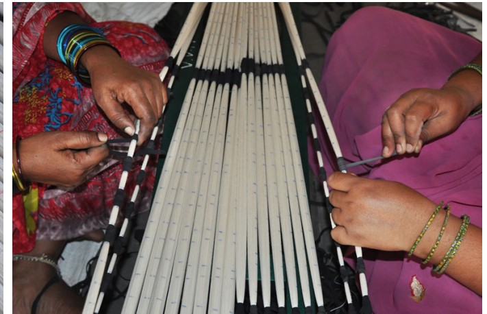
The design is tied with rubber strips.
