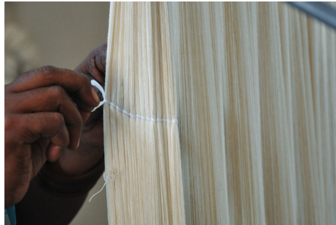
Cotton thread is laced to divide the warp in segments.
