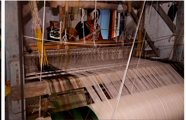
The warp threads being loaded into the loom for the weaving process.
