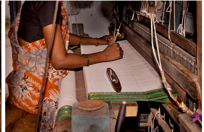
Once the fly shuttle is passed through the warp, the beater is pulled by the artisan to join threads.
