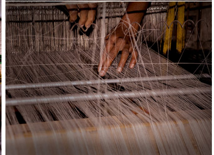
In case of any broken thread, while weaving, they are joined on the spot with hands and the process is resumed back.
