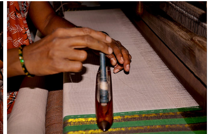
A spool wrapped with threads set inside a fly shuttle.
