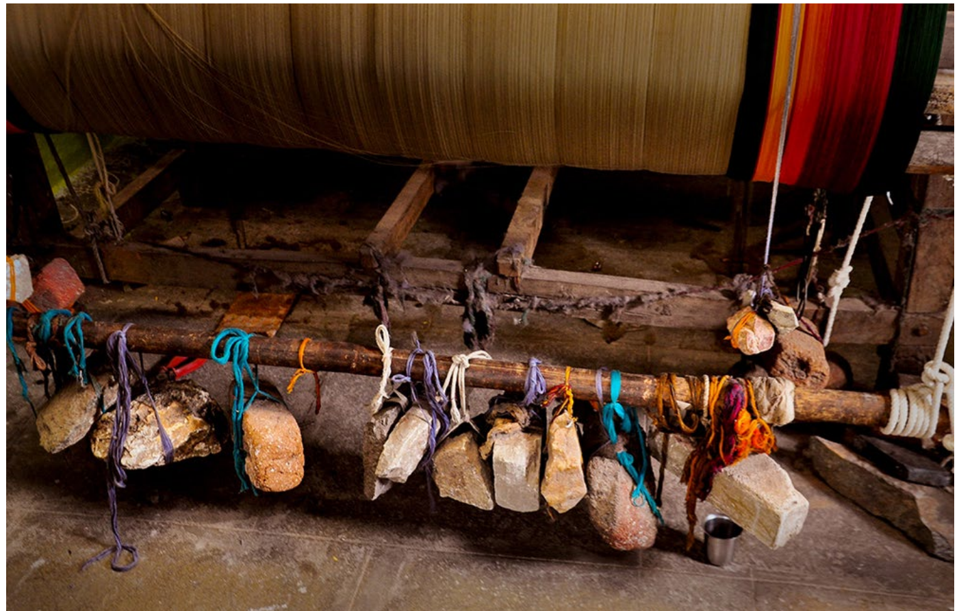
The stone used as a weight to keep a side of the weaving machine tight and intact.
