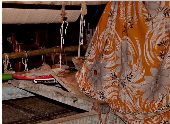
Pedaling helps in opening and closing warp shed to facilitate weaving.
