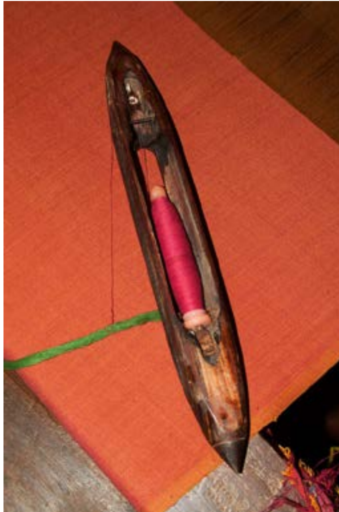
Fly-shuttle loaded with spindle.
