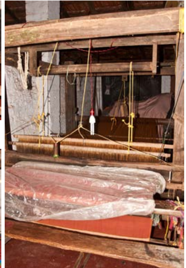
When the loom is not functional it is covered with polythene sheets to save the woven portion from dirt, dust, water and flies.
