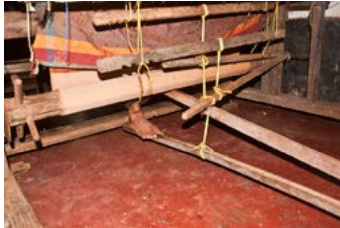
Pedaling helps in opening and closing of warp shed (two sets of healds bar) to facilitate weaving.
