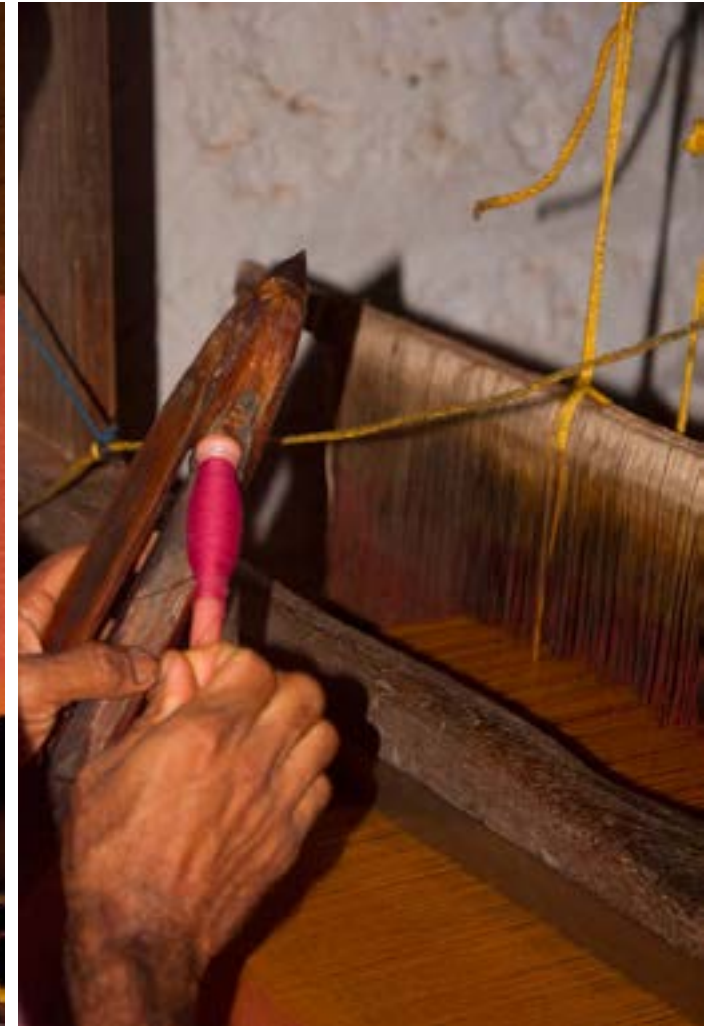
Weaver inserting the spindle / spool to the fly shuttle, before putting to the fly bar.
