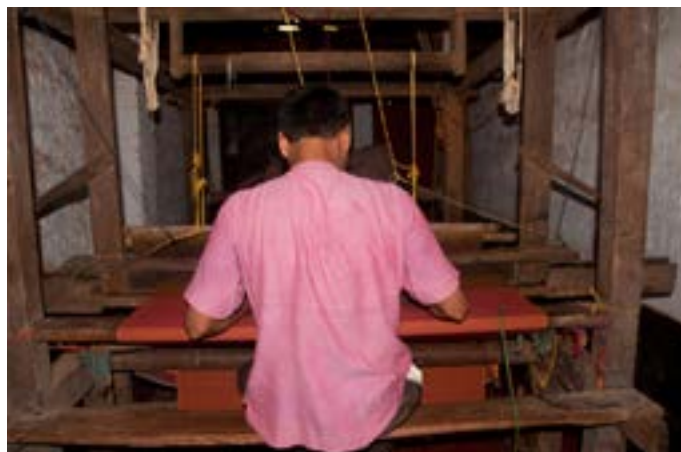
Basic floor loom made of wooden frames and bamboo poles. Weaver is busy in mending some broken warp thread.
