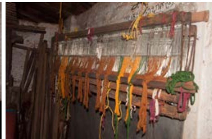
The warp is prepared and threads are passed through the healds. These threads are then connected to the take up beam.
