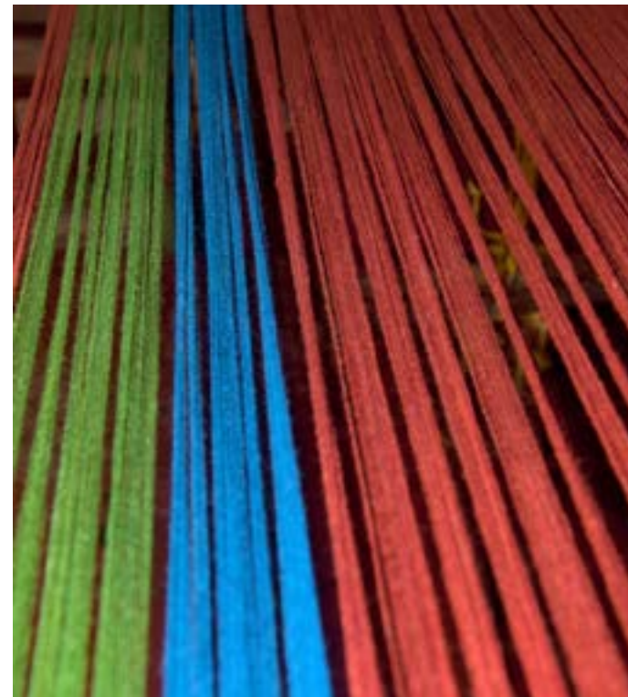
The warp with multi-coloured border threads. (Probably 2/40's, 2/60's, and 2/80's non mercerized cotton)
