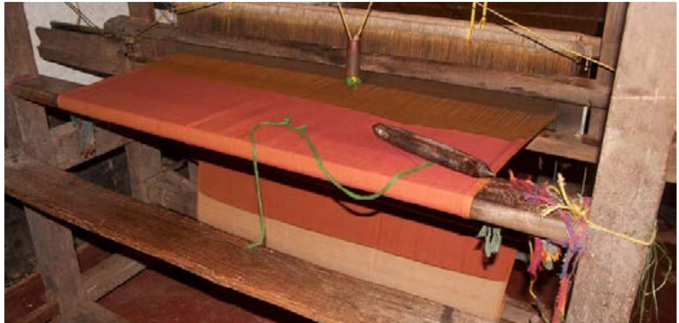
Woven sari is wound on a take-up beam. The flat wooden plank is the seat for the weaver. The fly shuttle can be seen on the loom.
