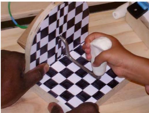
Figure.8 Racecar Pronation/Supination Test
