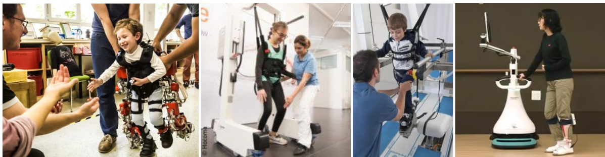
Figure 1. Robots for physiological assistance and guidance during walking rehabilitation <from the left: power suit ([Kid exoskeleton], 2016), mobile gait ([Andago], 2019), "end-effector robot" ([G-EO System], 2021, and walking guiding robot ([TREE], 2017)>
