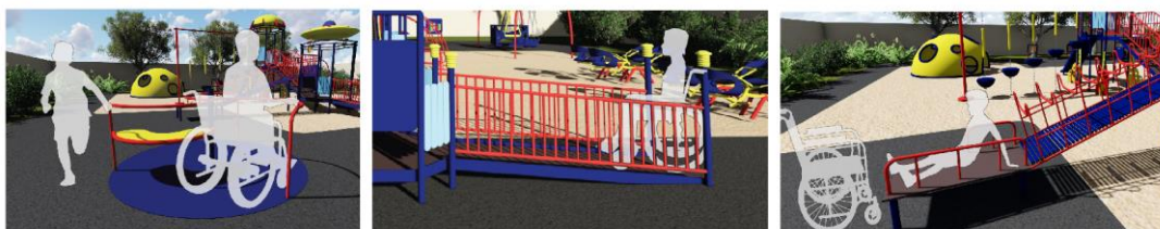
Figure 7. Provision of ramps, transfer platform and leveling of equipments
