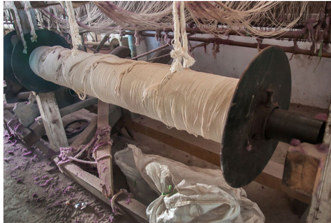
The yarn wound on the warping wheel is reeled over the iron rod for the warping process.
