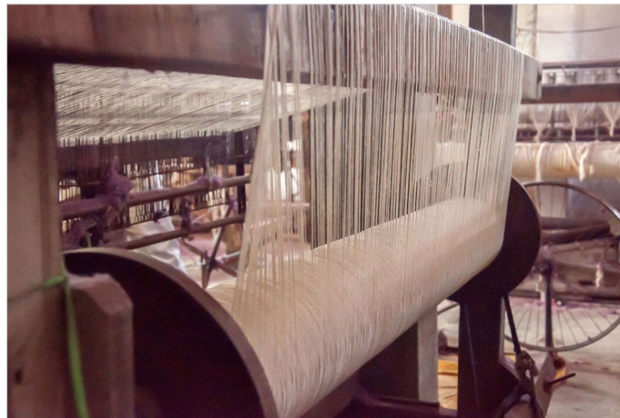
Yarn winded on the iron rod is fixed to handloom and threads are fixed.
