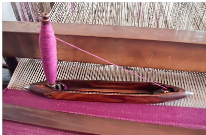
A flying shuttle is used for the wafting process of fabric.
