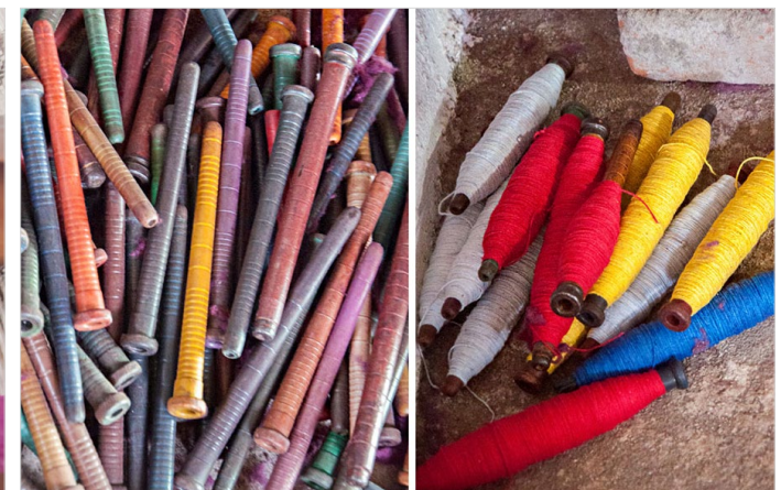
Spindles are wound with yarns, which are loaded in a flying shuttle.
