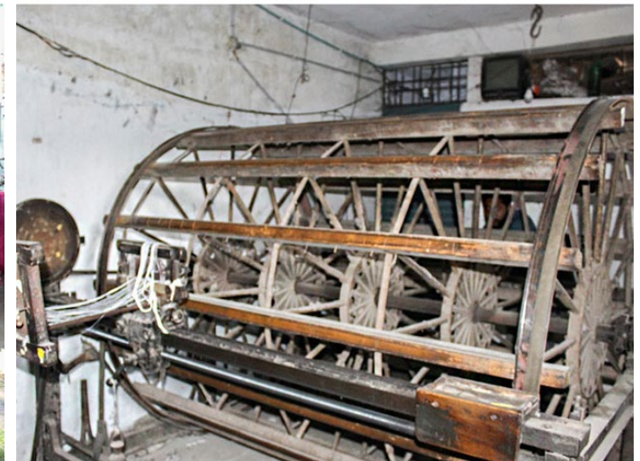
Threads being extracted from various spindles and wound on the warping wheel.
