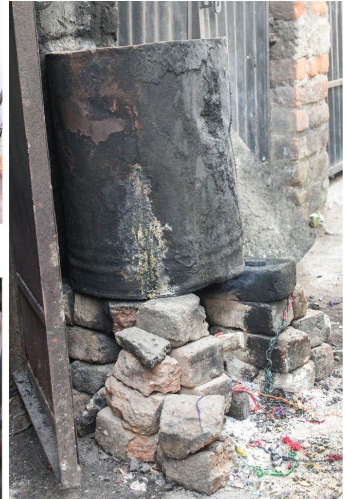
The dye is heated in a drum on a customized stove.
