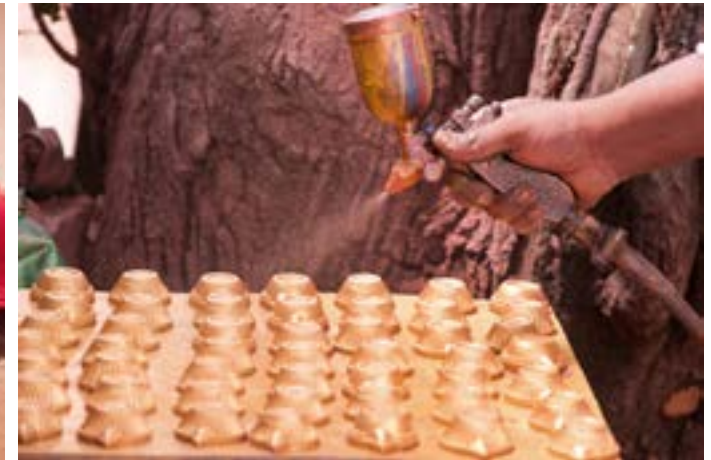
With the help of a spray machine artisan spraying colour on one side that is back side of diya.
