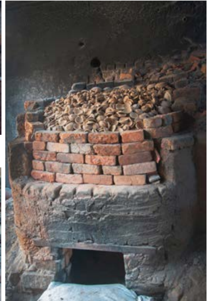
Waste plywood pieces are used for the burning process. All diyas are arranged properly inside the kiln.
