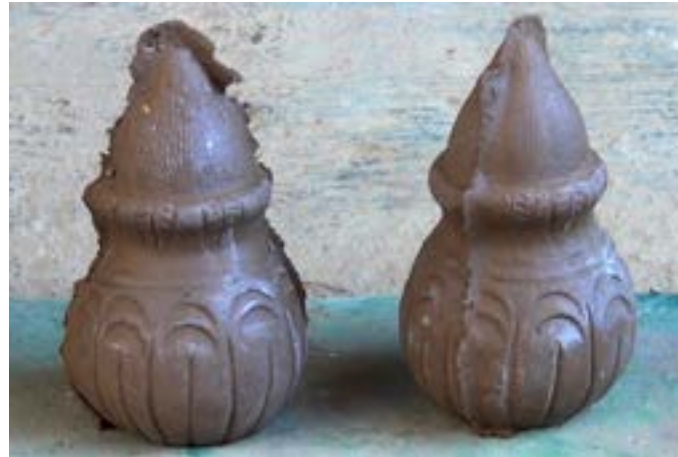
The final product is ready after removing both half of the mould.
