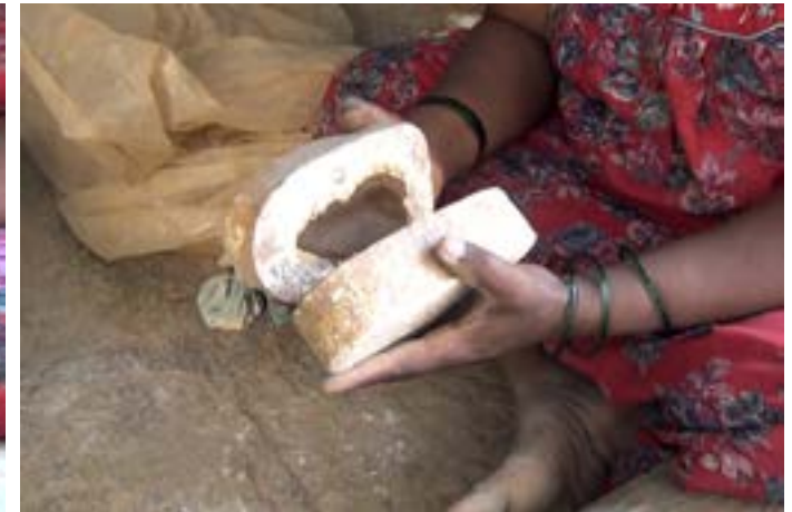
Clay is filed with little pressure to reach the cavities.
