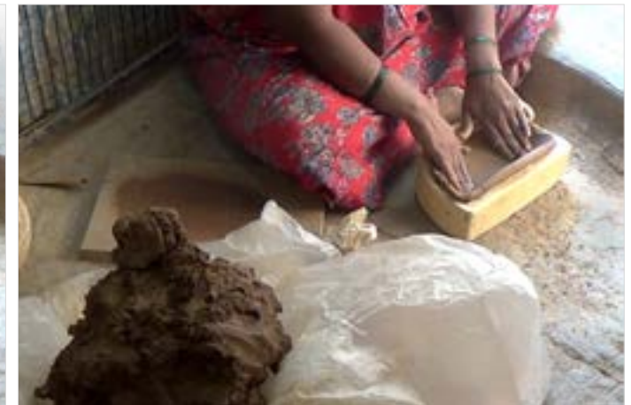
The clay slab is placed on the mould and pressed until it gets the shape of the mould.
