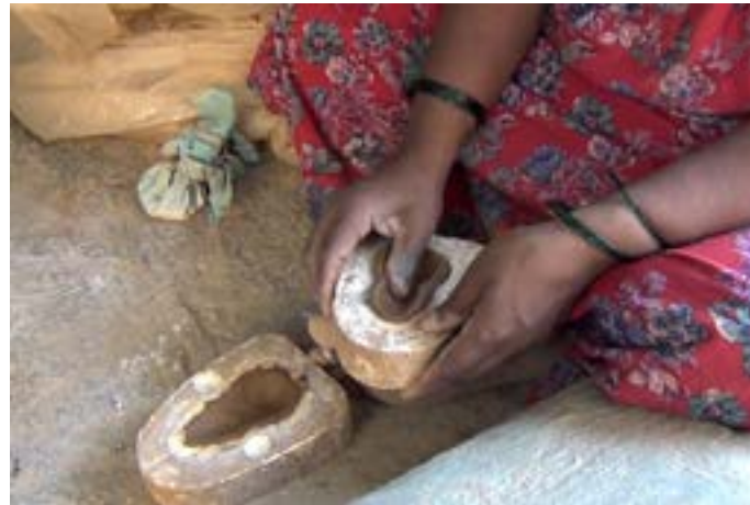
Artisan filing clay both half of the mould.
