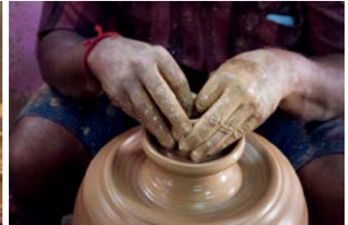
Artisan pulling out the clay to make the structure for diya.
