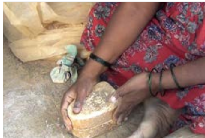
Both half of the mould is pressed for 15 seconds to get a proper shape.
