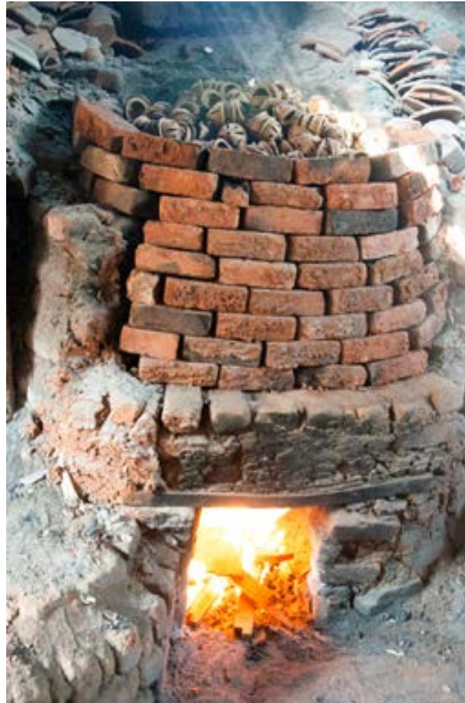
Burning process- 600 to 700 degrees temperature is maintained for 6 hours.
