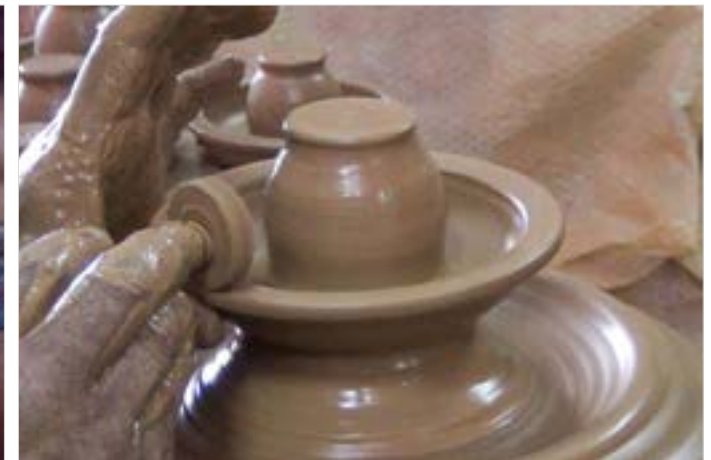
Creating design on the lamp with customized tool.
