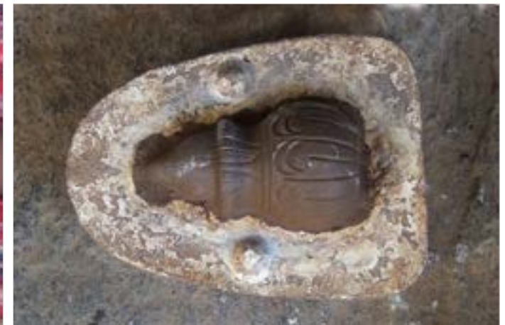
Both half of the mould is pressed for 15 seconds to get a proper shape.
