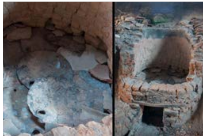
Iron plates are arranged on iron rods.
