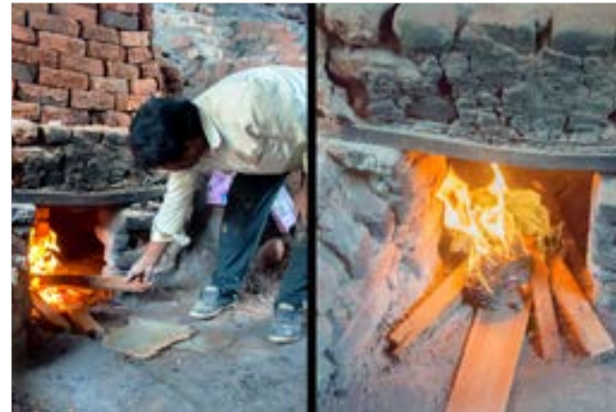
Waste plywood pieces are used for the burning process. All diyas are arranged properly inside the kiln.
