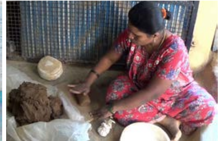
The clay is kneaded to make the wet slab.
