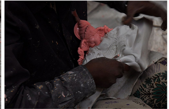
The rubber mold is removed, and the fiber statue is taken out.
