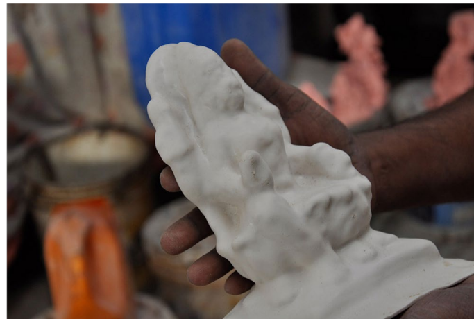
A rubber mold is used to cast the fiber statue.
