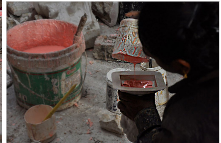
The fiber mixture is poured into the rubber mold.
