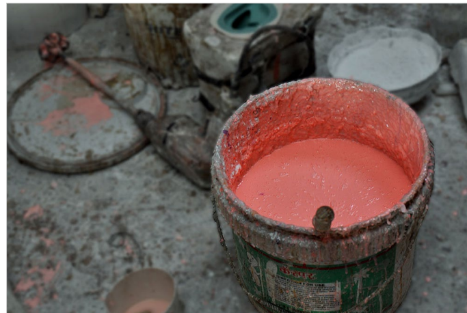
A mixture of chalk powder and resin, to make the fiber statue.
