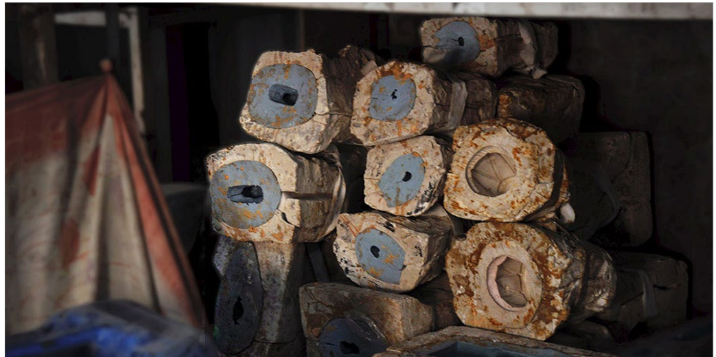
Plaster of Paris mold used to hold the fiber mixture while drying.
