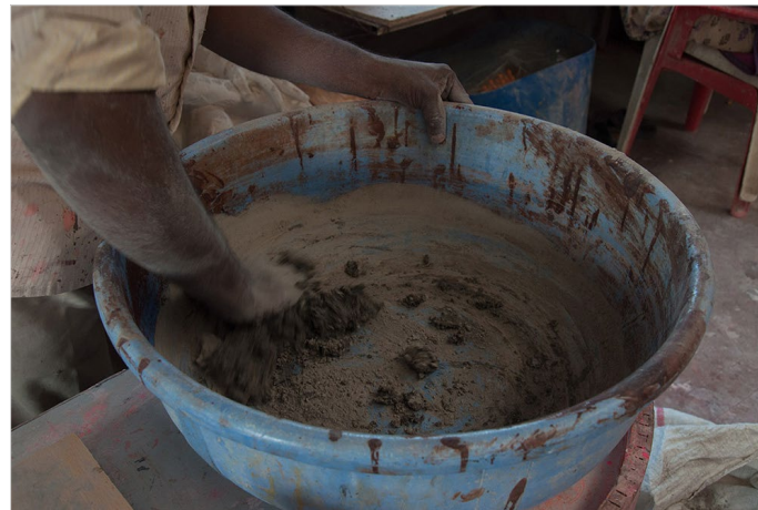
Clay powder and water being mixed until the right consistency is attained.
