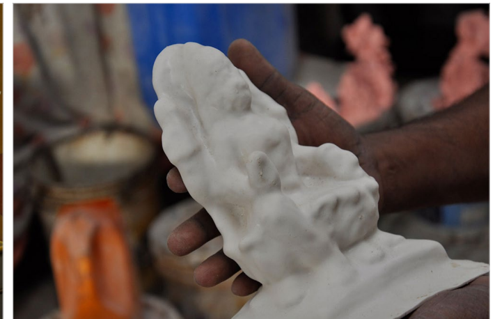
Liquid rubber poured on the clay model to take the impression.
