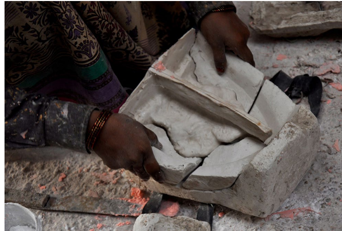
After the mixture dries, the plaster of paris is removed.
