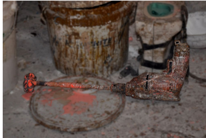
Peddle mixer, used for efficient and fast mixing.
