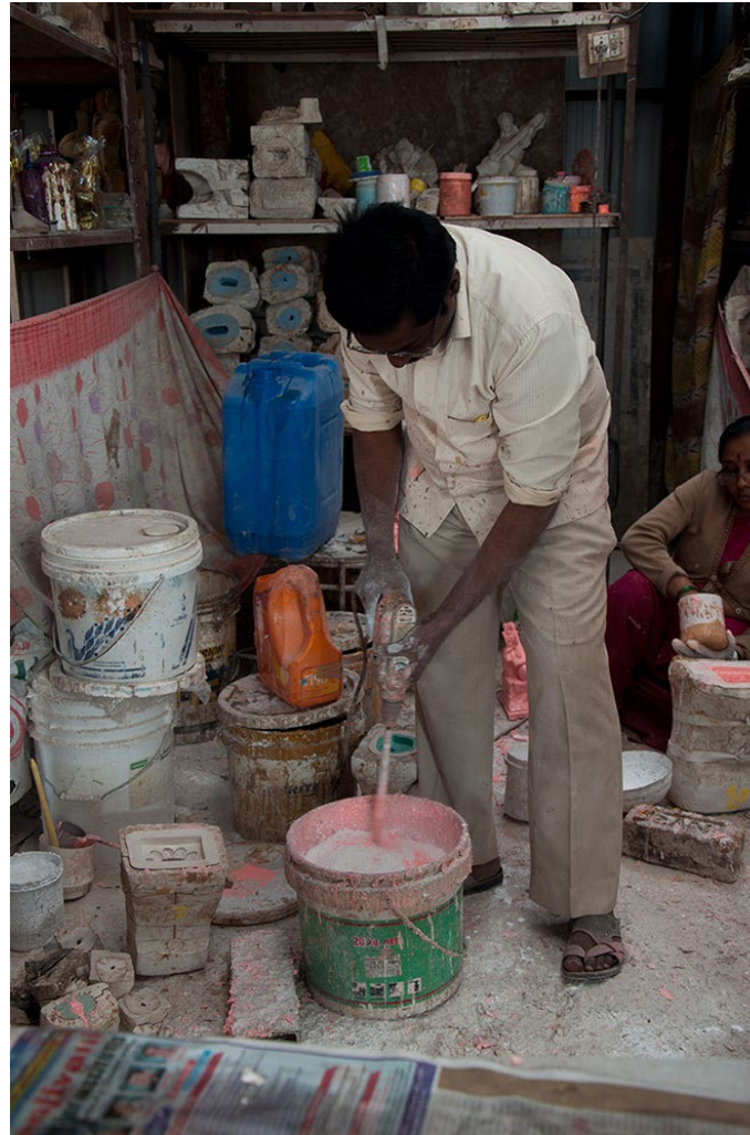
Chalk powder and resin mixed by a pedal mixer.
