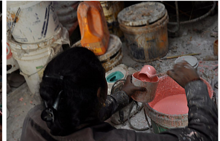
The mixture was added with a small quantity of hardener being poured into a smaller container.
