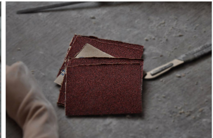
The sandpaper is used to smoothen the rough surface and remove excess pieces in the statue.
