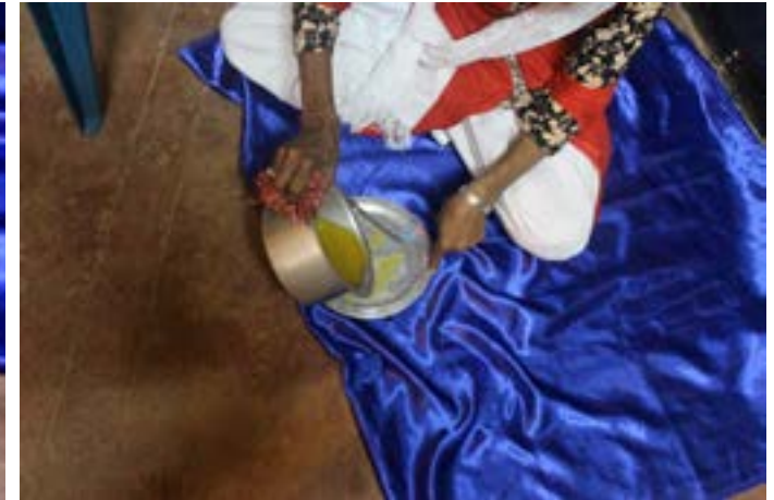
Dyed wax is poured in the plate and allowed to cool for 5 to 8 minutes.
