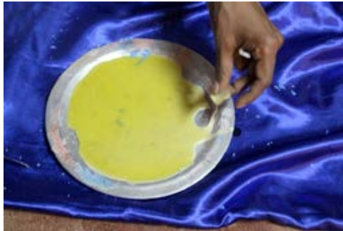
Wax is allowed to cool down until the required consistency is obtained, which eases the process of molding.
