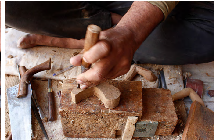
A small hole is made on arm for fixing purpose.
