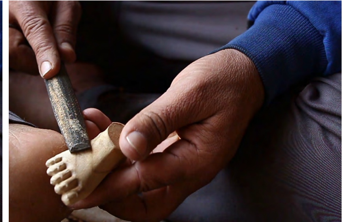
Front side of the foot is smoothened using a file.
