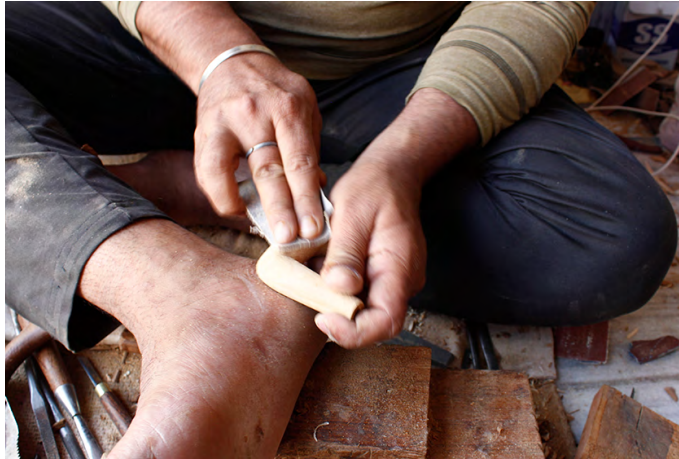
After attaining proper arm shape, it is smoothened using sandpaper.
