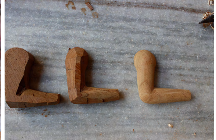
Different stages of arm making process.
