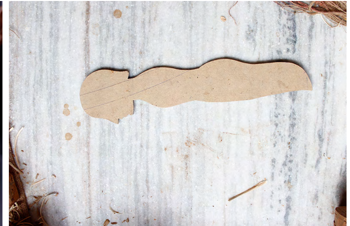
Stencil is used to mark the basic shape of an idol.
