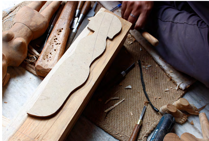
Wooden block is marked using a template.
