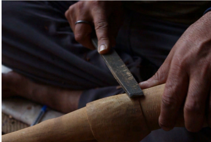
Flat filing is used for smoothing.
