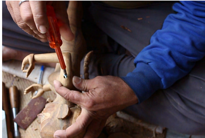
Hand is fixed to body using nail and screwdriver.
