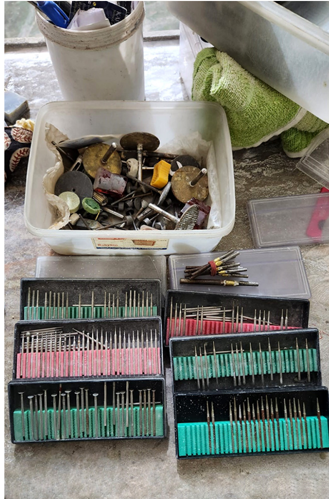
Diamond tools used for stone carving.
