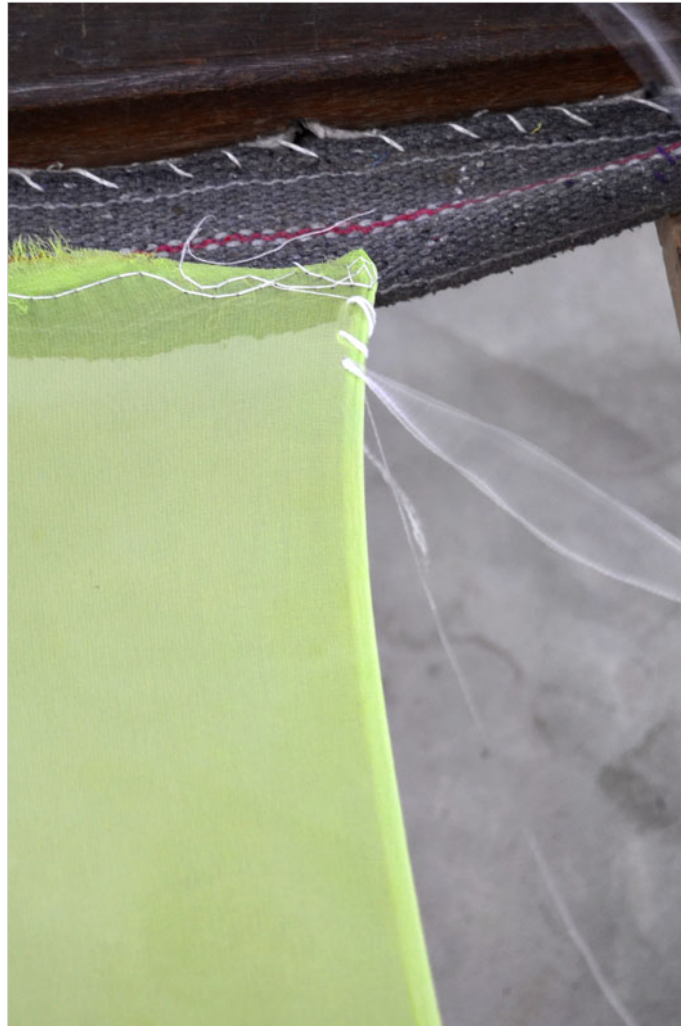
Fabric being tied to two sides of a wooden frame (known as 'khaat') using thick cords.
