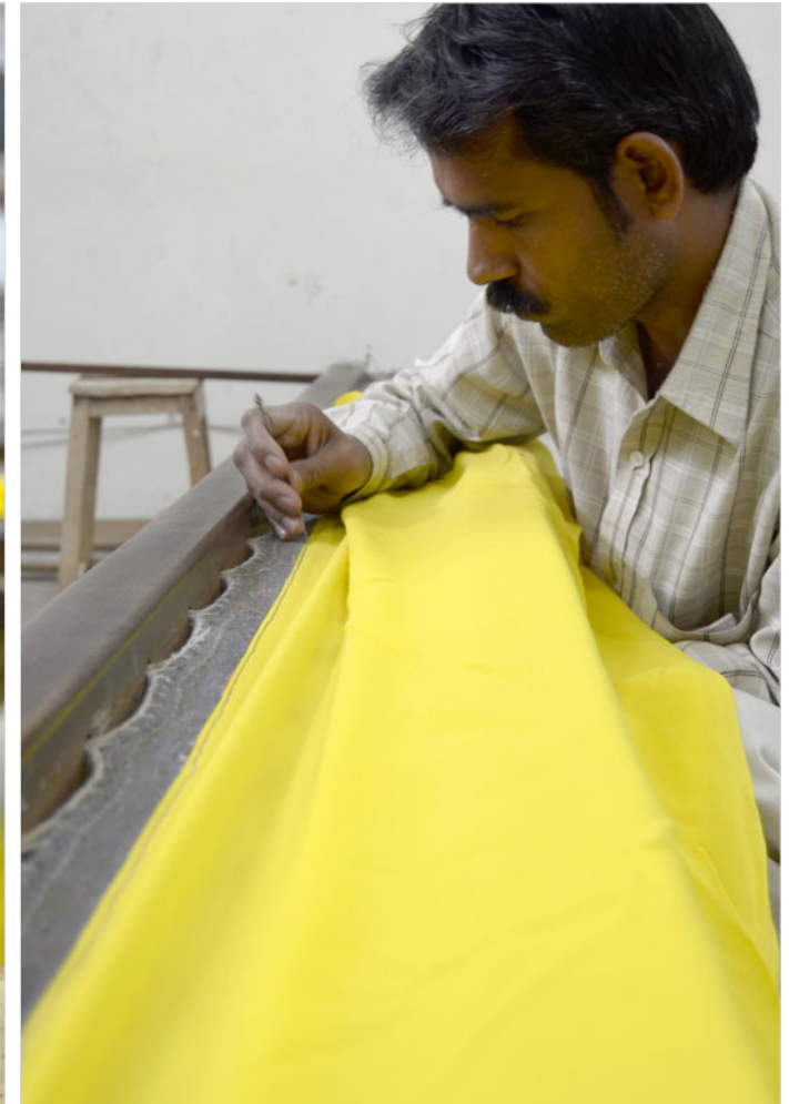
Fabric being tied to two sides of a wooden frame (known as 'khaat') using thick cords.
