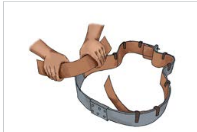
Plywood being fixed into the mold.
