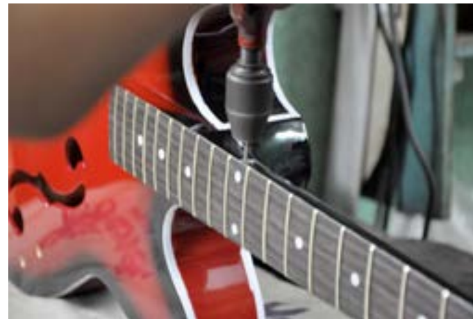
Holes made as a reference mark on the neck.
