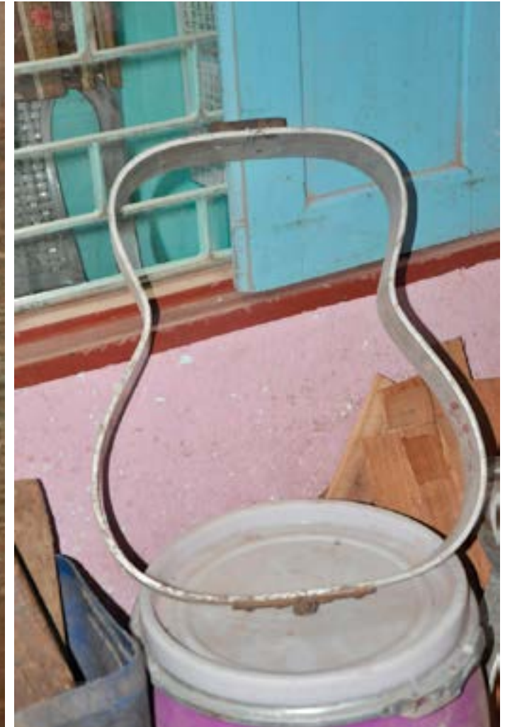
The mold is used to create the base body for the guitar.
