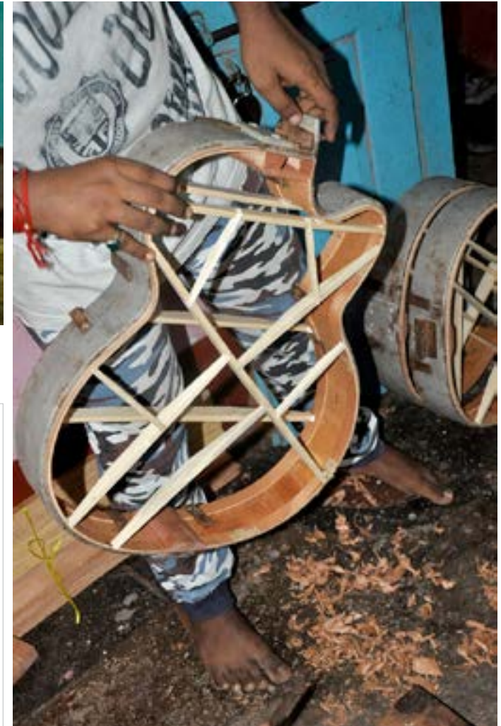
Artisan removing the mold frame.
