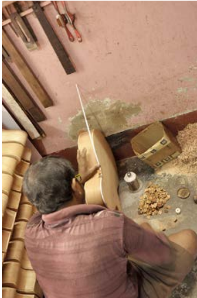
Decolam sheet strips are attached to the border.
