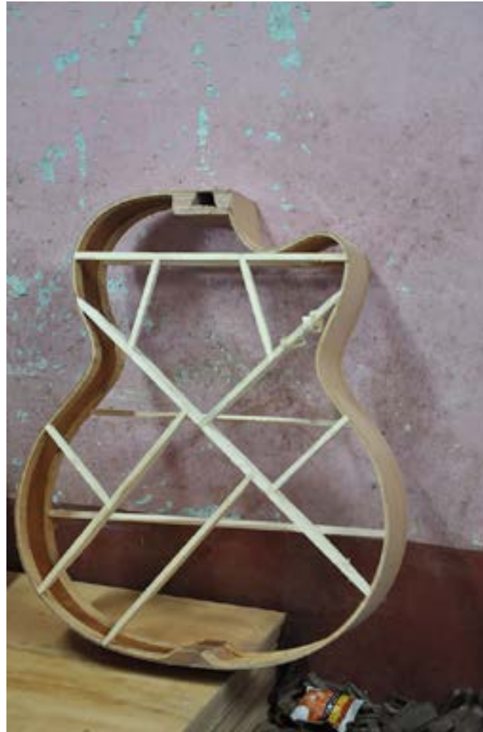
Supporting sticks being placed inside the body.
