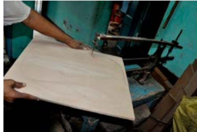
Artisan cutting the base body for the guitar.
