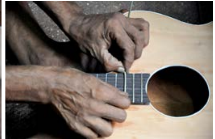
The fretboard is attached over the guitar neck and frets arranged according to the measurement.
