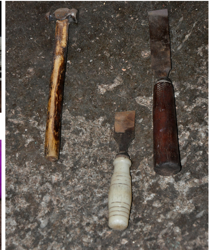
Chisels and hammer are used for the carving process.
