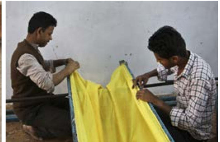
Ends of the fabric are tied to the metal frame.
