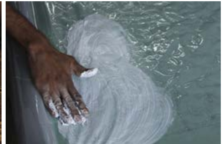
The paste is applied on the design sheet that is pinned to the fabric to trace the design.
