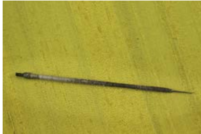
Needle (ari) shaped like a hook in the end used to embroider.
