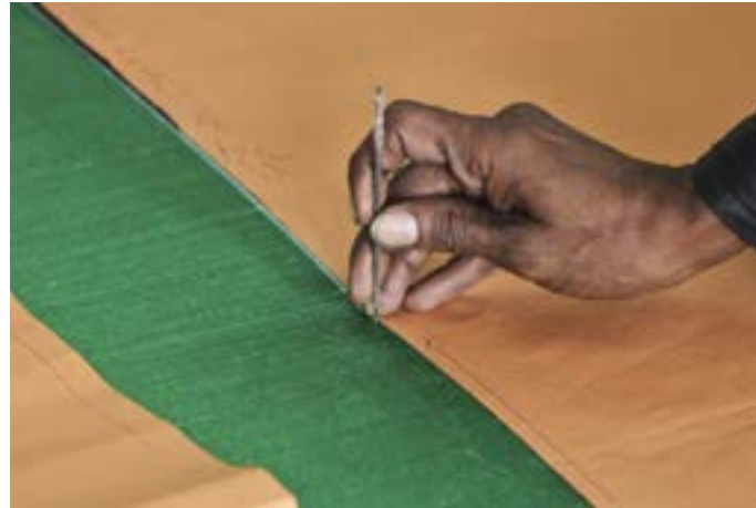
Thread is stitched along the sides of the stencil to mark the measurement.
