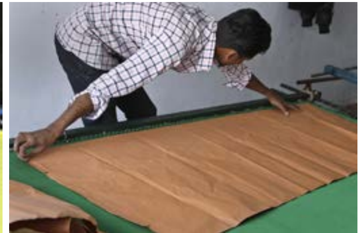
Stencil is spread along the fabric for measurement.
