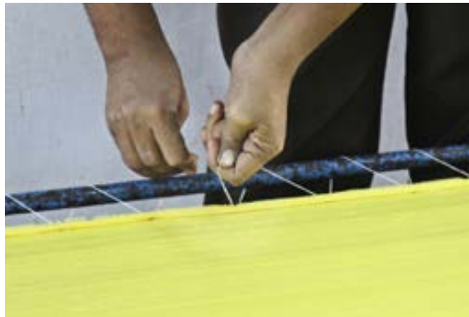
Fabric is spread on all sides and tied firmly to the frame.
