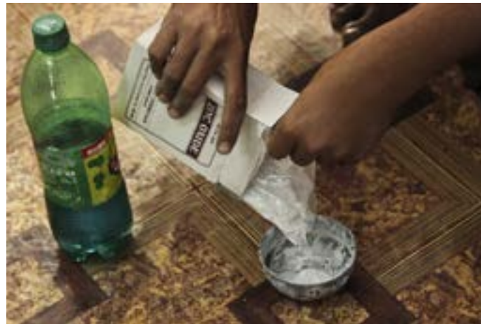
Thin paste of zinc powder and kerosene is made for tracing.
