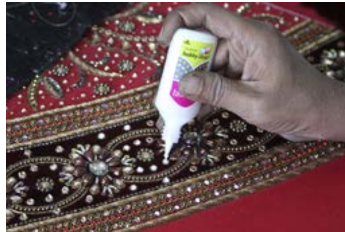
Stones are glued on the fabric using fabric adhesive.
