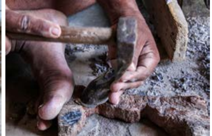
Reducing the thickness of the horn to fit it into the motor for rotation.
