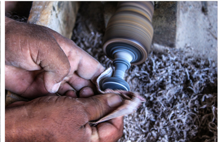
Buffing the artifact using a sand paper.
