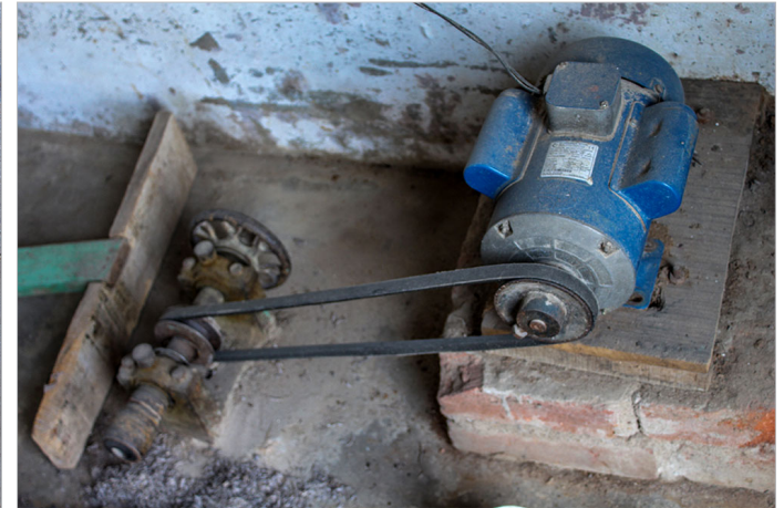
Motor used to rotate artifact at high speeds.
