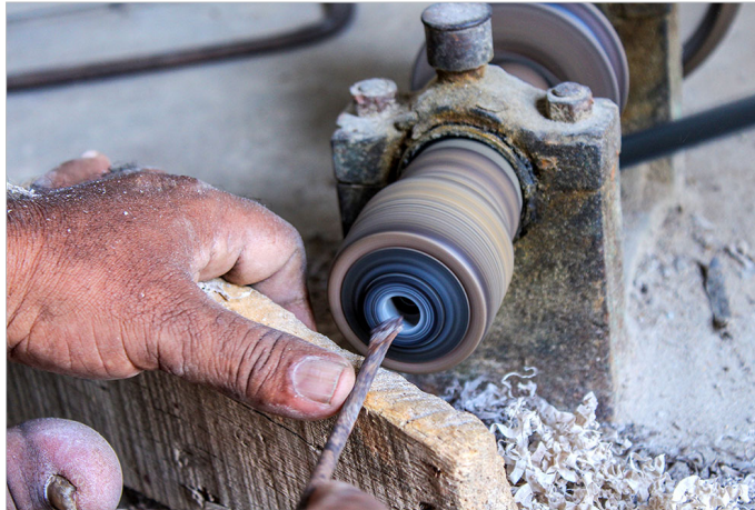
Creating a hole in the horn.
