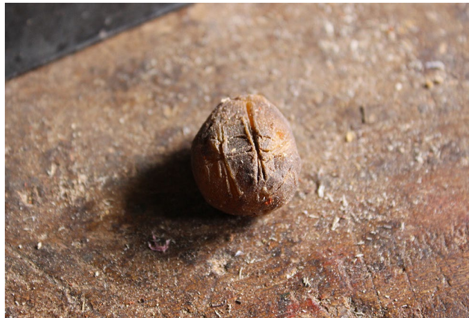
Wax applied to the blade of the coping saw for achieving friction while trimming the wood pieces.
