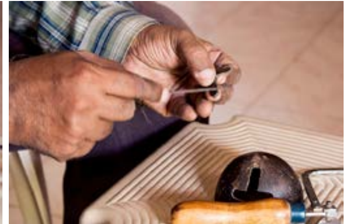
Triangular pile gives the proper and smooth design on shell.
