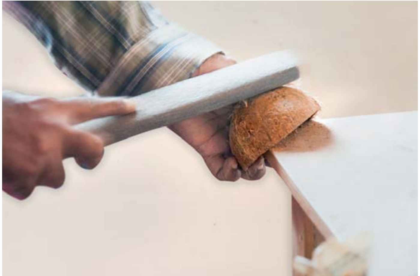
Artisan use a silicon carbide paper to get a smooth finishing.
