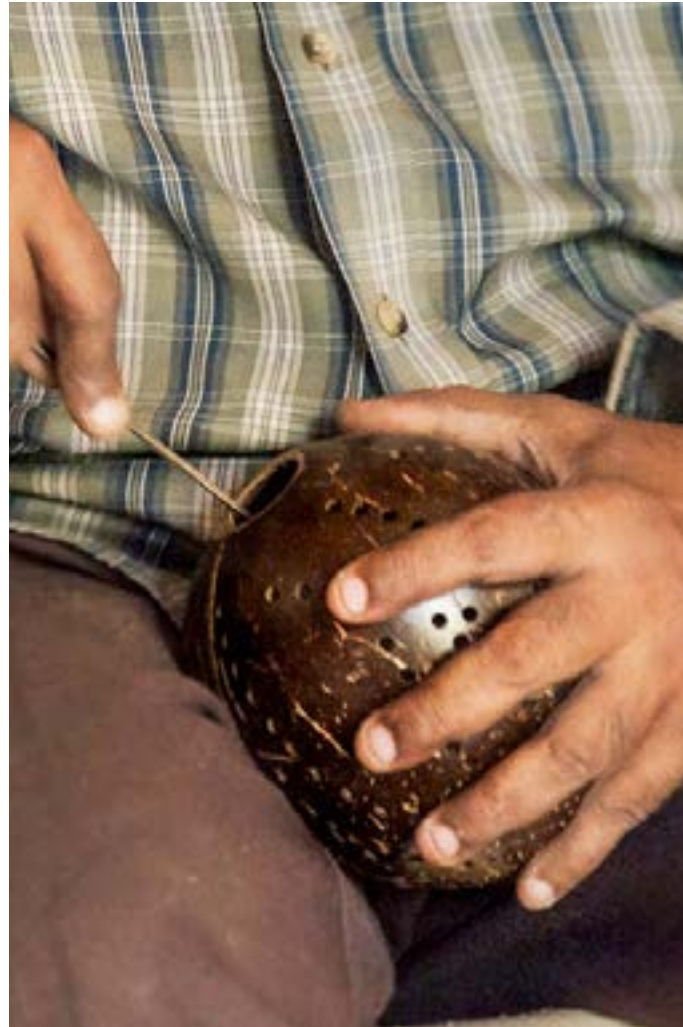
Using triangular pile artisan makes large hole for coconut shell lamp.
