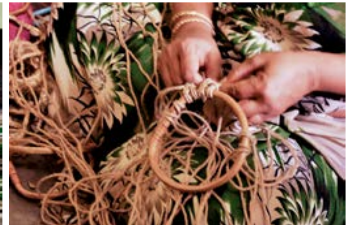
Eight jute threads being knitted on the bamboo handles to start the jute bag making process.
