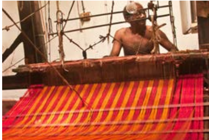
The warp threads are attached to the take-up beam.
