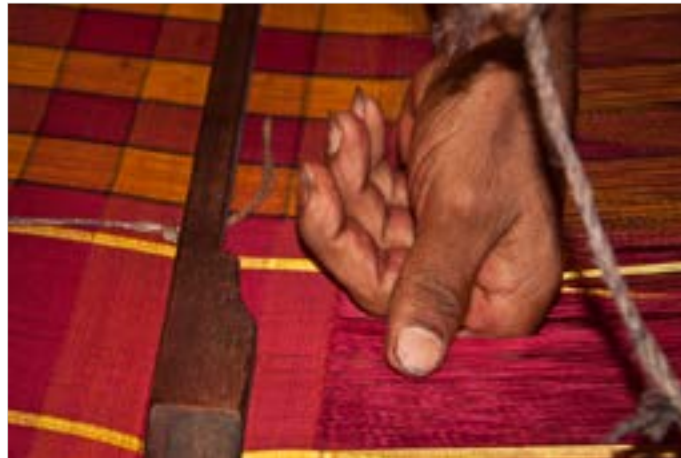
Artisan checking the stiffness of starched threads.
