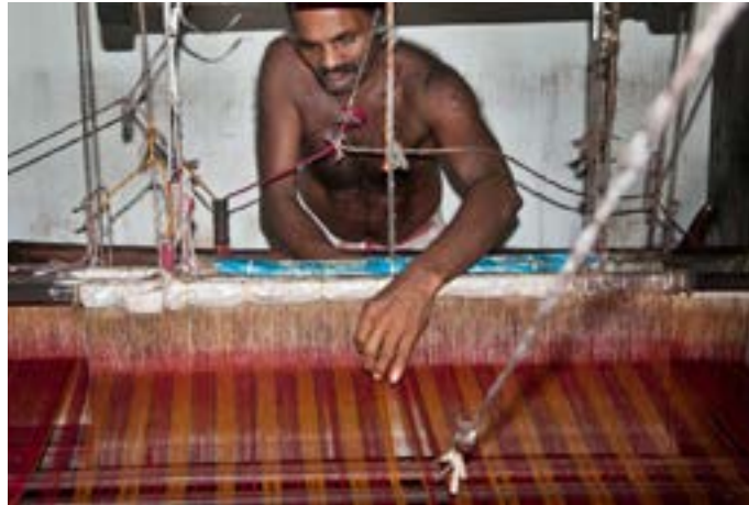
Weaver is Verifying and mending the broken threads.
