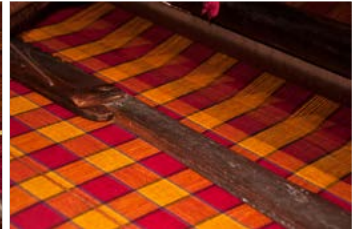
The wooden stick ( yardstick ) is fixed to the woven part of the sari for tightness and to maintain the uniform width.
