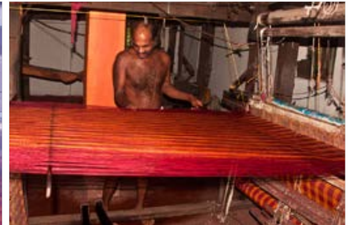
Final adjustment of warp before weaving.
