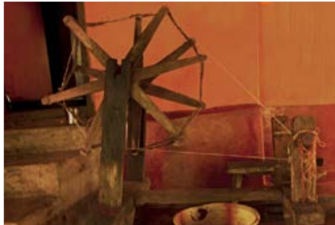
Charka ( Spinning wheel ) is used to spin the bobbins into spindles.
