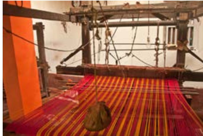
Coloured cotton warp loaded in the loom.
