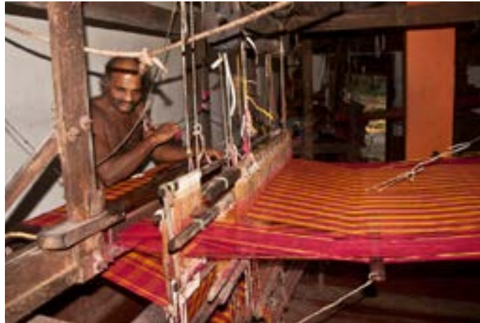
The woven sari is rolled to the take-up beam, which is near the pedal.
