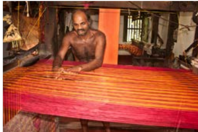
The warp of Yakshagaana sari is being inspected by weaver.
