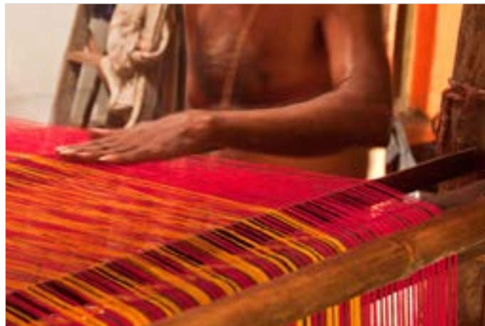
Wooden sticks (Lease ) are inserted in the warp of threads for tightness and to keep the 2 sets of thread separate.
