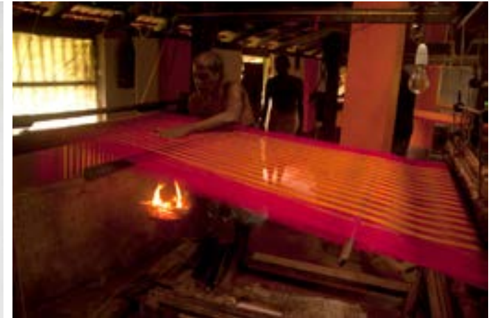
Fire is used to dry the cotton threads after starching.
