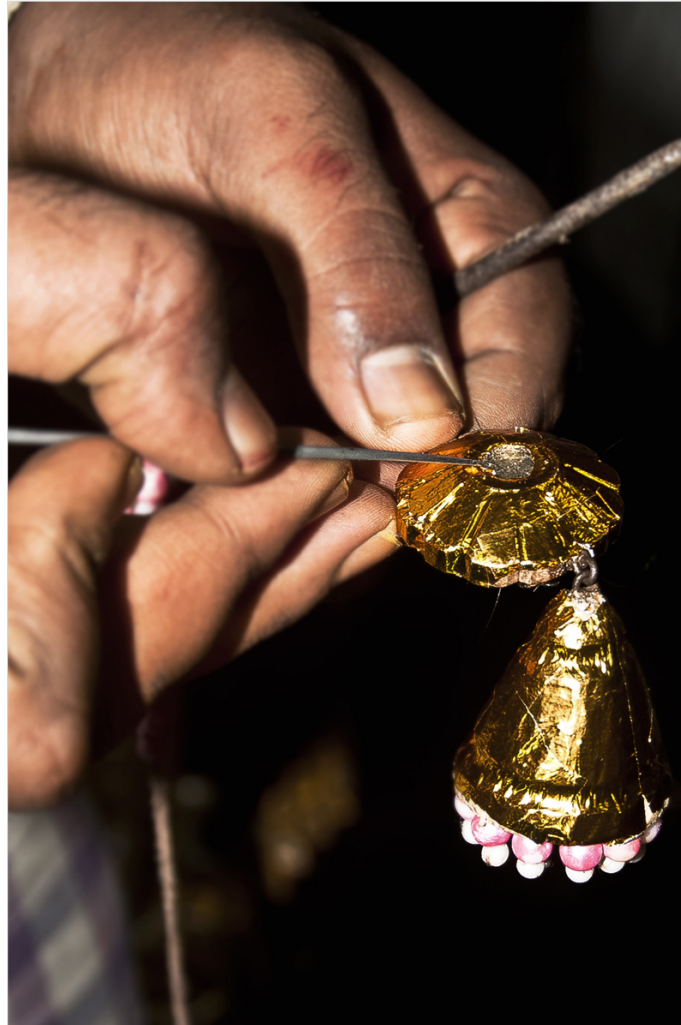
Sharp tools are used to fix the foil on the jewellery surface.
