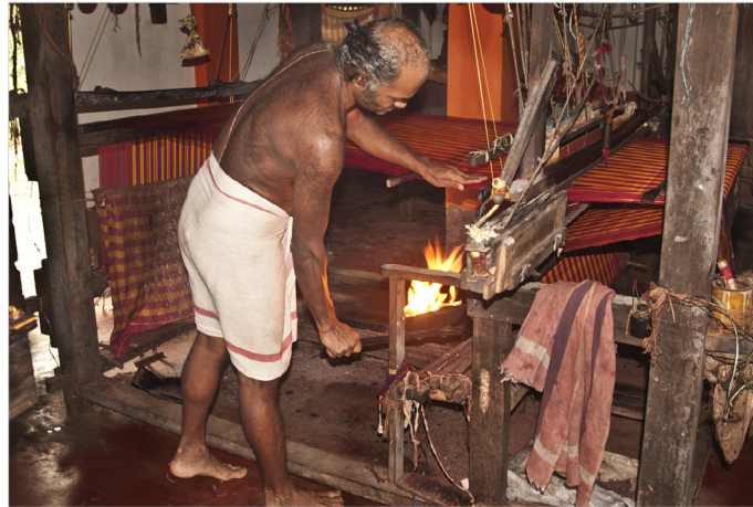
The warp is heated to dry the starch.
