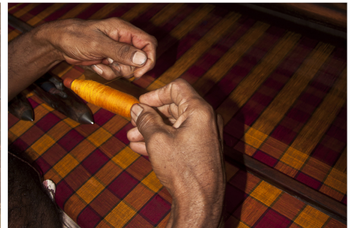
Weaver is inserting the Spindle in the fly shuttle.
