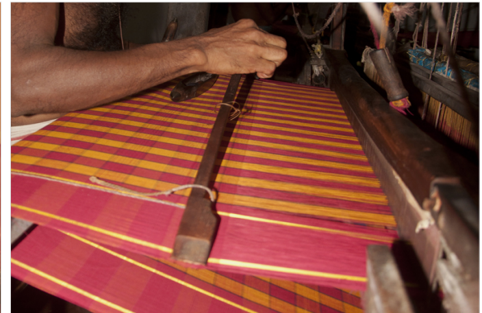
The weaver is putting a wooden tool (like a yardstick) to keep the width of the woven sari uniform.
