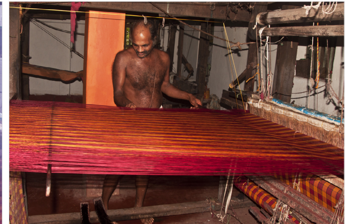
Final adjustment of warp before weaving.
