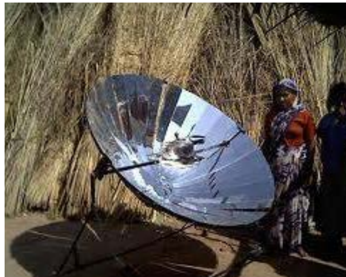
Parabolic type solar cooker
